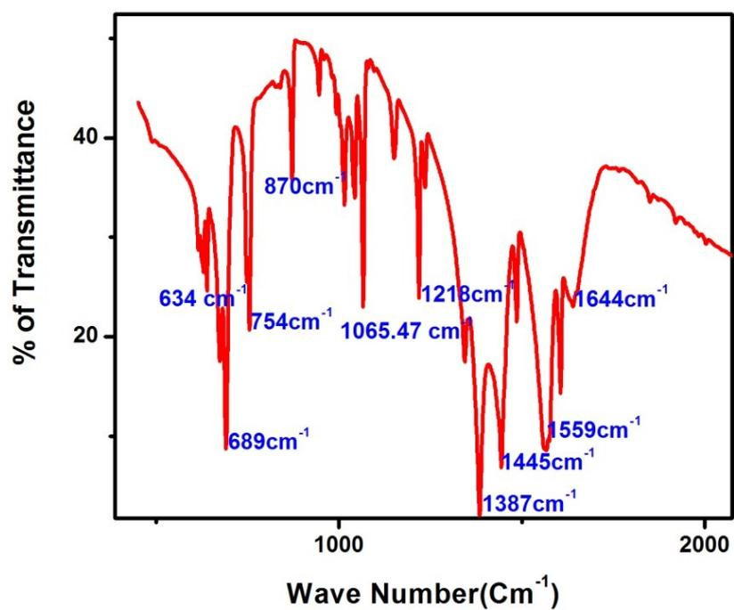
Fig. SI 4: FTIR spectrum of complex 1.
