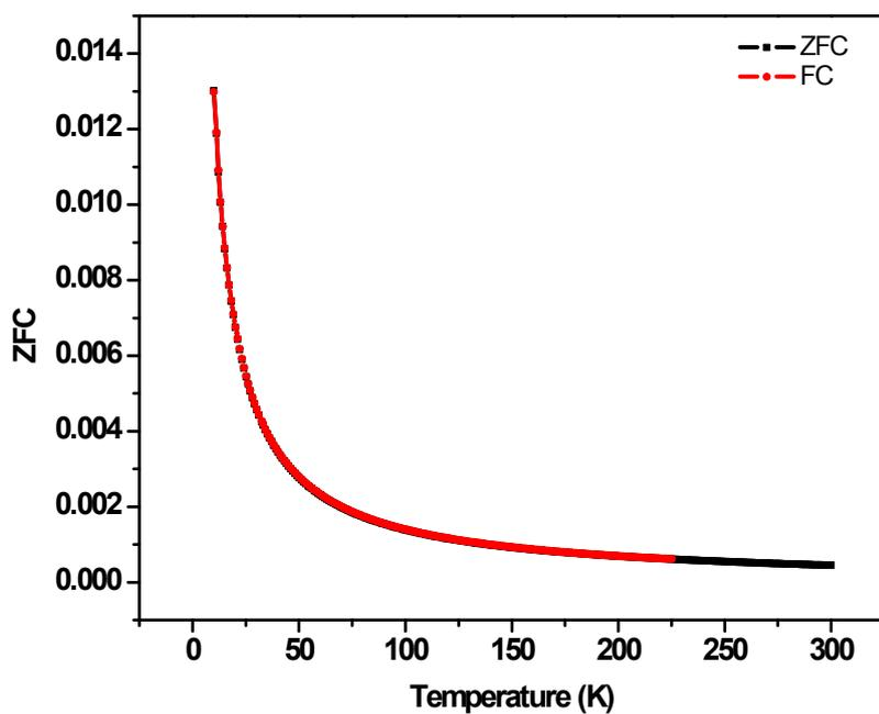
Fig. SI 3. Temperature dependent magnetization plots of complex 1 at 100 Oe.
