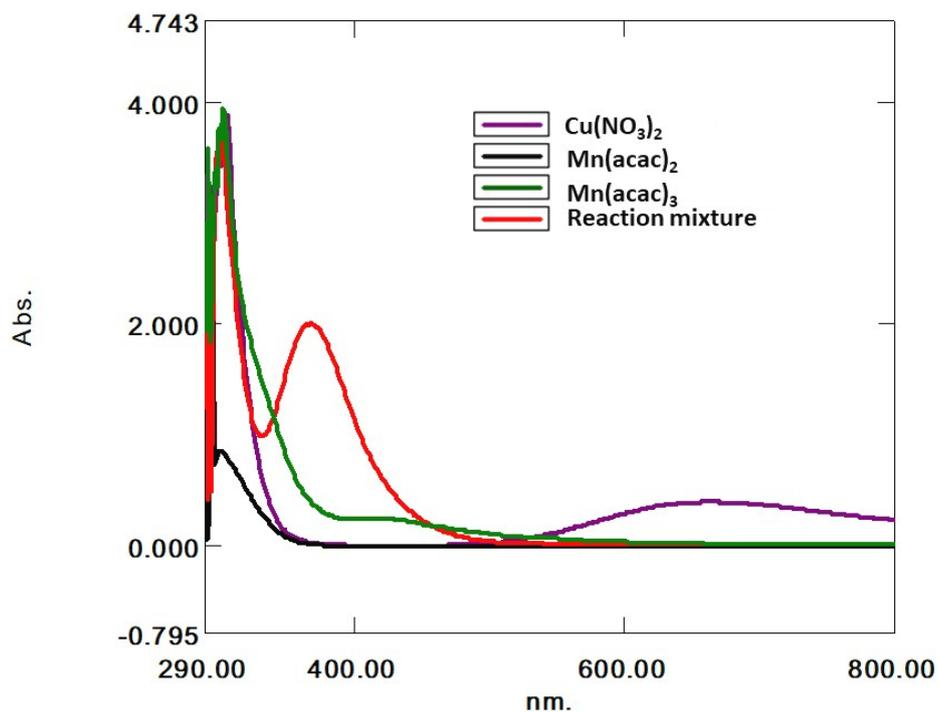
**Fig. SI 1 (A):** UV-vis spectra of (i) Cu(NO<sub>3</sub>)<sub>2</sub>, (ii) Mn(acac)<sub>2</sub>, (iii) Mn(acac)<sub>3</sub> and (iv) Reaction mixture of complexation
