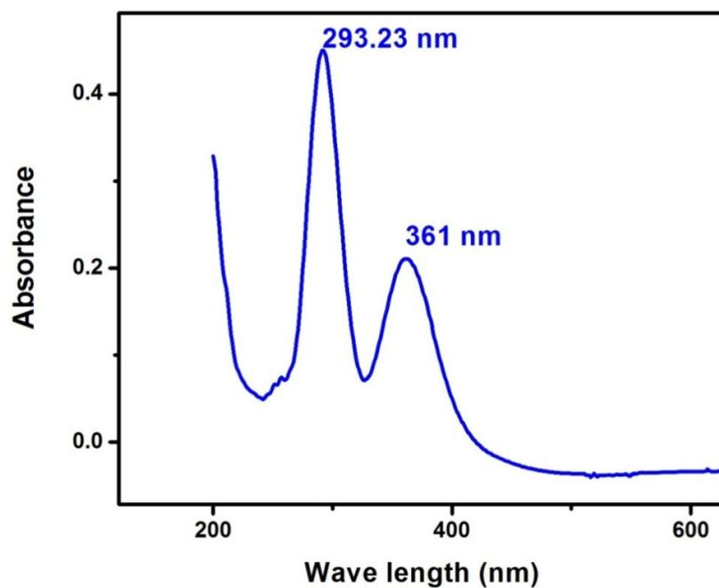
**Fig. SI 1(B):** UV-vis spectrum of complex 1 in methanol.
