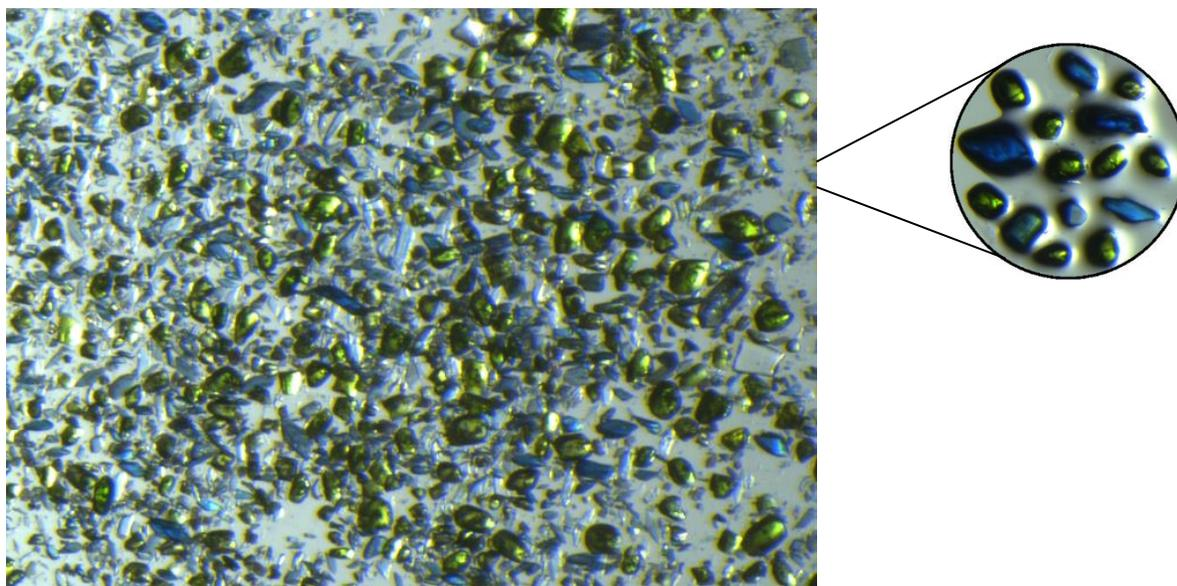
Figure S1: Concomitant crystals of copper(II) isonicotinate-*N*-oxide- form I (blue) and form II (green)
