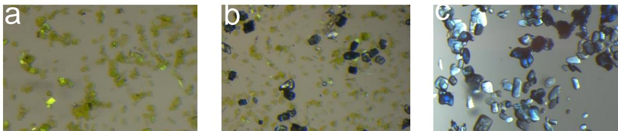
Figure S2: Crystallisation of (a) form-II (green) in (<math><3.5\%</math> water), (b) concomitant crystals (5-10% water) and (c) form-I (blue) (>10% water) in ethanol-water.
