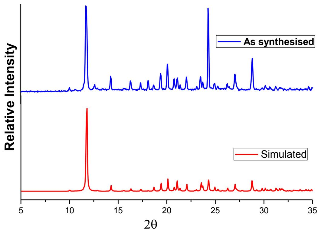
Figure S6: XRPD comparison of simulated and bulk solid of form-IV
