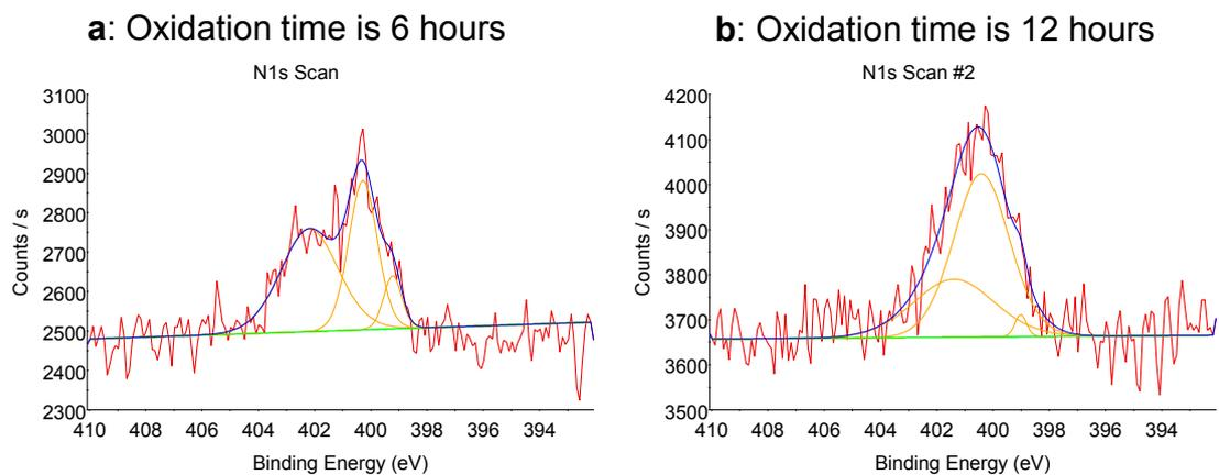
Figure 3s The N1s high resolution XPS analysis of the NG on SiCm prepared by the reactions between hydrazine and the MG on SiC oxidized in concentrated HNO<sub>3</sub> for 6 (a) and 12 (b) hours, respectively.
