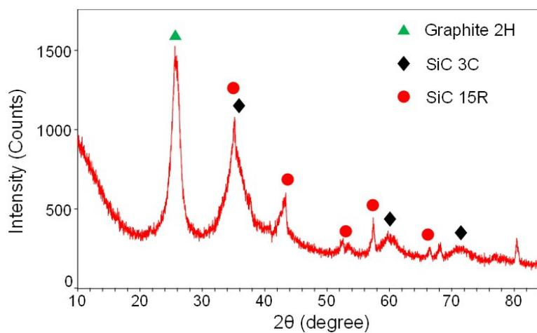
Figure 5s The XRD pattern of the NG on SiCm prepared by the reactions between hydrazine and the MG on SiC oxidized in concentrated HNO<sub>3</sub> for 96 hours
