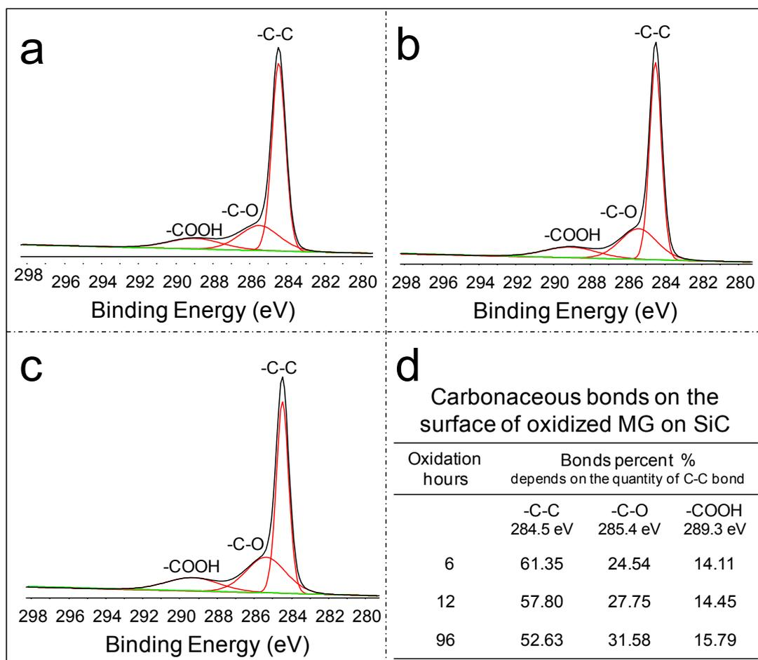
Figure 2s The high resolution C1s XPS analysis of the oxidized MG on SiC after treated in concentrated HNO<sub>3</sub> for 6 (a), 12 (b), 96 (c) hours, respectively; (d) the calculated carbonaceous bonds on the surface of the MG on SiC
