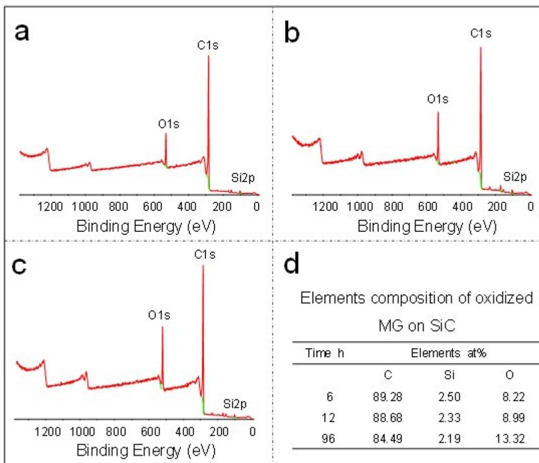
Figure 1s The XPS spectra of the MG on SiC oxidized in concentrated HNO<sub>3</sub> for 6 (a), 12 (b), 96 (c) hours, respectively; the elements composition on the surface (d) of oxidized MG on SiC
