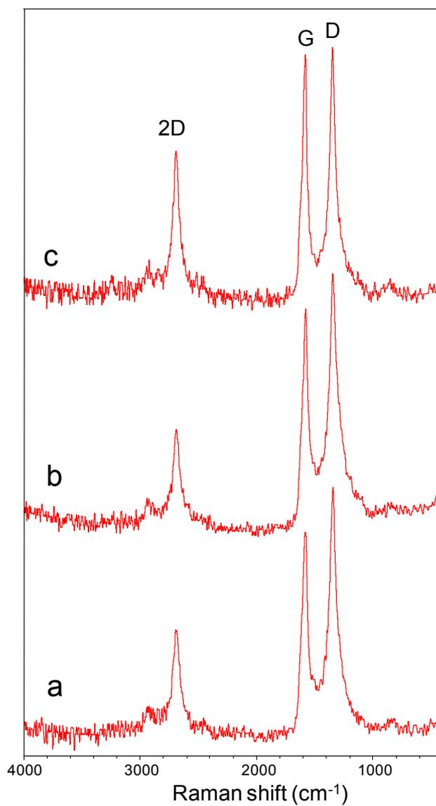
Figure 4s The Raman spectra of NG on SiCm which prepared by the reduction reactions with hydrazine and oxidized MG on SiC that treated in concentrated  $\text{HNO}_3$  for 6 (a), 12 (b) and 96 (c) hours.
