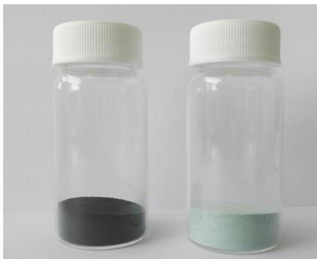
Fig. S4. Image of the samples of MIL-101/MoS<sub>2</sub> (left) and MIL-101 (right).
