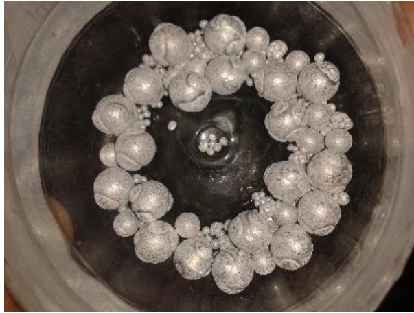
Fig. S1 Cold welding photograph of aluminum powders ball milled for 14 h without using \text{NH}_4\text{Cl} .
