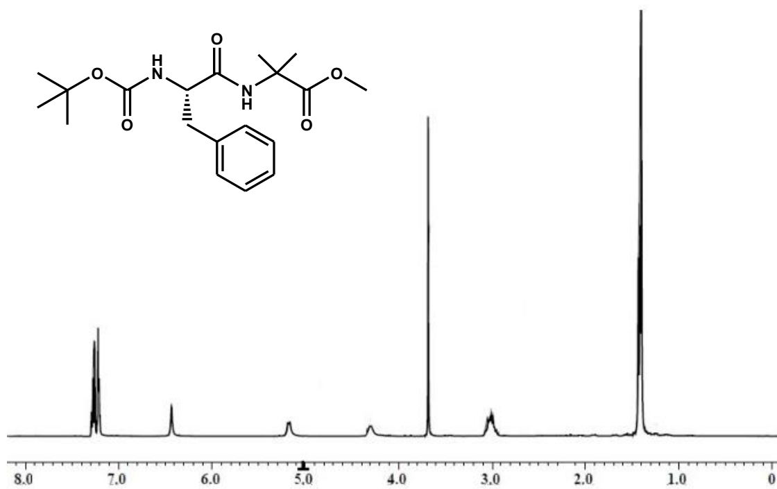
Figure S1: 1 H NMR (500 MHz, CDCl 3 ) spectrum of Boc-Phe-Aib-OMe.
