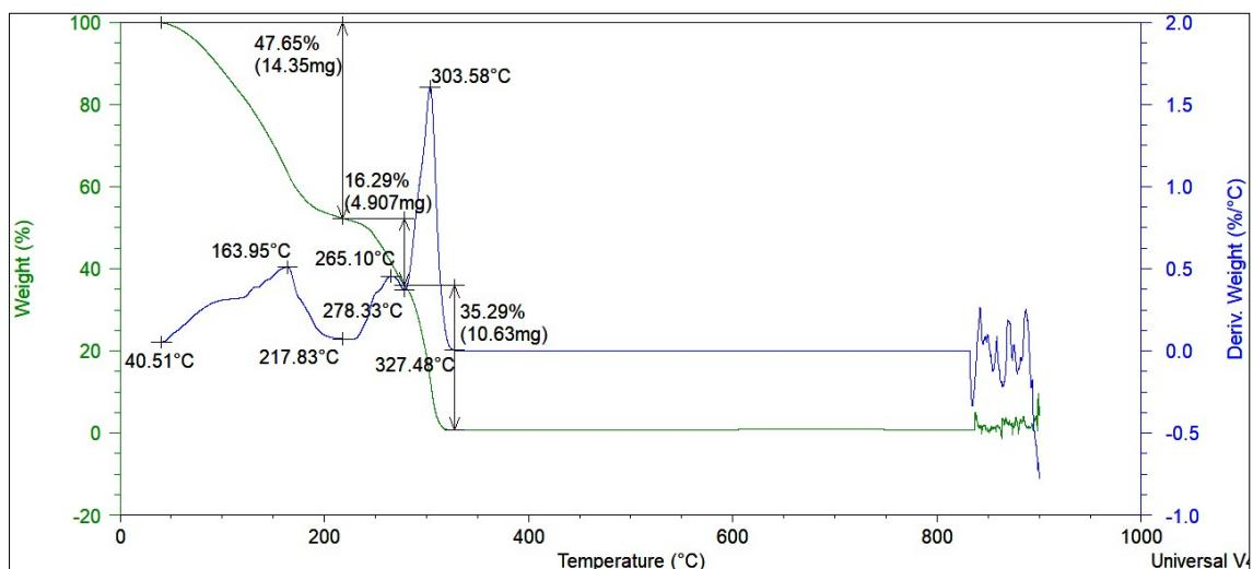
**Figure S8.** TGA of ChCl:Ethyleneglycol (1:1).
