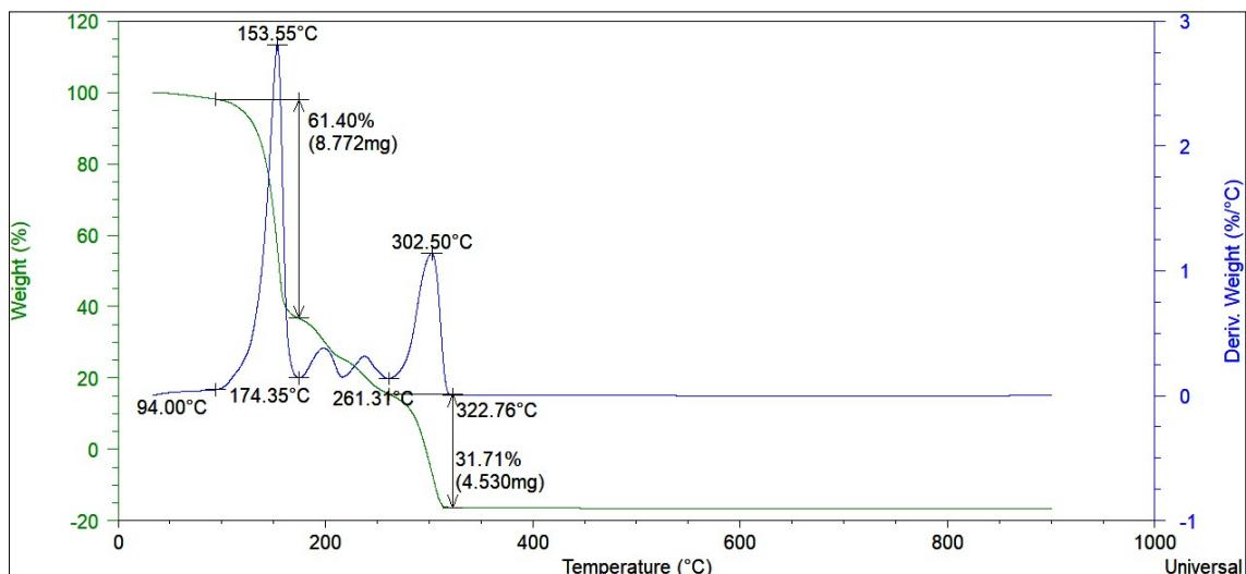
**Figure S12.** TGA of ChCl:maloni acid (1:2).
