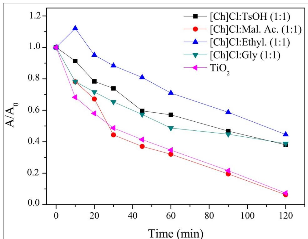
**Figure S53.** Graph of MO photodecomposition promoted by DES+TiO<sub>2</sub> coated. ChCl:TsOH 1:1+TiO<sub>2</sub> coated (**black**); ChCl:malonic acid 1:1+TiO<sub>2</sub> coated (**red**); ChCl:ethyleneglycol 1:1+TiO<sub>2</sub> coated (**blue**); ChCl:glycerol 1:1+TiO<sub>2</sub> coated (**green**); TiO<sub>2</sub> pure (**pink**).
