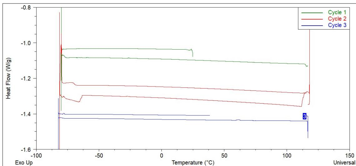
**Figure S33.** DSC curve of ChCl:Malonic Acid (1:1).
