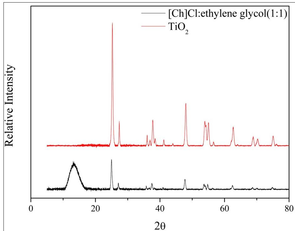
**Figure S46.** XRD data of pure  $\text{TiO}_2$  (red) and [Ch]Cl:ethylene glycol (1:1)+ $\text{TiO}_2$  (black).
