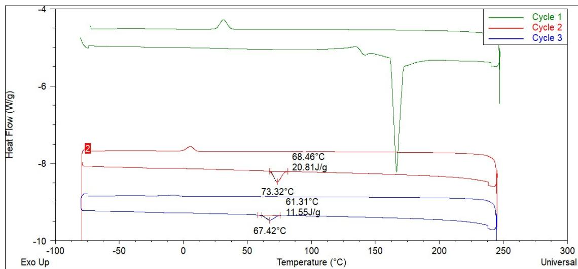
**Figure S43.** DSC curve of ChCl:malonic acid (1:2)+TiO<sub>2</sub> coated.
