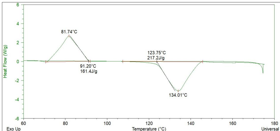
**Figure S24.** DSC curve of Urea. Cycle 1.
