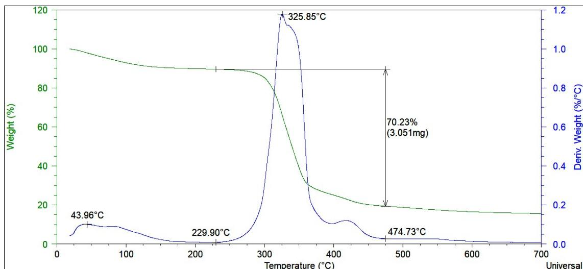
**Figure S23.** TGA of ChCl:TsOH 1:2+TiO<sub>2</sub> coated.
