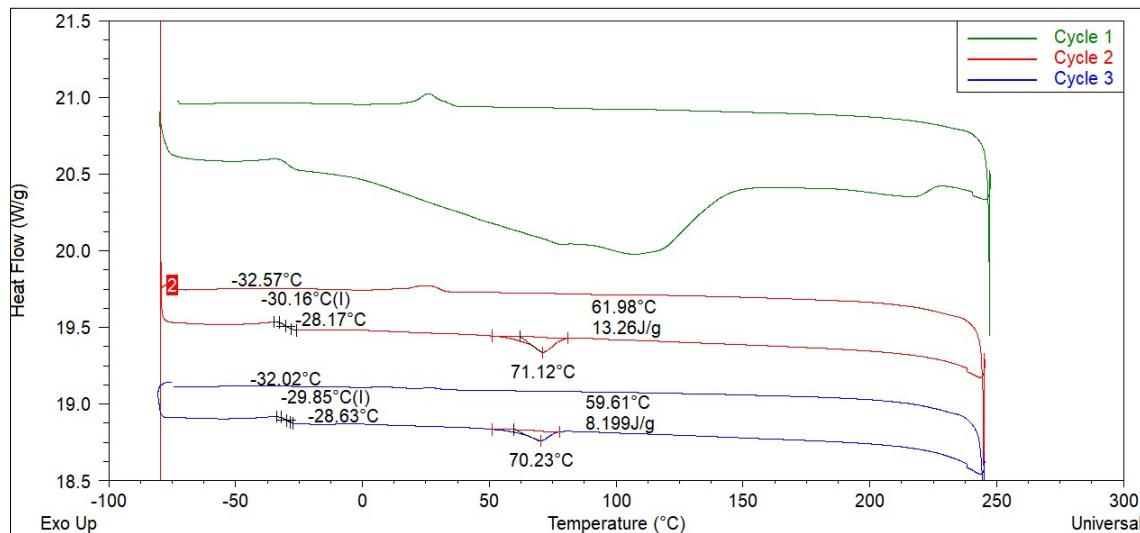
**Figure S39.** DSC curve of ChCl:ethyleneglycol (1:2)+TiO<sub>2</sub> coated.
