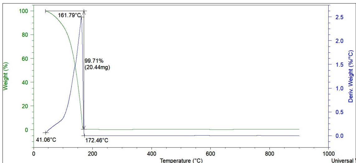
**Figure S3.** TGA of ethyleneglycol.
