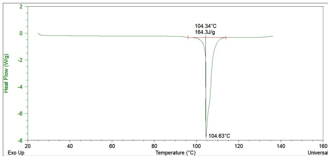
**Figure S27.** DSC curve of TsOH. Cycle 1
