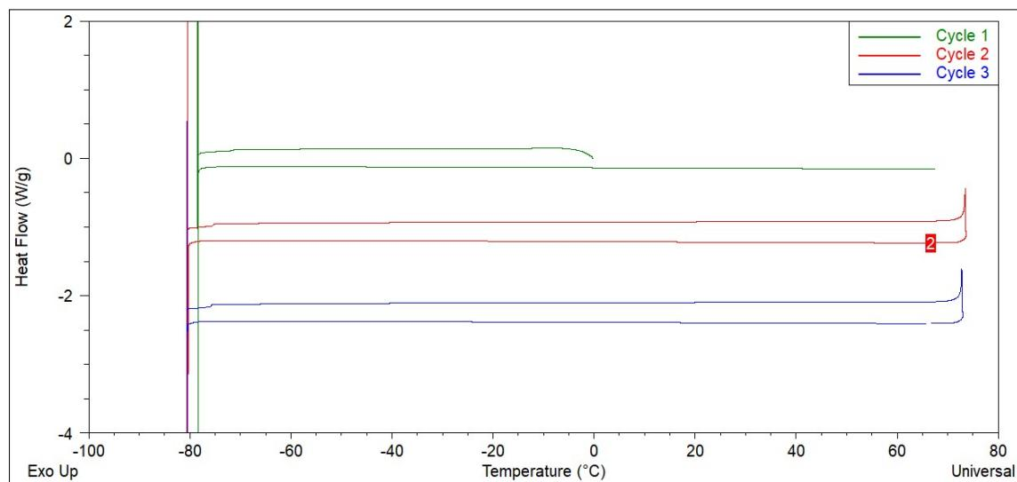
**Figure S30.** DSC curve of ChCl:Ethyleneglycol (1:2).
