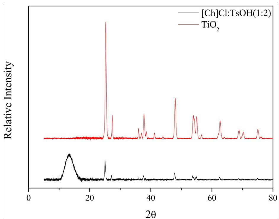
**Figure S52.** XRD data of pure TiO<sub>2</sub> (**red**) and [Ch]Cl:Toluene Sulfonic Acid (1:2)+TiO<sub>2</sub> (**black**).
