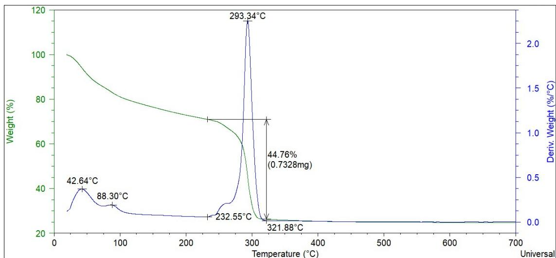
**Figure S16.** TGA of ChCl:ethyleneglycol 1:1+TiO<sub>2</sub> coated.
