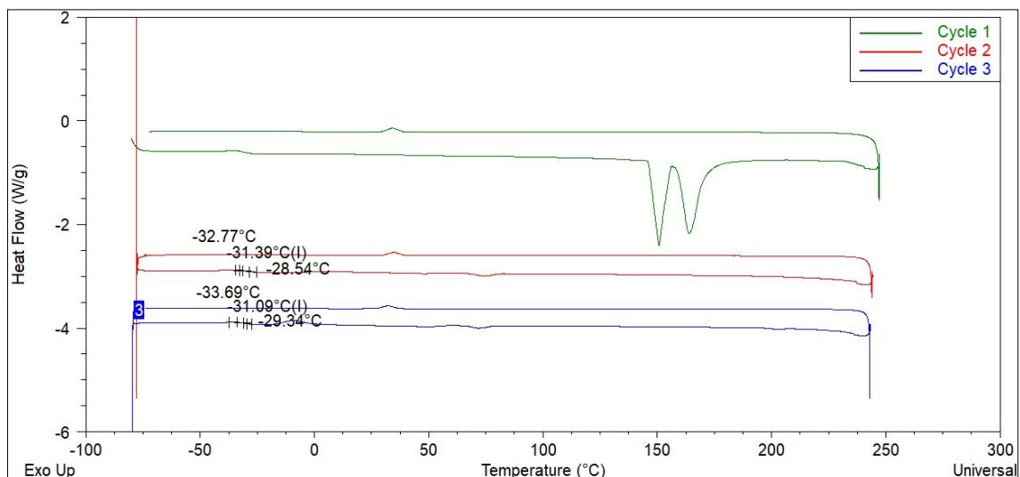
**Figure S40.** DSC curve of ChCl:glycerol (1:1)+TiO<sub>2</sub> coated.
