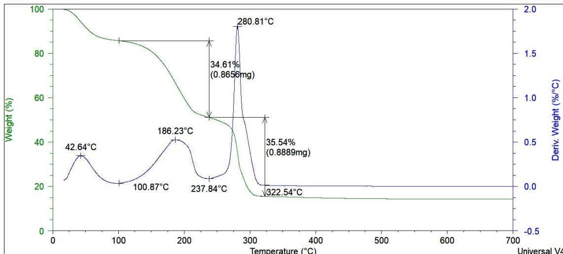
**Figure S19.** TGA of ChCl:glycerol 1:2+TiO<sub>2</sub> coated.
