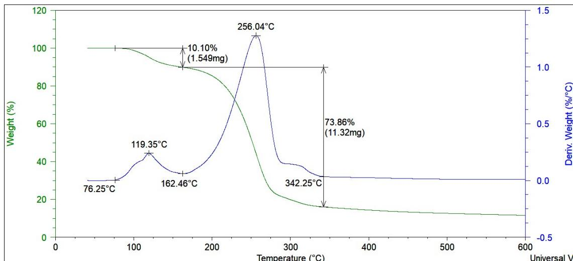
**Figure S3.** TGA of toluene sulphonic acid.
