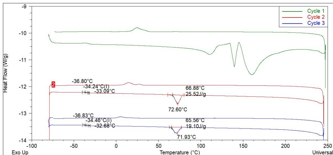
**Figure S42.** DSC curve of ChCl:malonic acid (1:1)+TiO<sub>2</sub> coated.
