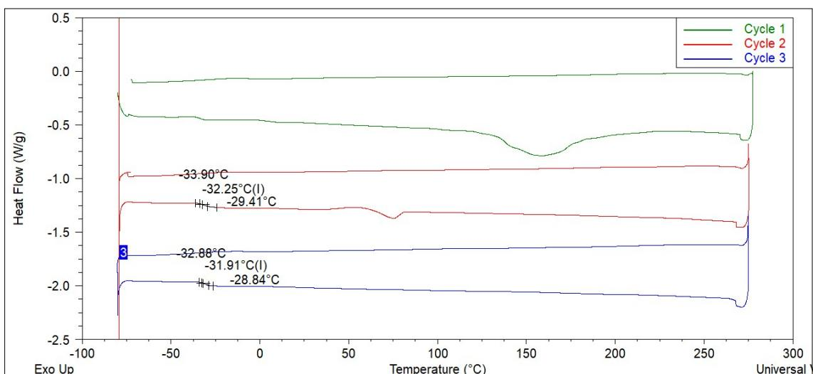
**Figure S45.** DSC curve of ChCl:TsOH (1:2)+TiO<sub>2</sub> coated.
