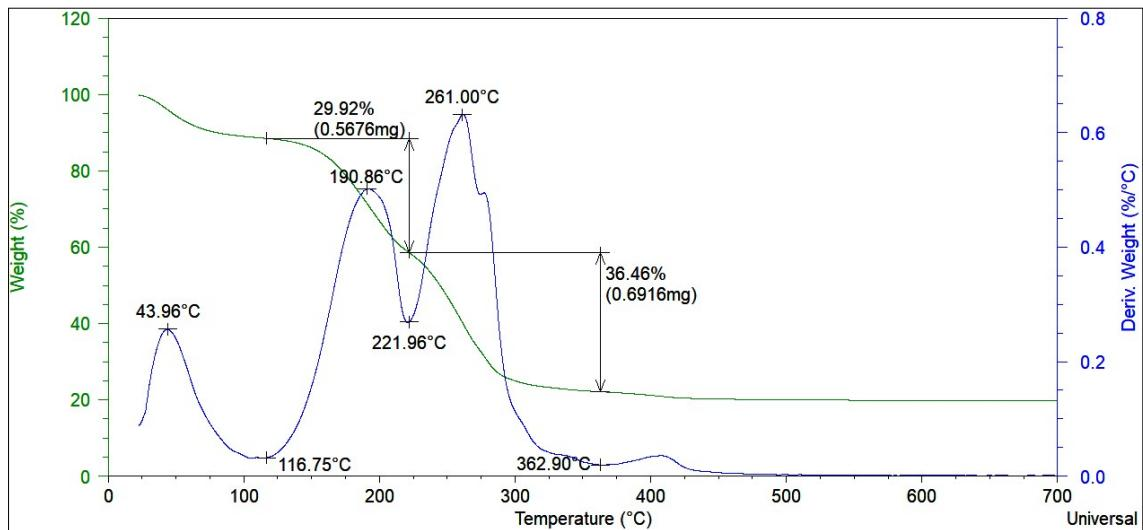
**Figure S15.** TGA of ChCl:urea 1:2+TiO<sub>2</sub> coated.
