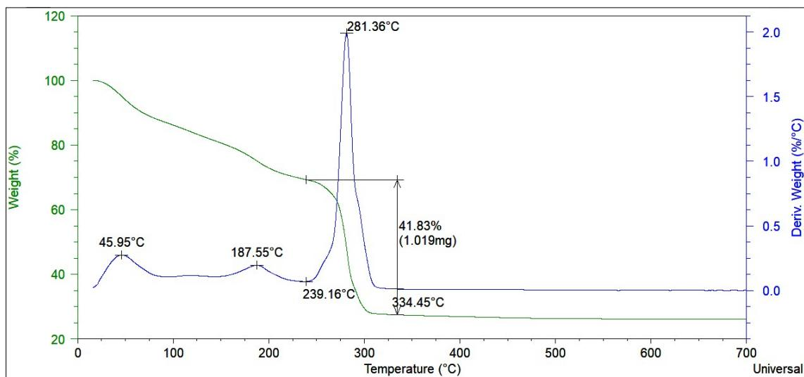
**Figure S18.** TGA of ChCl:glycerol 1:1+TiO<sub>2</sub> coated.
