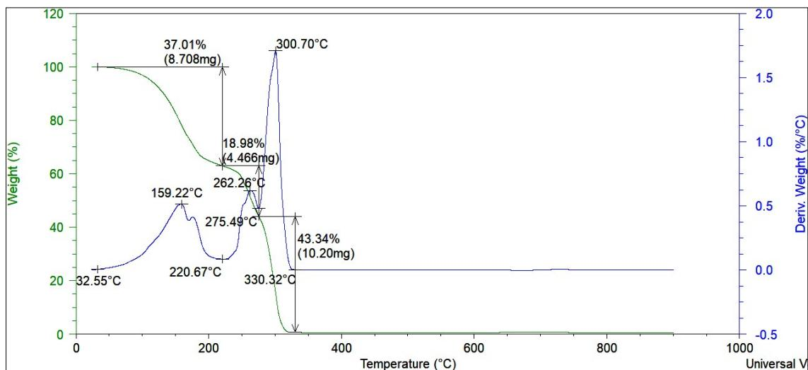
**Figure S9.** TGA of ChCl:Ethyleneglycol (1:2).
