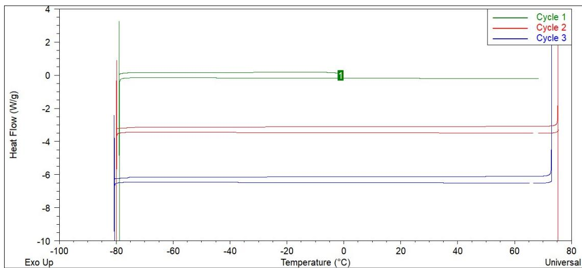
**Figure S29.** DSC curve of ChCl:Ethylene glycol (1:1).
