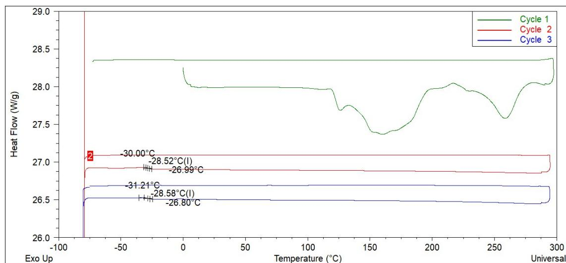
**Figure S37.** DSC curve of ChCl:urea (1:2)+TiO<sub>2</sub> coated.
