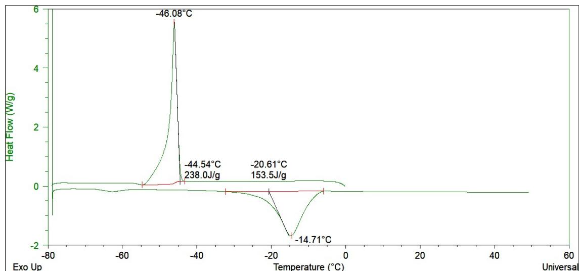
**Figure S25.** DSC curve of Ethyleneglycol. Cycle 1.
