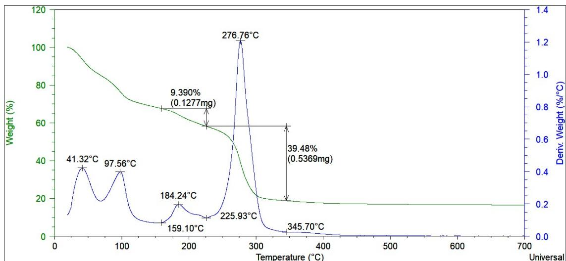
**Figure S17.** TGA of ChCl:ethyleneglycol 1:2+TiO<sub>2</sub> coated.
