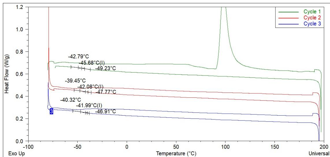
**Figure S36.** DSC curve of ChCl:TsOH (1:2).
