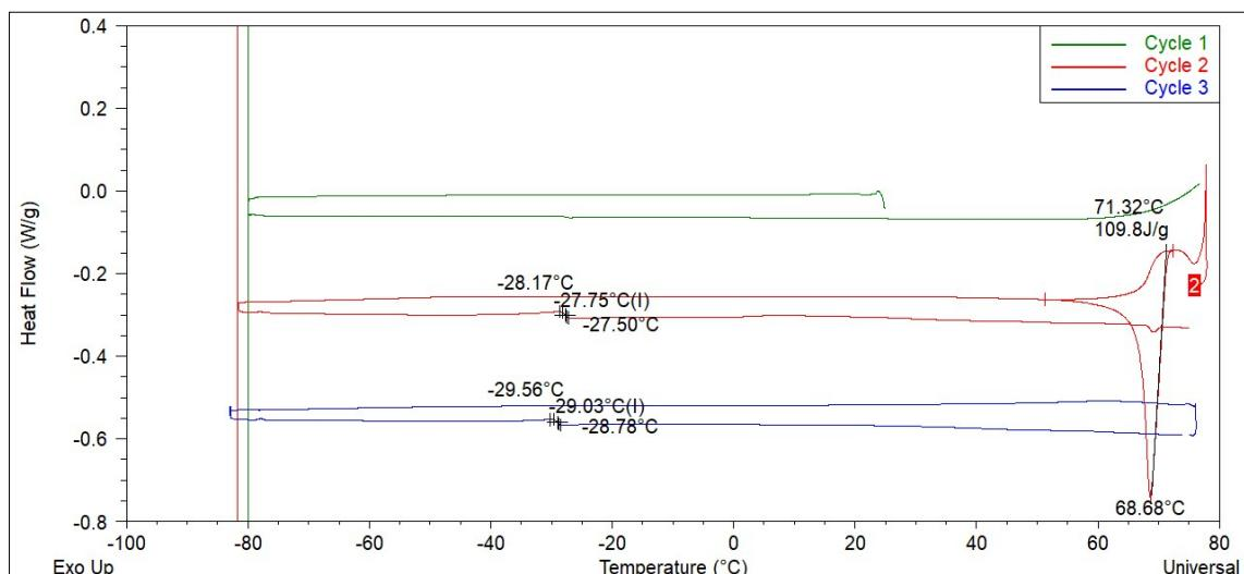
**Figure S35.** DSC curve of ChCl:TsOH (1:1).
