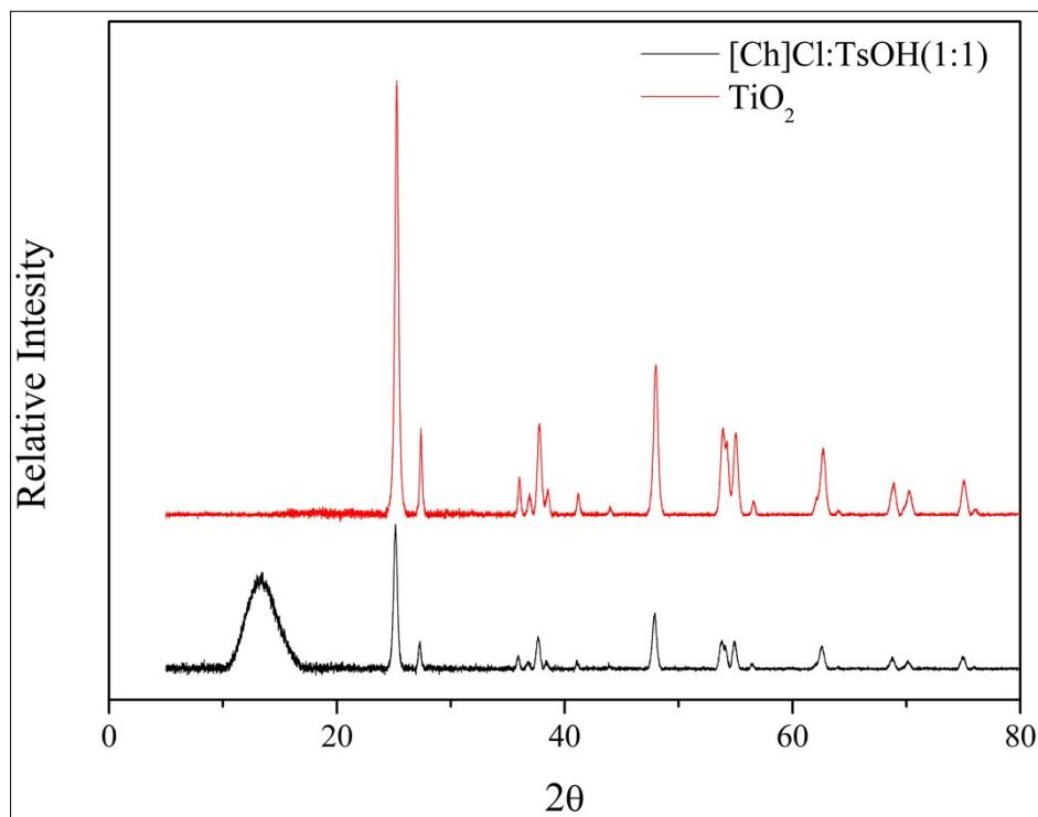
**Figure S51.** XRD data of pure  $\text{TiO}_2$  (red) and  $\text{[Ch]Cl:Toluene Sulfonic Acid (1:1)+TiO}_2$  (black).
