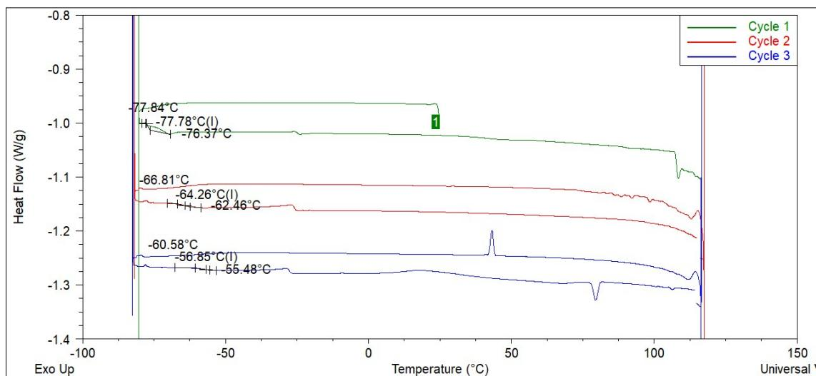
**Figure S34.** DSC curve of ChCl:Malonic Acid (1:2).
