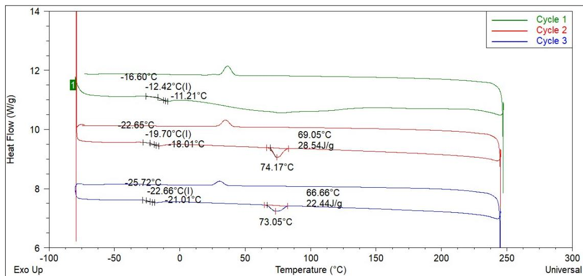
**Figure S38.** DSC curve of ChCl:ethyleneglycol (1:1)+TiO<sub>2</sub> coated.
