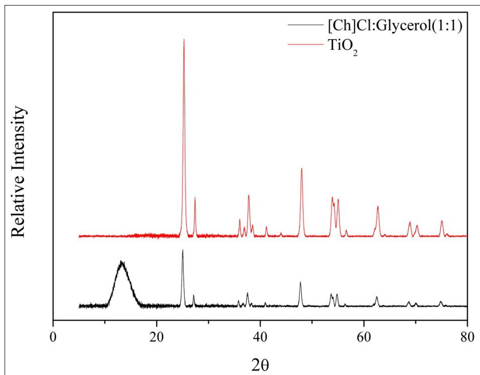
**Figure S48.** XRD data of pure  $\text{TiO}_2$  (**red**) and [Ch]Cl:glycerol (1:1)+ $\text{TiO}_2$  (**black**).
