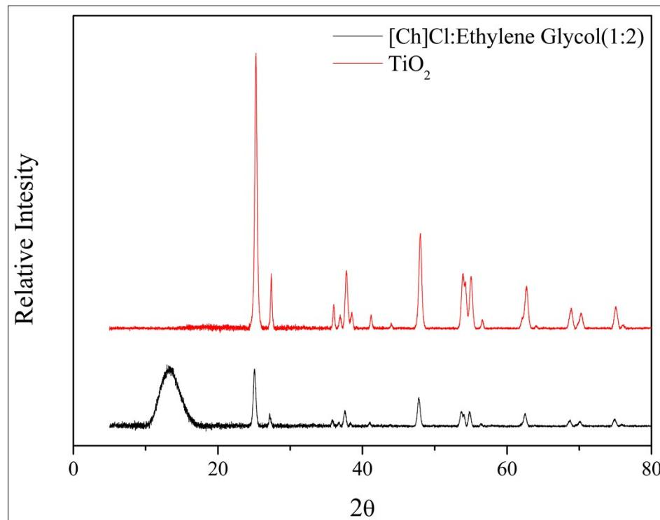
**Figure S47.** XRD data of pure  $\text{TiO}_2$  (red) and [Ch]Cl:ethylene glycol (1:2)+ $\text{TiO}_2$  (black).
