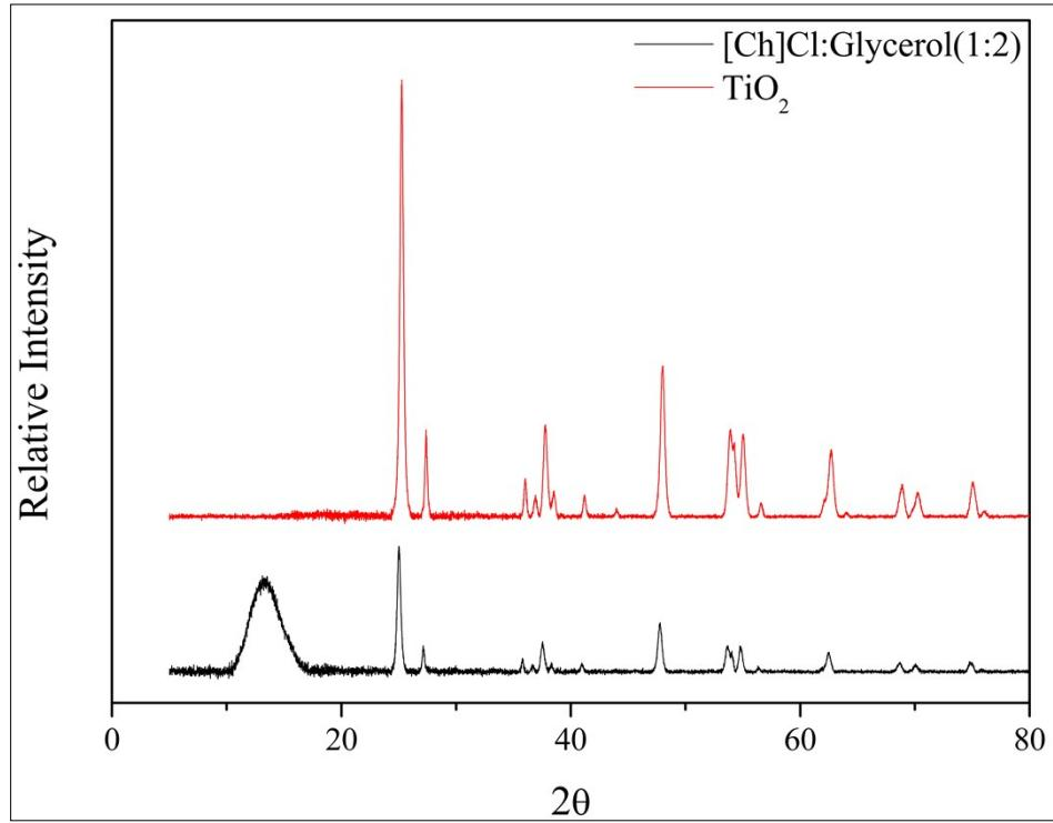
**Figure S49.** XRD data of pure  $\text{TiO}_2$  (**red**) and [Ch]Cl:glycerol (1:2)+ $\text{TiO}_2$  (**black**).
