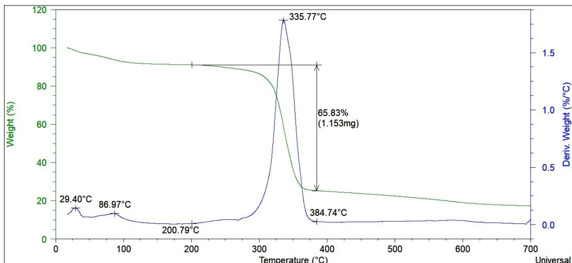
**Figure S22.** TGA of ChCl:TsOH 1:1+TiO<sub>2</sub> coated.
