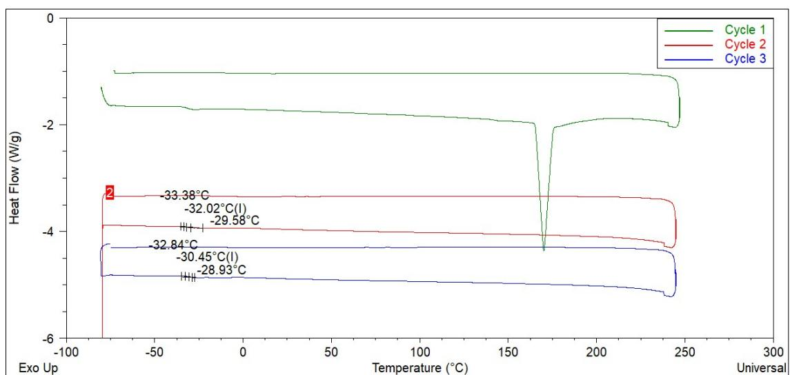
**Figure S41.** DSC curve of ChCl:glycerol (1:2)+TiO<sub>2</sub> coated.
