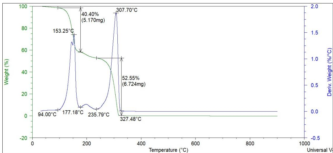
**Figure S11.** TGA of ChCl:malonic acid (1:1).
