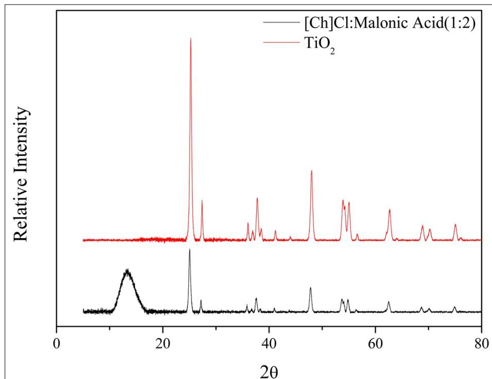
**Figure S50.** XRD data of pure  $\text{TiO}_2$  (red) and  $\text{[Ch]Cl:Malonic Acid (1:2)+TiO}_2$  (black).
