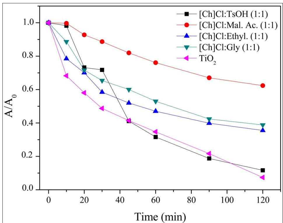
**Figure S54.** Graph of MO photodecomposition promoted by DES+TiO<sub>2</sub>. ChCl:TsOH 1:1+TiO<sub>2</sub> coated (**black**); ChCl:malonic acid 1:1+TiO<sub>2</sub> coated (**red**); ChCl:ethyleneglycol 1:1+TiO<sub>2</sub> coated (**blue**); ChCl:glycerol 1:1+TiO<sub>2</sub> coated (**green**); TiO<sub>2</sub> pure (**pink**).
