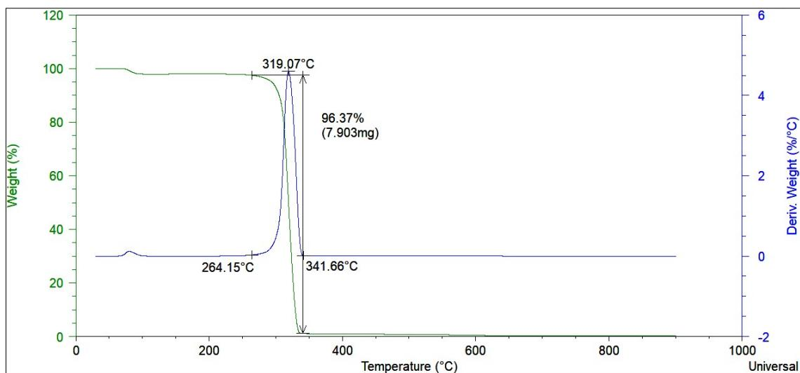
**Figure S1.** TGA of choline chloride.
