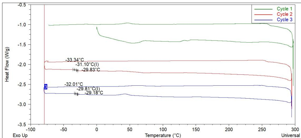
**Figure S44.** DSC curve of ChCl:TsOH (1:1)+TiO<sub>2</sub> coated.
