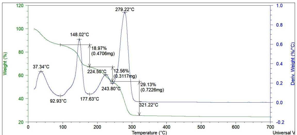
**Figure S20.** TGA of ChCl:malonic acid 1:1+TiO<sub>2</sub> coated
