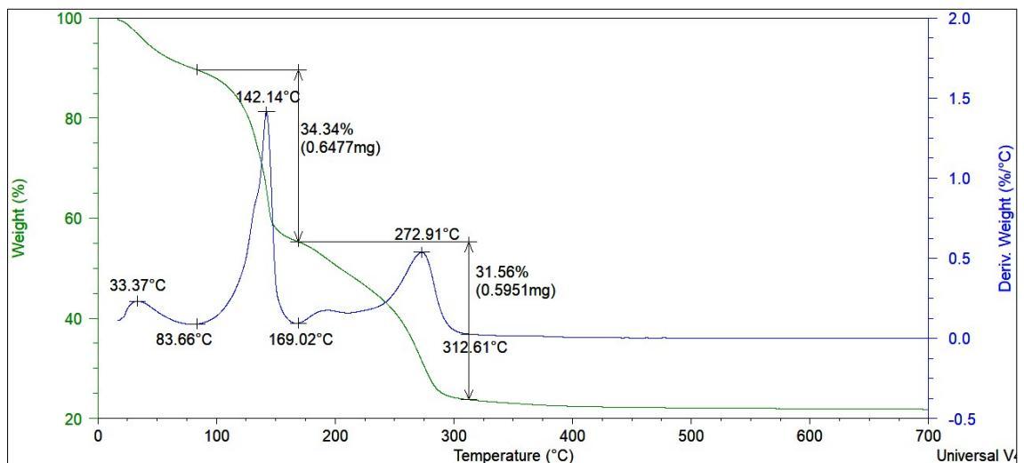
**Figure S21.** TGA of ChCl:malonic acid 1:2+TiO<sub>2</sub> coated.
