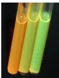
**Fig. S6** Photoimage illustrating the luminescent color changes of **1** upon different concentrations (from left to right:  $0.5 \times 10^{-2}$  M,  $1.0 \times 10^{-3}$  M,  $0.5 \times 10^{-3}$  M) under 365 nm handheld UV lamp.
