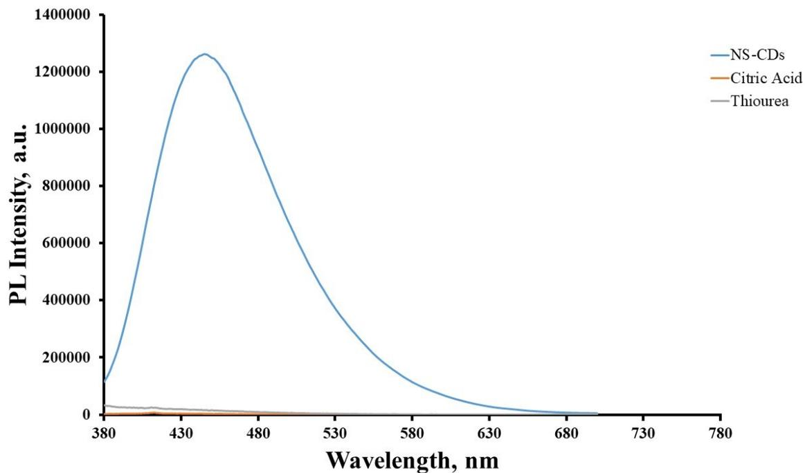
Figure S2: The PL emission of the citric acid and thiourea as compared to NS-CDs at 360nm excitation.
