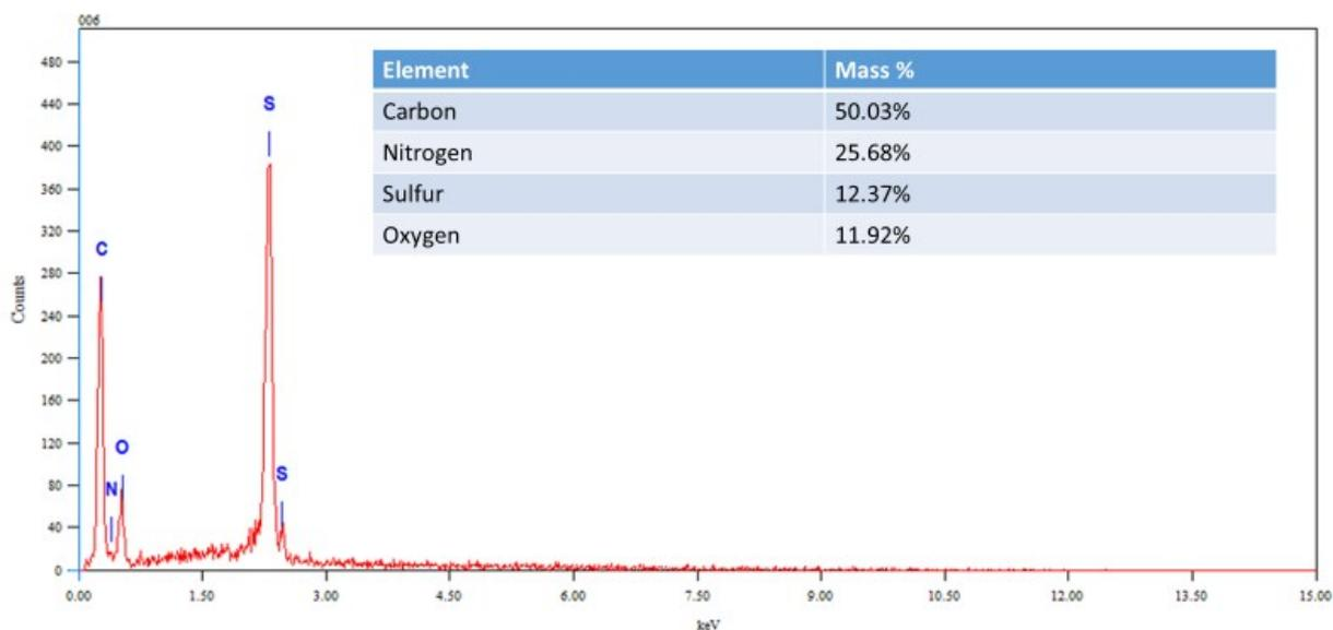
Figure S1: The EDX spectrum of the NS-CDs. Inset shows the content of elements in percentage.
