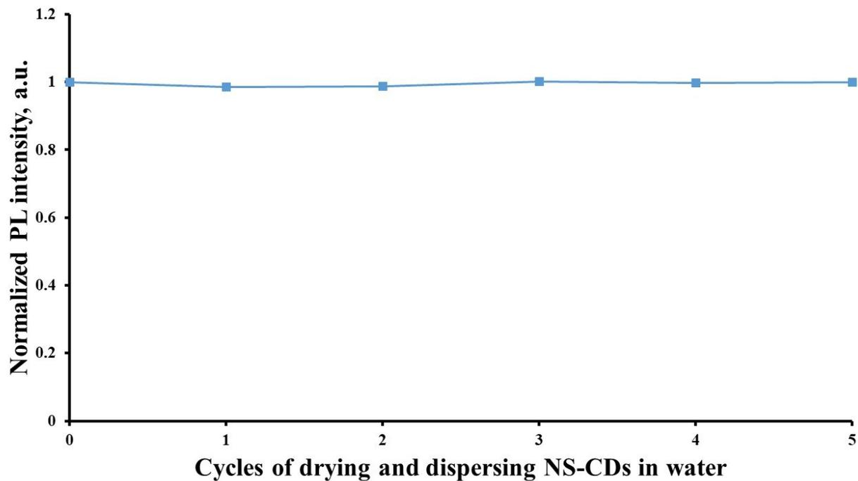
Figure S4: The effect of repetitive drying and dispersing on normalized PL intensity of NS-CDs.
