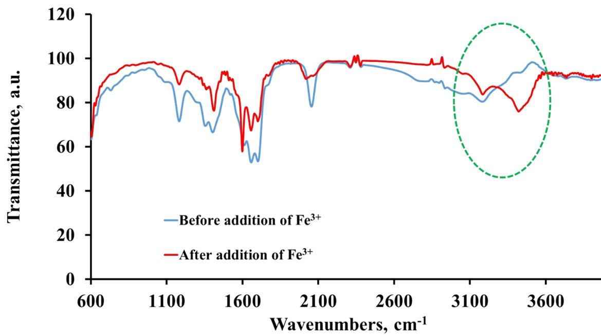
Figure S6: FTIR spectra of NS-CDs before and after the addition of Fe<sup>3+</sup>.
