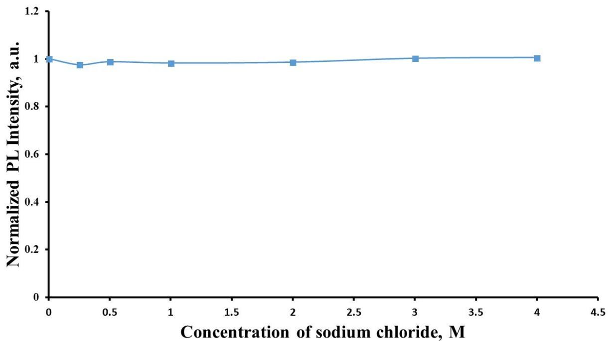
Figure S3: The effect of ionic strength on normalized PL intensity of NS-CDs.
