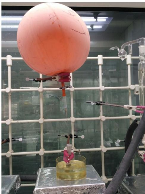
**Figure S5.** Experimental Setup for the carbonylation of the terminal acetylene.
