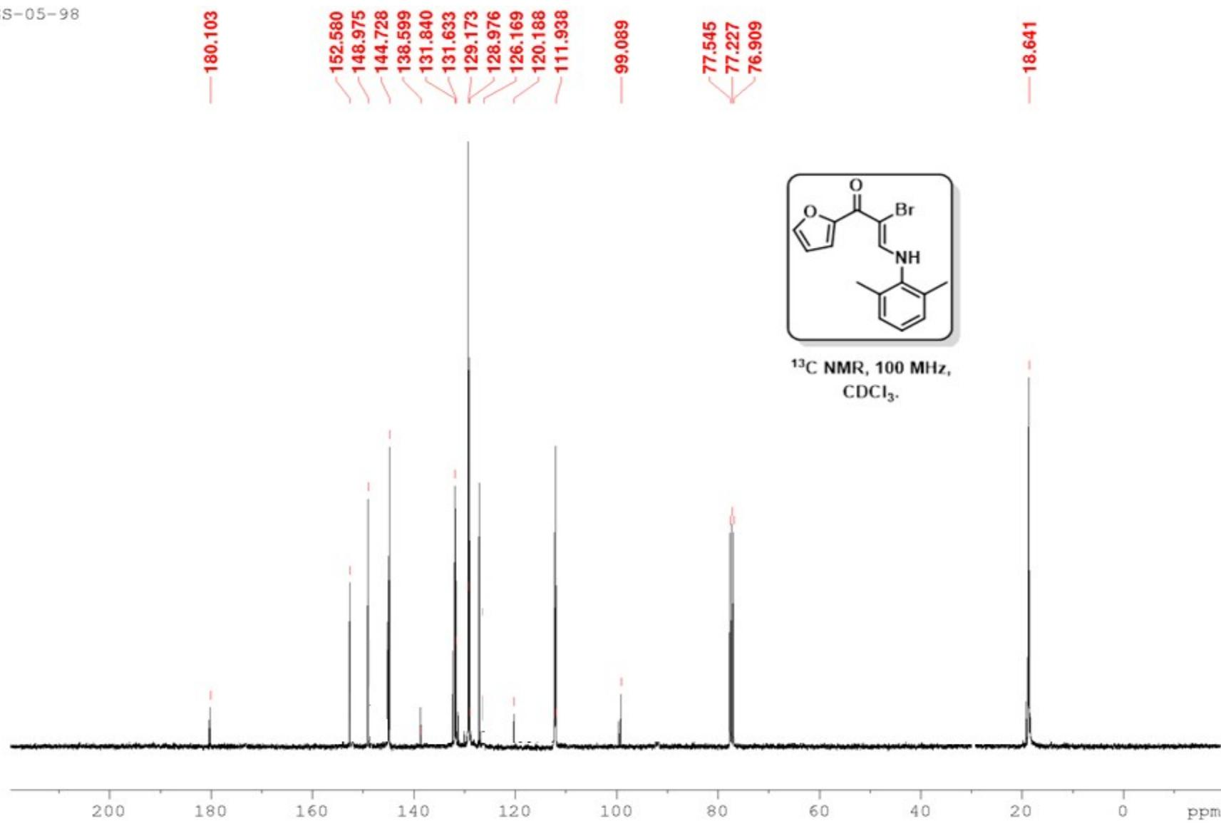
Figure 60:  $^{13}\text{C}$  NMR Compound 2x
