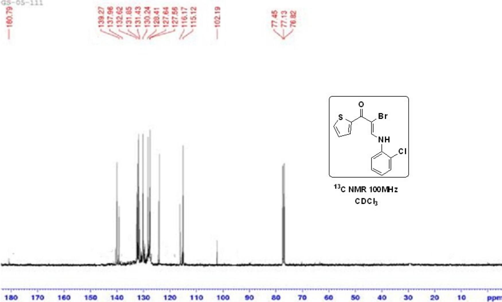
Figure 46: <sup>13</sup>C NMR Compound 2o
