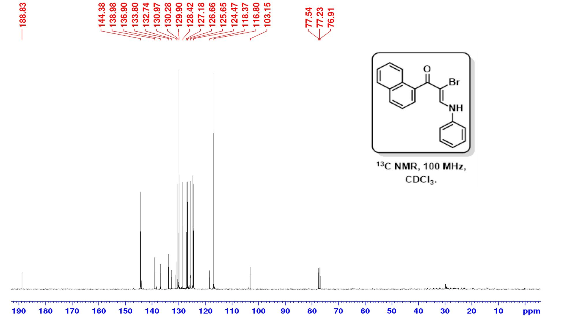
**Figure 28:  $^{13}\text{C}$  NMR Compound 2f**
