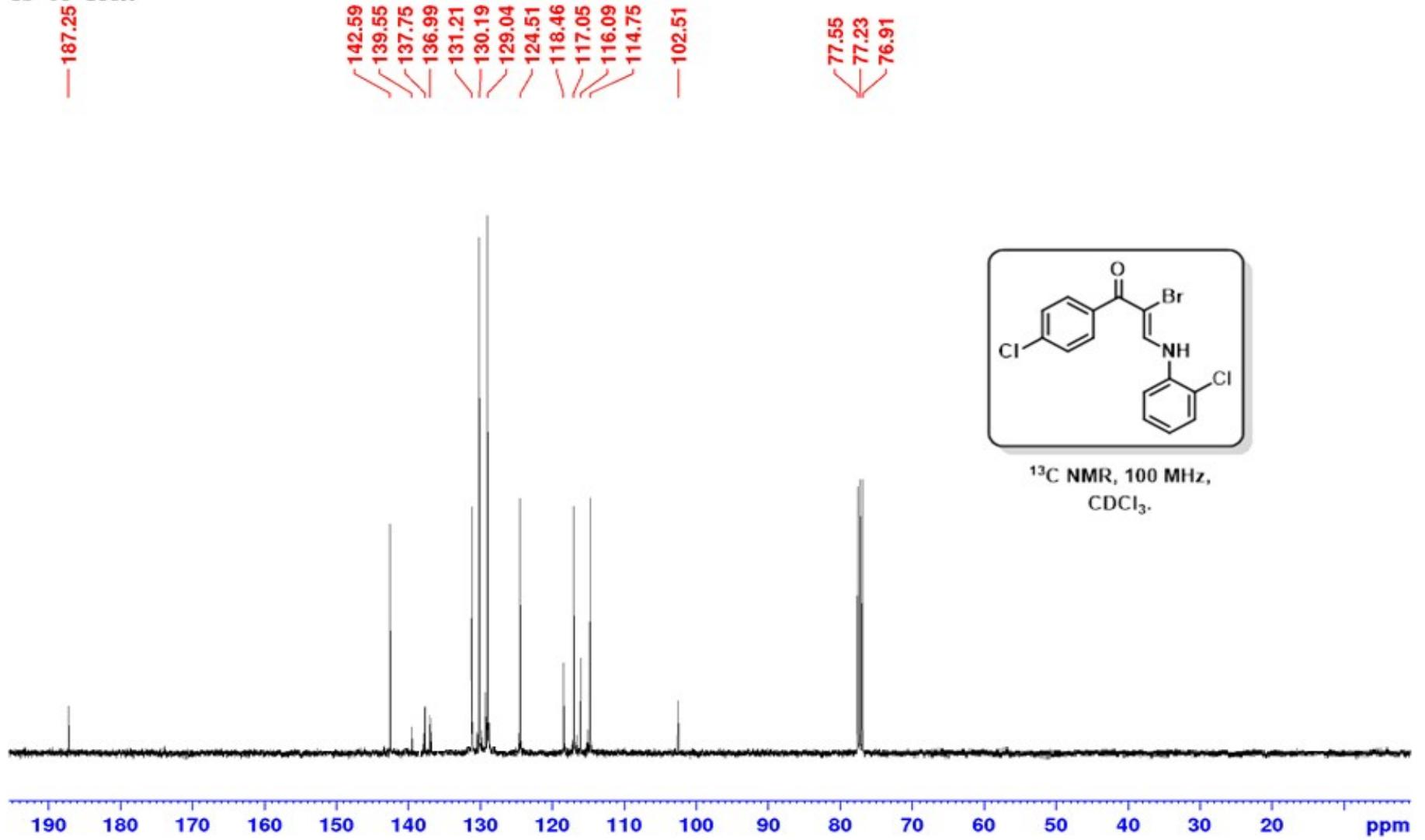
Figure 36:  $^{13}\text{C}$  NMR Compound 2j
