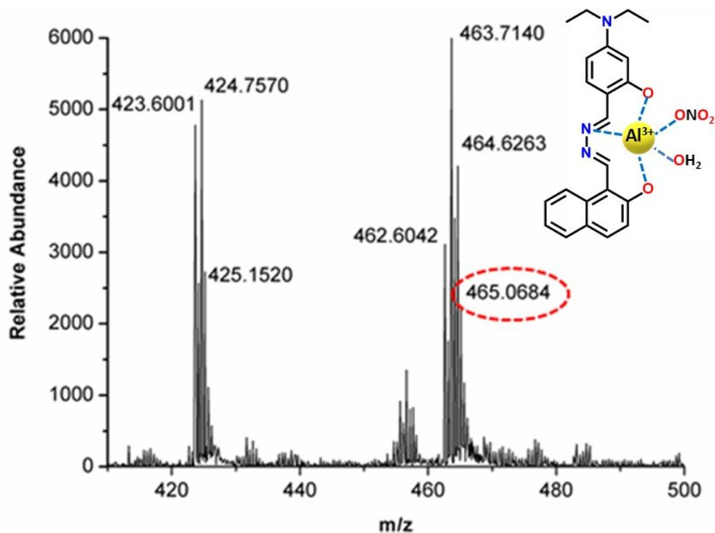
**Fig. S19:** ESI-MS spectrum of isolated solid (NDEA+Al<sup>3+</sup>).
