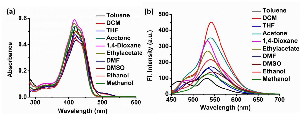
**Fig. S6:** (a) Absorbance and (b) Emission spectra of **NDEA** ( $1 \times 10^{-5}$  M) in the solvents of varying polarity.
