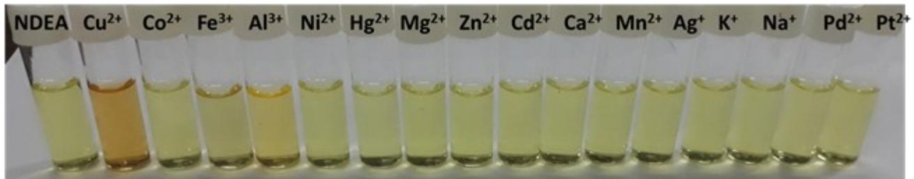
**Fig. S8:** Visual colour changes in the solution of **NDEA** ( $1 \times 10^{-5}$  M, DMSO : H<sub>2</sub>O : MeOH = 0.1 : 1.9 : 8.0, v/v, HEPES buffer, pH 7.4) on addition of 10 equiv. of different cations in H<sub>2</sub>O.
