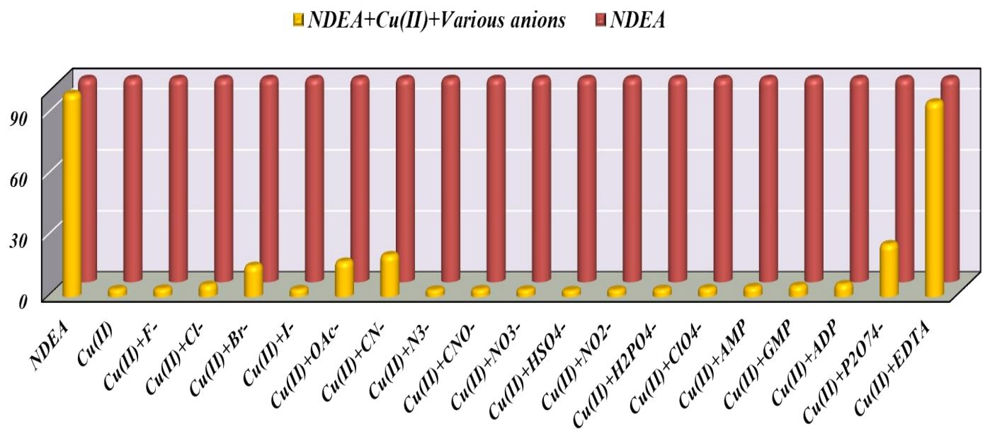
**Fig. S22:** Bar chart showing emission changes at  $\lambda_{\text{max}} = 534$  nm on the addition of various anions (3.0 eq.) in the solution of **NDEA+Cu<sup>2+</sup>** ( $1 \times 10^{-5}$  M, DMSO : H<sub>2</sub>O : MeOH = 0.1 : 1.9 : 8.0, v/v, HEPES buffer, pH 7.4)
