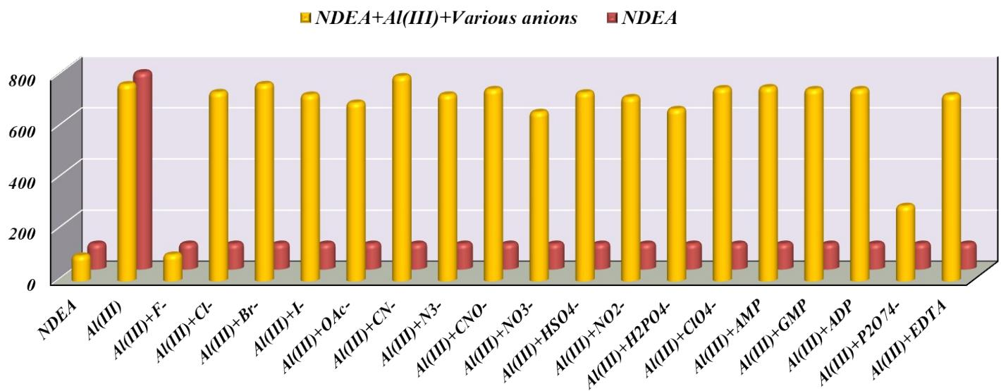
**Fig. S21:** Bar chart showing emission changes at  $\lambda_{\text{max}} = 552$  nm on the addition of various anions (3.0 eq. each) in the solution of **NDEA+Al<sup>3+</sup>** ( $1 \times 10^{-5}$  M, DMSO : H<sub>2</sub>O : MeOH = 0.1 : 1.9 : 8.0, v/v, HEPES buffer, pH 7.4).
