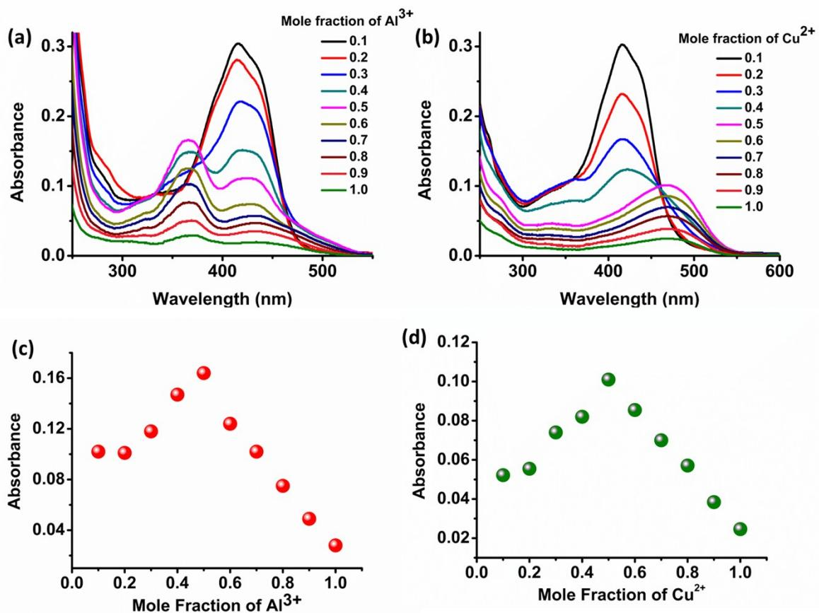
**Fig.S12:** Variation in the absorbance of NDEA ( $1 \times 10^{-5}$  M, DMSO : H<sub>2</sub>O : MeOH = 0.1 : 1.9 : 8.0, v/v, HEPES buffer, pH 7.4) against the mole fraction of (a) Al<sup>3+</sup> ions and (b) Cu<sup>2+</sup>ions. Their corresponding Job's plots against mole fraction of (c) Al<sup>3+</sup> ions at  $\lambda_{\max} = 362$  nm ( $1 \times 10^{-5}$  M, H<sub>2</sub>O) and (d) Cu<sup>2+</sup> ions at  $\lambda_{\max} = 471$  nm ( $1 \times 10^{-5}$  M) is shown.
