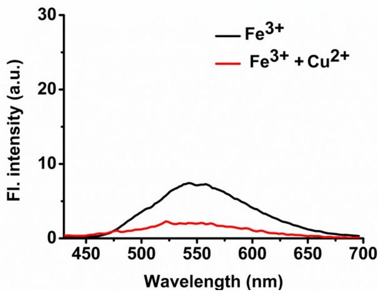
**Fig.S11:** Fluorescence spectra of **NDEA** ( $1 \times 10^{-5}$ M, DMSO : H<sub>2</sub>O : MeOH = 0.1 : 1.9 : 8.0, v/v, HEPES buffer, pH 7.4) showing quenching response of Cu<sup>2+</sup> ions towards **NDEA+Fe<sup>3+</sup>** ensemble.
