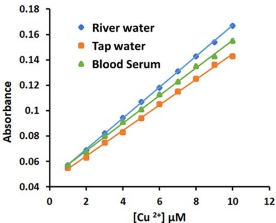
**Fig. S26:** Proof-of-concept experiments with NDEA (at  $\lambda_{\text{max}} = 471 \text{ nm}$ ) for determining Cu<sup>2+</sup> ions in real samples.
