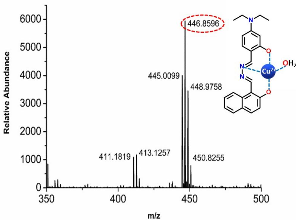
**Fig. S20:** ESI-MS spectrum of isolated solid (NDEA+Cu<sup>2+</sup>).
