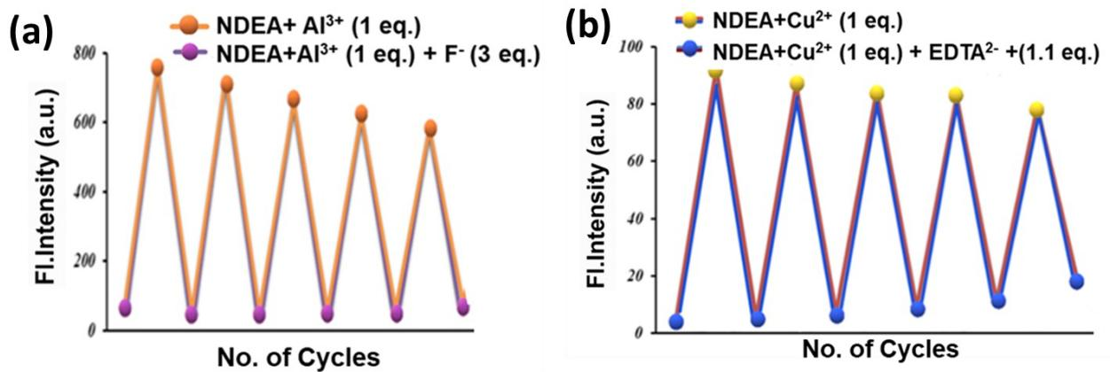
**Fig. S23:** Reversible cycles of NDEA ( $1 \times 10^{-5}$  M, DMSO : H<sub>2</sub>O : MeOH = 0.1 : 1.9 : 8.0, v/v, HEPES buffer, pH 7.4) (a) Al<sup>3+</sup> with F<sup>-</sup> and (b) Cu<sup>2+</sup> with EDTA<sup>2-</sup> respectively.
