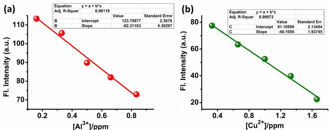
**Fig. S14:** Calibration curves for determination of the detection limit of NDEA ( $1 \times 10^{-5}$  M, DMSO : H<sub>2</sub>O : MeOH = 0.1 : 1.9 : 8.0, v/v, HEPES buffer, pH 7.4) for (a) Al<sup>3+</sup> ions (b) Cu<sup>2+</sup> ions using fluorescence titrations data.
