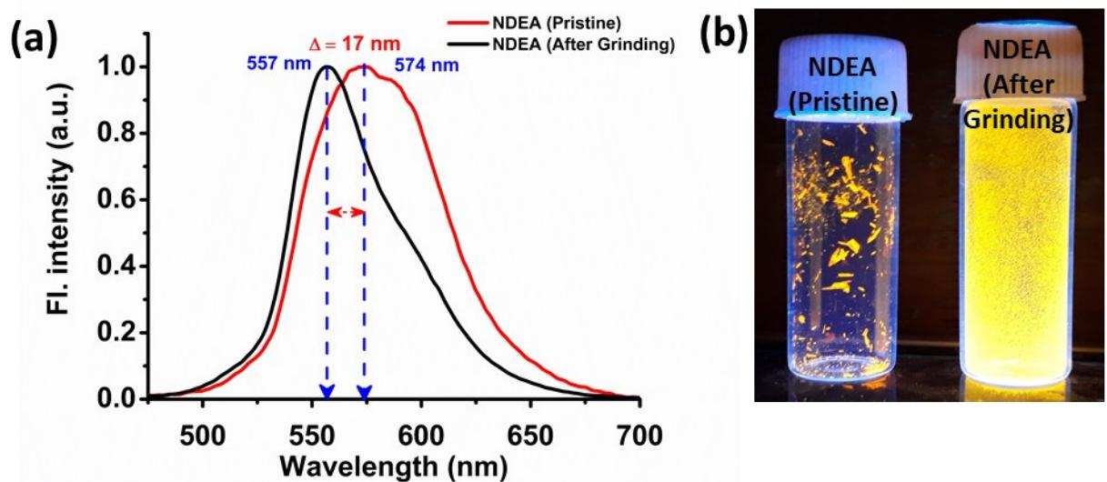
**Fig. S24:** (a) Normalized solid-state emission spectra of NDEA (pristine) and NDEA obtained after grinding and (b) the same as seen in UV lamp.
