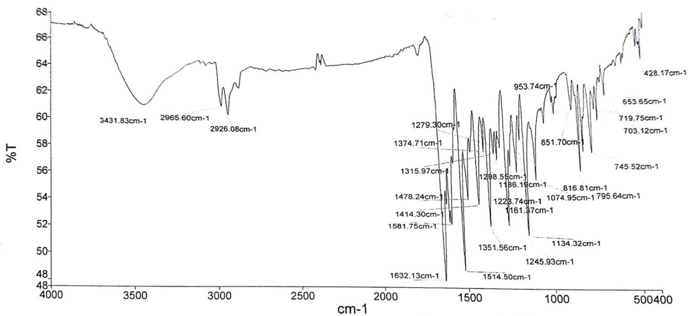
**Fig. S1:** IR spectrum of NDEA at room temperature.
