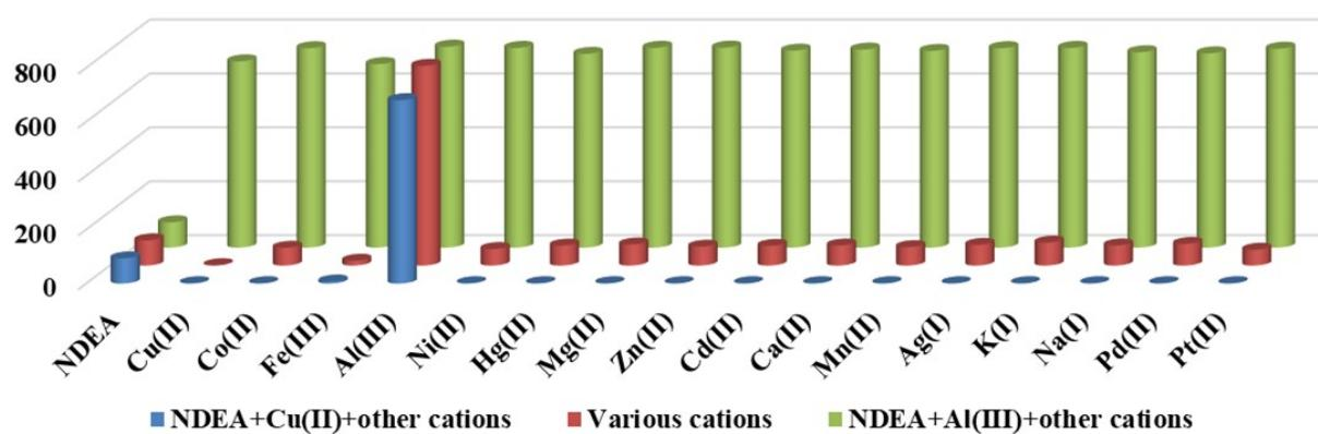
**Fig. S15:** Bar diagrams showing emission responses from NDEA ( $1 \times 10^{-5}$  M, DMSO : H<sub>2</sub>O : MeOH = 0.1 : 1.9 : 8.0, v/v, HEPES buffer, pH 7.4) upon addition of 10 equiv. of various metal ions (red bars). The green and blue coloured bars depict interference test of 10 equiv. of Al<sup>3+</sup> and Cu<sup>2+</sup> at  $\lambda_{\text{em}} = 552$  and 534 nm respectively.
