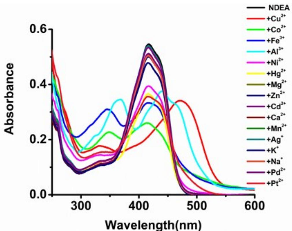
**Fig. S9:** Absorption spectra of **NDEA** ( $1 \times 10^{-5}$  M, DMSO : H<sub>2</sub>O : MeOH = 0.1 : 1.9 : 8.0, v/v, HEPES buffer, pH 7.4) in the presence of various cations (10 equiv. each).
