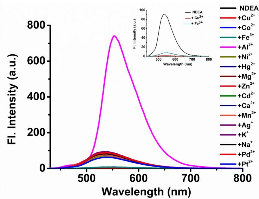
**Fig. S10:** Fluorescence spectra of **NDEA** ( $1 \times 10^{-5}$ M, DMSO : H<sub>2</sub>O : MeOH = 0.1 : 1.9 : 8.0, v/v, HEPES buffer, pH 7.4) in the presence of various cations (10 eq.), inset shows the quenching response of Cu<sup>2+</sup> and Fe<sup>3+</sup> ions.
