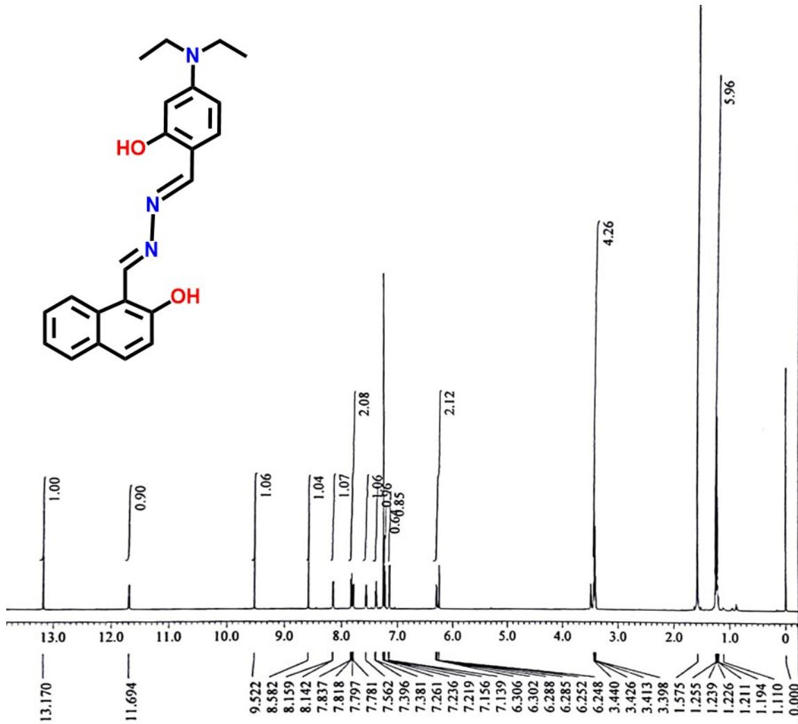
Fig. S2: <sup>1</sup>H-NMR spectrum of NDEA in CDCl<sub>3</sub> at room temperature.
