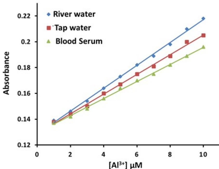
**Fig. S25:** Proof-of-concept experiments with NDEA (at  $\lambda_{\text{max}} = 362 \text{ nm}$ ) for determining Al<sup>3+</sup> ions in real samples.
