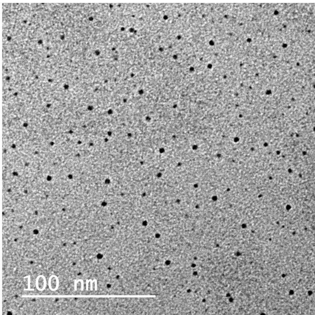
**Figure S4 shows TEM image of MAPbBr<sub>3</sub> using Oleic and oleylamine (100/200 $\mu$ l) in CHCl<sub>3</sub>**
