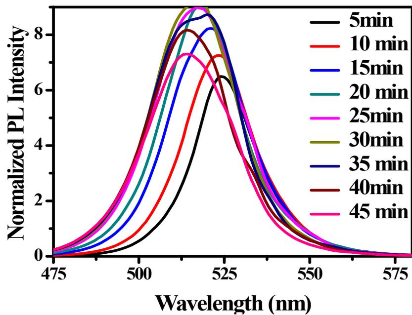
Figure S8 shows shifted time dependent PL studies of perovskite solution in the presence of 400 μL of water
