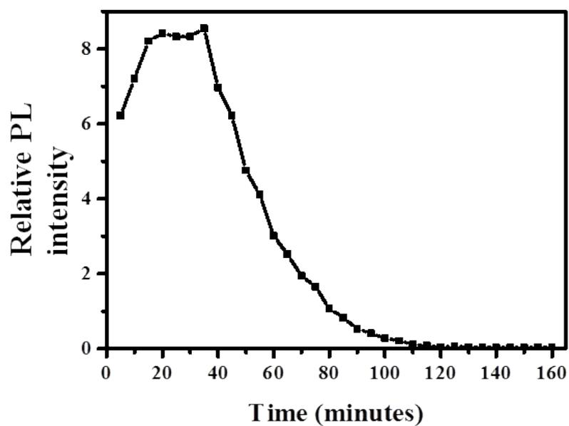
**Figure S9 shows decreasing relative PL intensity and degradation of perovskite solution in 150 minutes in the presence of water**
