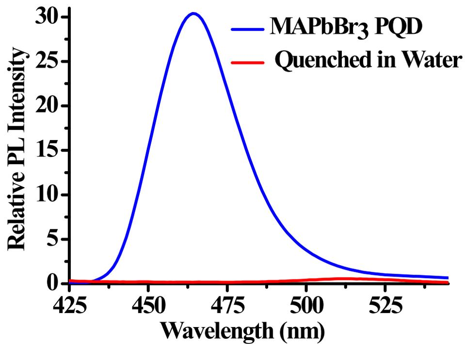
Figure S7 Quenching of MAPbBr<sub>3</sub> solution (synthesized using oleic acid) in small amount of water
