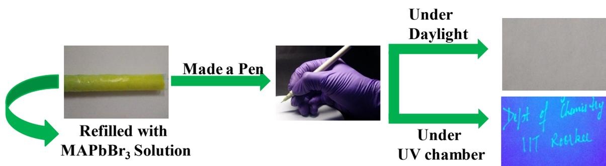
Figure S10 refilling of pen and application as fluorescent ink
