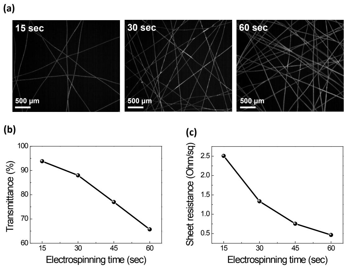
**Figure S5** (a) Optical microscopy images of PAA fiber webs with varying electrospinning times. (b) Optical transmittance and (c) sheet resistance of Ag NTR-CPI as a function of electrospinning time.
