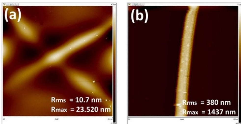
**Figure S2** AFM image of (a) Ag NTR-CPI and (b) non-embedded Ag NTR on glass (The scan area is 20  $\mu\text{m} \times 20 \mu\text{m}$ )
