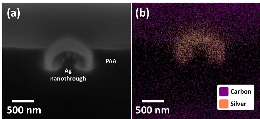
**Figure S3** Cross-sectional (a) SEM image and (b) EDAX mapping image of Ag NTR embedded in PAA film as prepared in FIB
