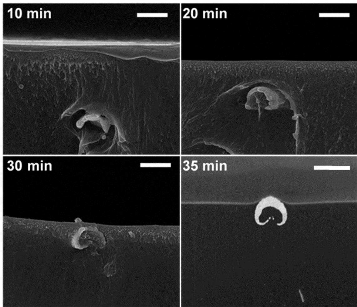
**Figure S1** Cross-section SEM images of Ag NTR embedded in CPI film with varying PAA drying times. The scale bar is 1  $\mu\text{m}$
