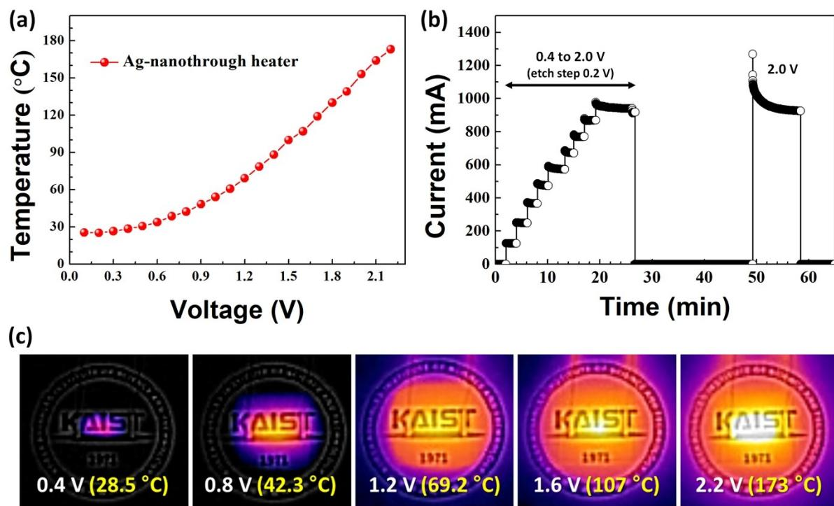
**Figure S7** (a) Temperature profile of the Ag NTR-CPI by joule heating under diverse voltages. (b) Current response of the Ag NTR-CPI as a function of applied voltages ranging 0 to 2.0 V in each step for 30 sec and (b) 0 to 2.4 V in each for 5 min. (c) IR camera images of the each voltage with temperature.
