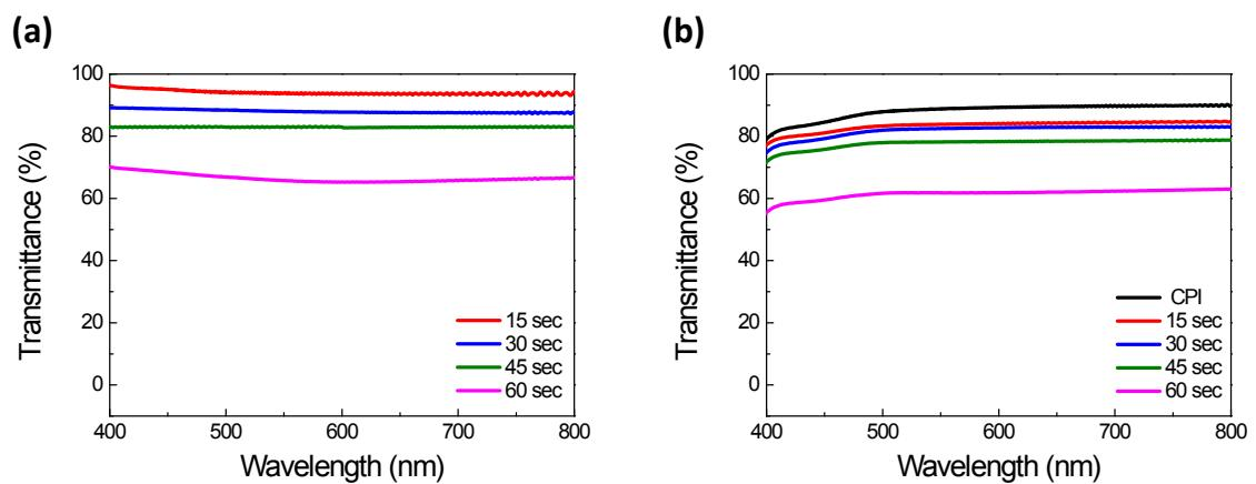
**Figure S4** Optical transmittance spectra of Ag NTR-CPI film with varying electrospinning time. (a) Baseline with bare CPI film and (b) ambient air
