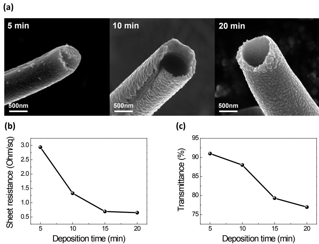
**Figure S6** (a) Cross-section SEM images of Ag NTR including PAA core template with varying deposition time. (b) Sheet resistance and (c) optical transmittance of Ag deposition time of Ag NTR-CPI as a function of electrospinning time.
