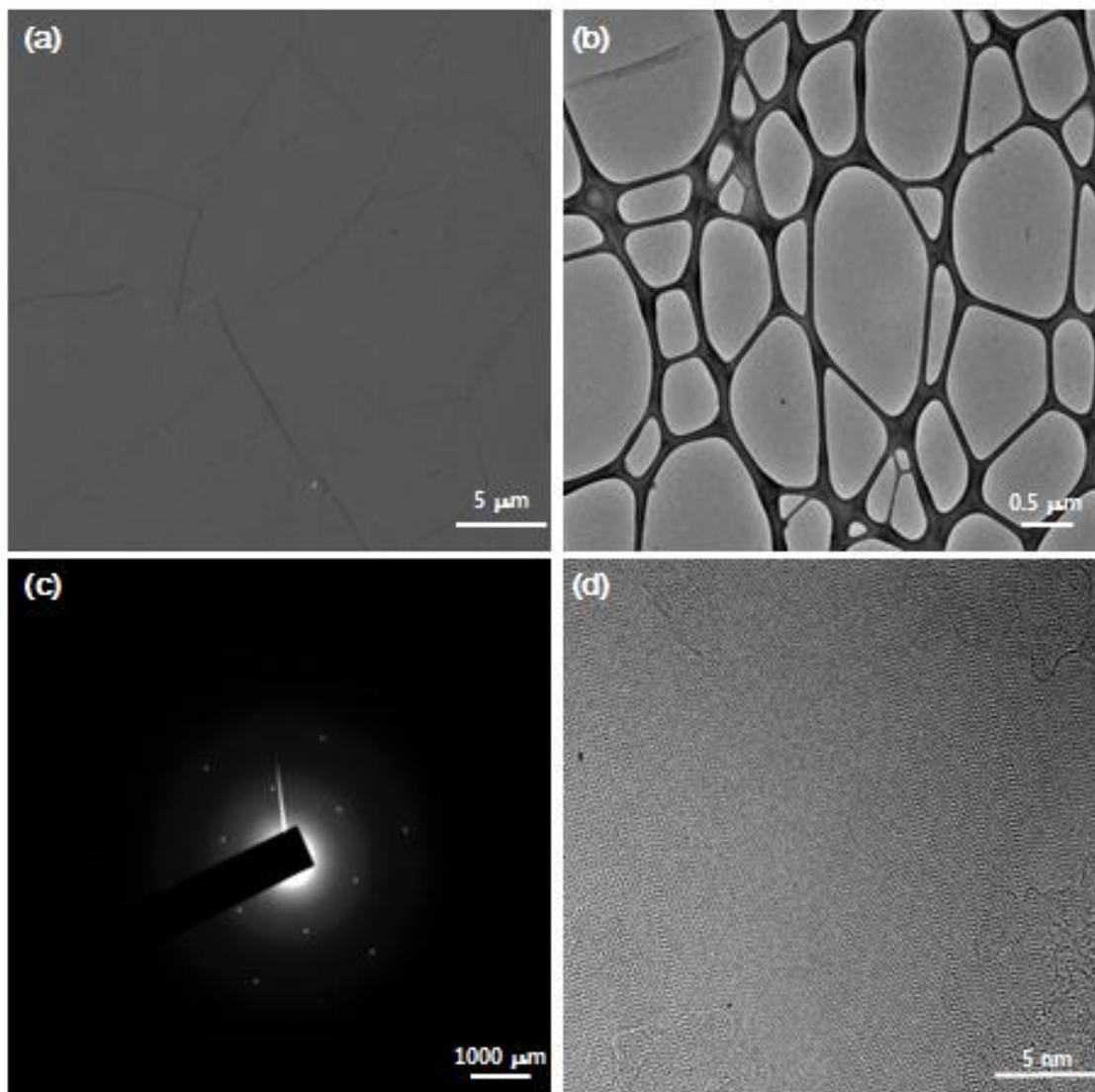
Fig. S1 (a) Representative SEM and (b) HRTEM images of the monolayer graphene film with (c) distinctive SAED pattern. (d) Representative Cs-corrected STEM image of the monolayer graphene.
