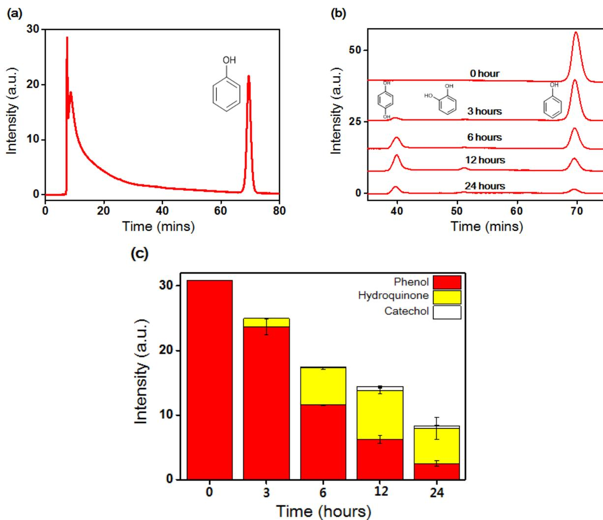
Fig. S2 (a) HPLC analysis of hydrogen peroxide (100 mM) and phenols (1 mM). Hydrogen peroxide show strong, broad signals peaking at 7.43 and 8.65 minutes. (b) Time-dependent HPLC analysis and (c) quantified intensities with 9 cm<sup>2</sup> graphene film after 0, 3, 6, 12 and 24 hours of incubation with 1 mM phenols and 100 mM hydrogen peroxide.
