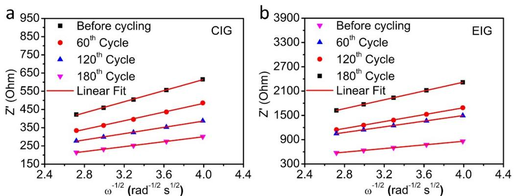
**Fig. S14** Relationship between  $Z'$  and  $\omega^{-1/2}$  of the (a) CIG and (b) EIG electrodes.
