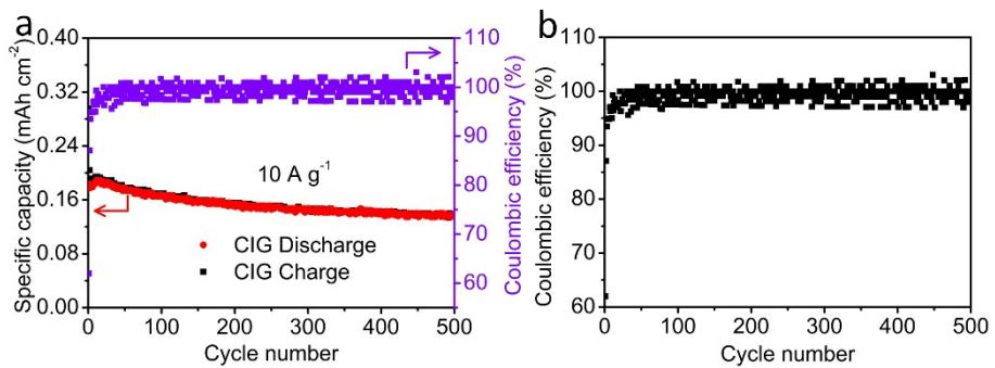
**Fig. S13** (a) Cycling performance of the CIG/LiFePO<sub>4</sub> full-cell at 10 A g<sup>-1</sup> over 500 cycles. (b) Coulombic efficiency of the CIG/LiFePO<sub>4</sub> full-cell at 10 A g<sup>-1</sup> on an expanded scale.
