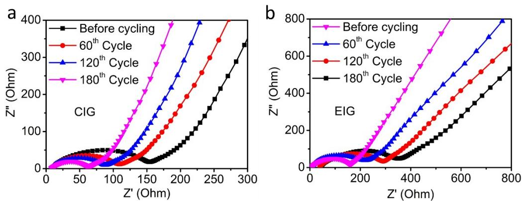
**Fig. S15** Nyquist plots of the (a) CIG and (b) EIG electrodes at different cycles from  $10^5$  to 0.01 Hz.
