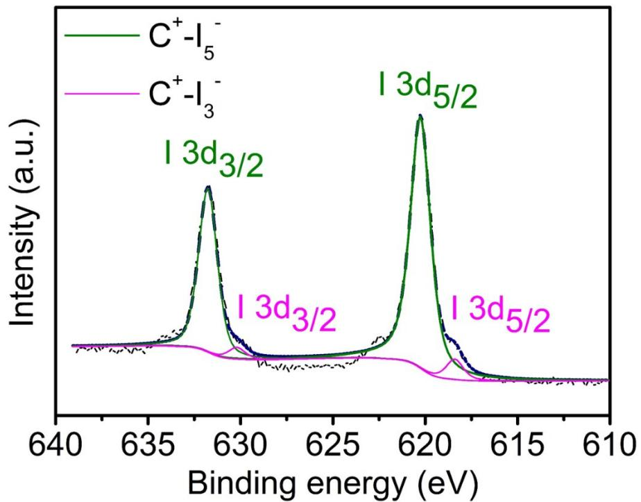
**Fig. S1** I 3d XPS spectrum of the EIG composite.
