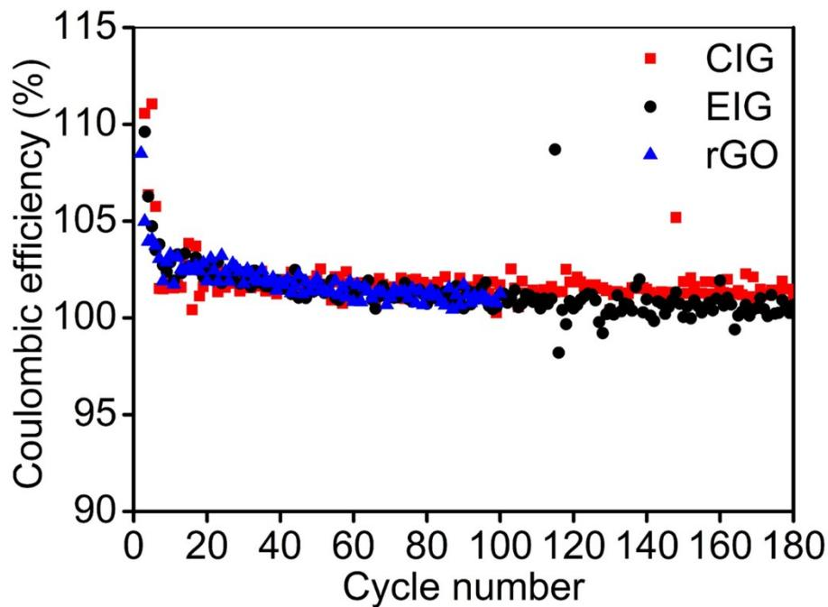
**Fig. S5** Coulombic efficiencies of the CIG, EIG and rGO anodes at 500 mA g<sup>-1</sup>.
