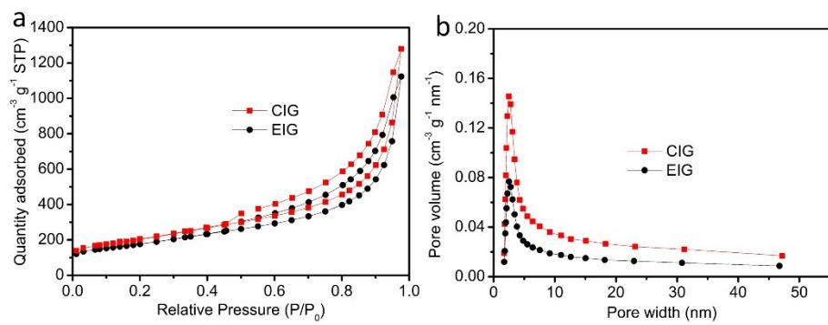
**Fig. S4** (a) Nitrogen adsorption-desorption isotherms of CIG and EIG. (b) BJH Pore-size distributions of CIG and EIG.
