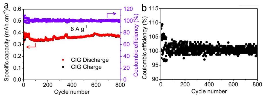
**Fig. S11** (a) Cycling performance of the CIG electrode at  $8 \text{ A g}^{-1}$  over 800 cycles. (b)
