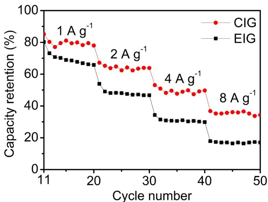
**Fig. S10** The capacity retention of the CIG and EIG anodes cycled at high rates.
