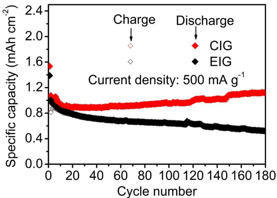
**Fig. S6** Cycling performance of the CIG and EIG electrodes at 500 mA g<sup>-1</sup>.
