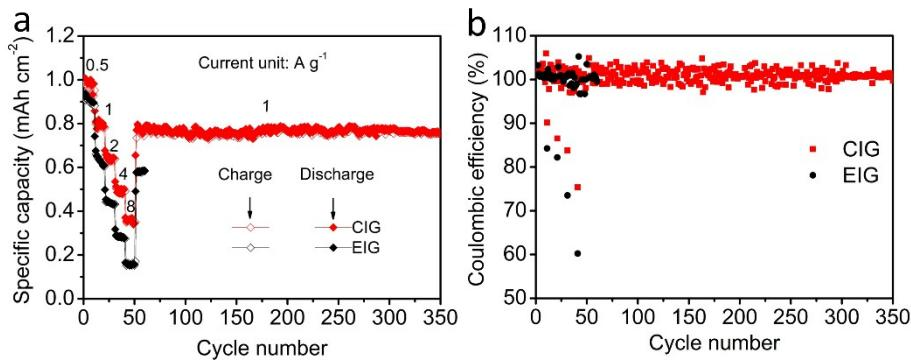
**Fig. S8** (a) Rate performance and (b) coulombic efficiencies of the CIG and EIG electrodes at the corresponding current densities after 5 cycles' activation at  $0.2 \text{ A g}^{-1}$ .
