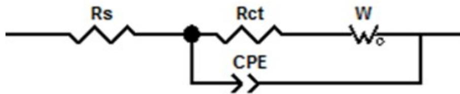
**Fig. S7** The equivalent circuit model of electrochemical impedance spectroscopy (EIS).
