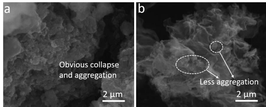
**Fig. S16** SEM images of the (a) EIG and (b) CIG composites after 180 cycles at  $0.5 \text{ A g}^{-1}$ .
