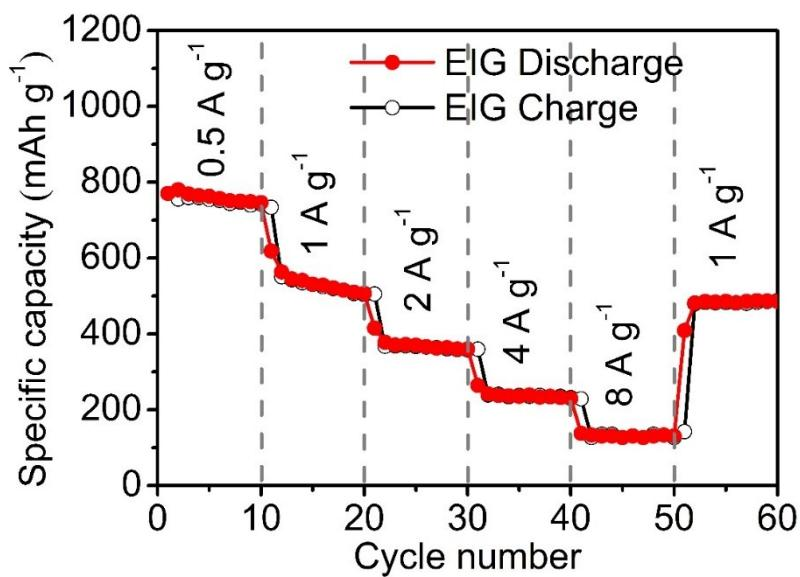
**Fig. S9** Rate performance of the EIG electrode at corresponding current densities from  $0.5 \text{ A g}^{-1}$  to  $8 \text{ A g}^{-1}$  after 5 cycles' activation at the current density of  $0.2 \text{ A g}^{-1}$ .
