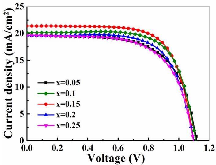
Figure S1  $J$ - $V$  curves of the  $\text{FA}_{1-x}\text{Cs}_x\text{PbI}_3$  perovskite PSCs with different Cs contents ( $x$  values).
