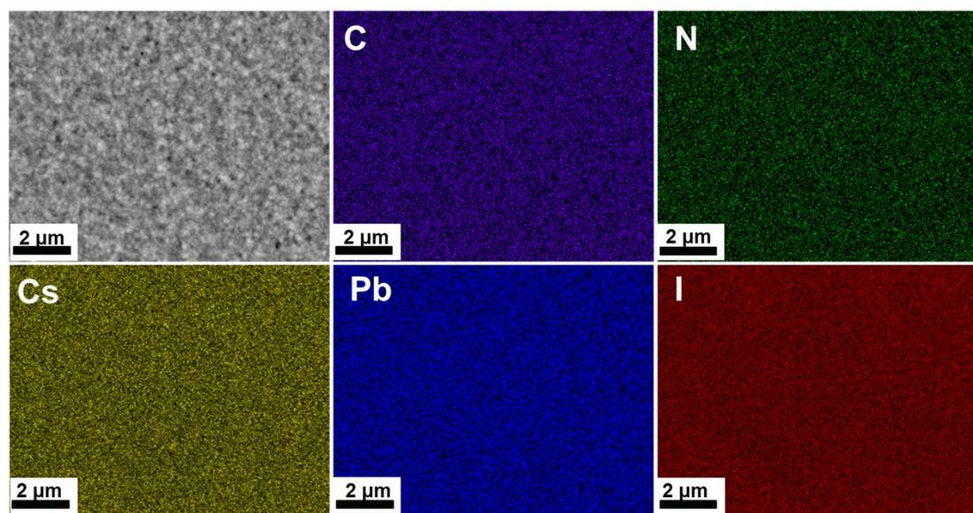
Figure S4 EDS mapping of  $\text{MA}_{0.1}\text{FA}_{0.75}\text{Cs}_{0.15}\text{PbI}_3$  films on ZnO layer.
