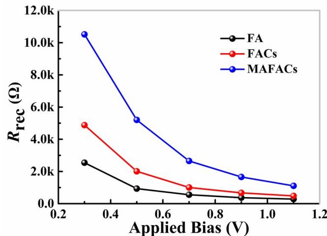
Figure S8 Plots of  $R_{rec}$  at different applied biases extracted from impedance measurements of the three devices under dark conditions.
