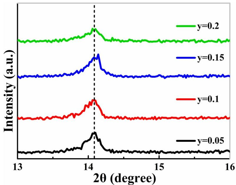
Figure S2 Magnified XRD patterns of the (101) lattice plane of  $\text{MA}_y\text{FA}_{0.85-x}\text{Cs}_{0.15}\text{PbI}_3$  thin films with various MA contents ( $y$  values).
