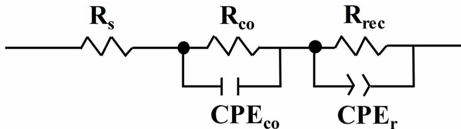
Figure S9 The equivalent circuit model for PSCs in EIS under AM 1.5G illumination.
