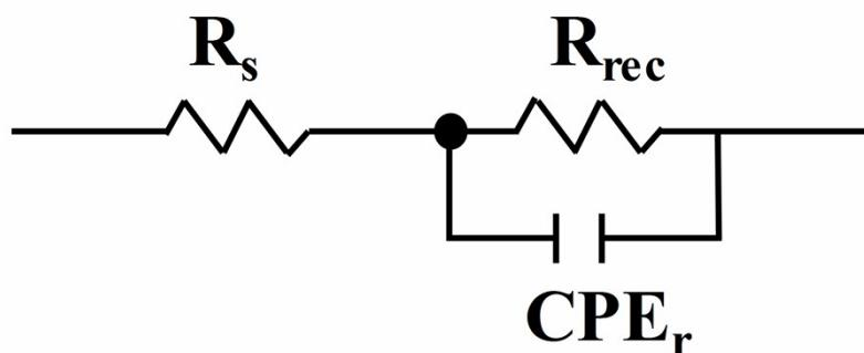
Figure S7 The equivalent circuit model for PSCs in EIS under dark condition.
