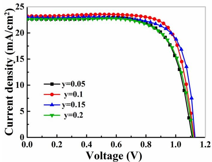
Figure S3  $J$ - $V$  curves of the  $\text{MA}_y\text{FA}_{0.85-y}\text{Cs}_{0.15}\text{PbI}_3$  perovskite PSCs with different MA contents ( $y$  values).
