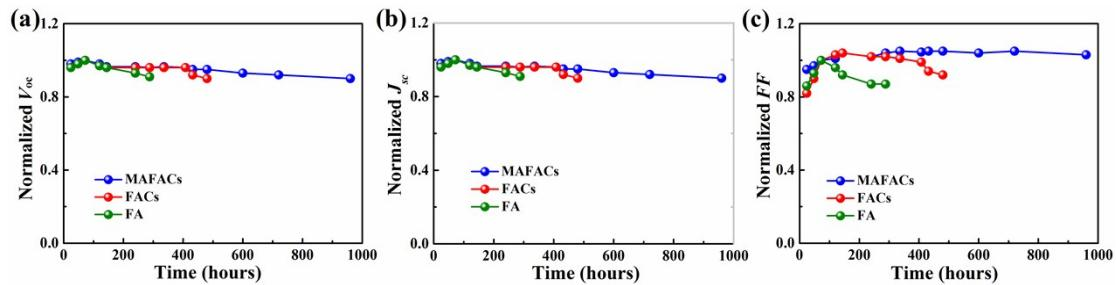
Figure S5 The long-term (a)  $V_{oc}$  (b)  $J_{sc}$  (c) FF of  $\text{FAPbI}_3$ ,  $\text{FA}_{0.85}\text{Cs}_{0.15}\text{PbI}_3$  and  $\text{MA}_{0.1}\text{FA}_{0.75}\text{Cs}_{0.15}\text{PbI}_3$  devices without encapsulation stored in the ambient environment with relative humidity of 40–60% at room temperature.
