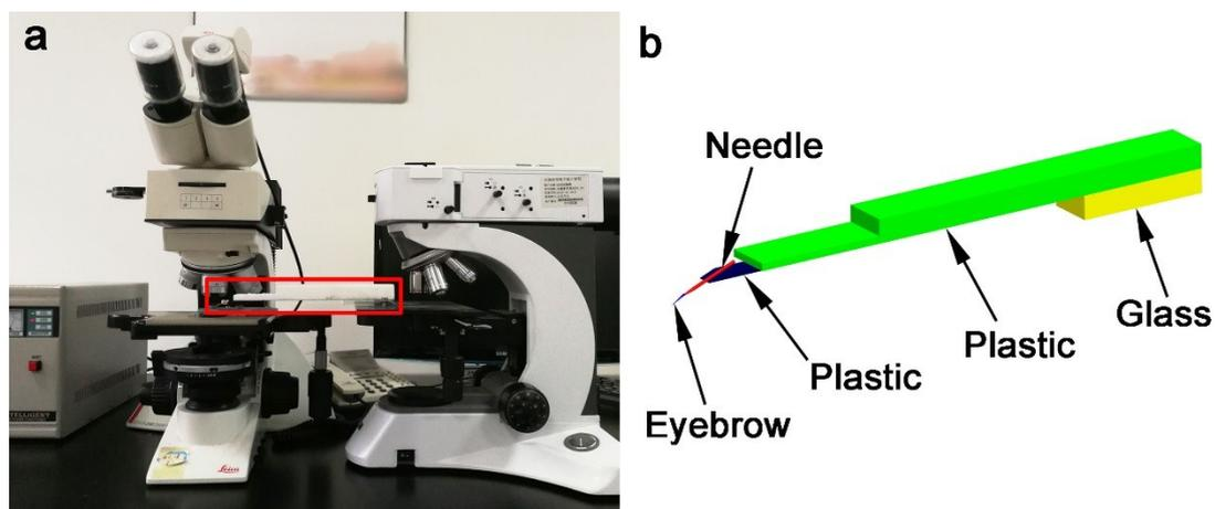
Extended Data Figure 1 (a) Photograph of an optical (left) and metallurgical (right) microscopes and (b) schematic diagram of an eyebrow fixed on a needle connecting plastics and a glass block marked by the red rectangle in (a).
