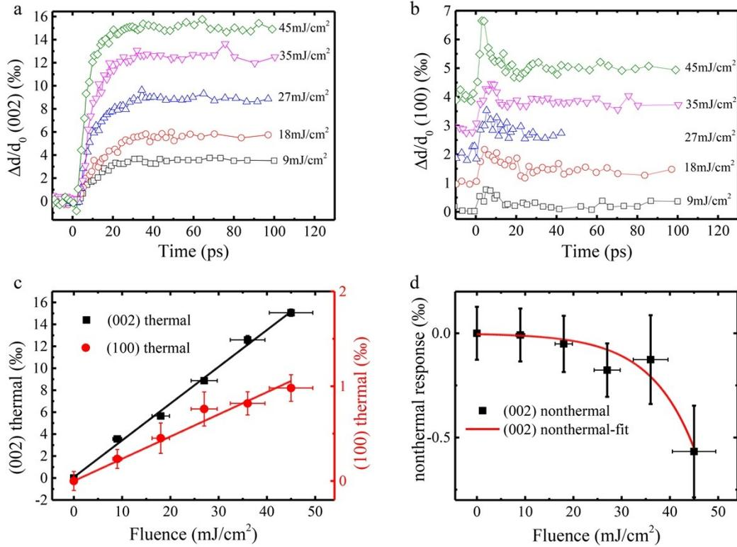
Figure S2. Pump laser fluence dependence of structural dynamics of MWCNTs. (a) and (b) show the temporal evolutions of the (002)- and (100)- plane lattice spacings for the laser fluences indicated. (c) fluence dependence of the magnitudes of thermal lattice changes of the (002)- and (100)-plane estimated at time delay > 30 ps. (d) fluence dependence of the maximal magnitudes (at  $\sim 3$  ps) of nonthermal lattice changes of the (002)-plane.
