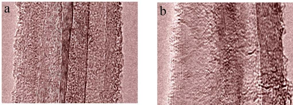
Figure S3. TEM lattice images of MWCNTs taken after pump laser irradiation of (a) 35 mJ cm<sup>-2</sup> and (b) 100 mJ cm<sup>-2</sup>, respectively. In (a) the MWCNTs remain intact after pump laser excitation, while in (b) visible structural damages occur, as evidenced by the disordered layers and the ablated layers.
