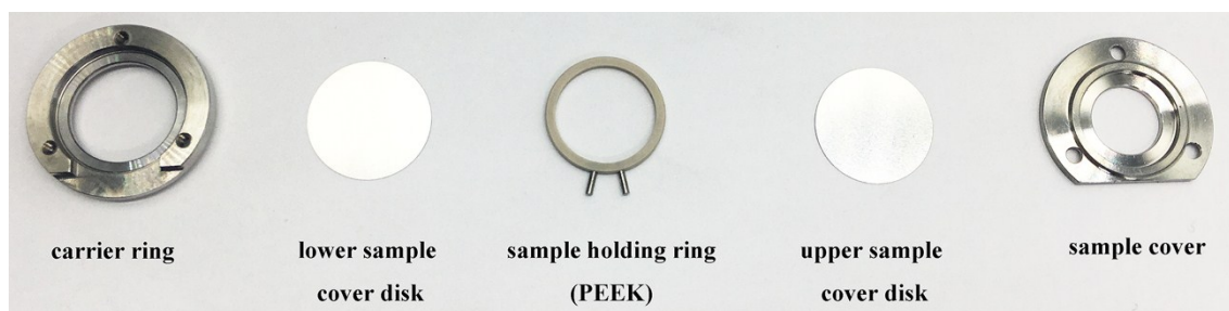
Fig. S1 The sample holder used in “liquids” thermal conductivity test model.
