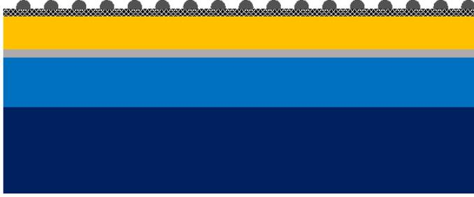
Figure S1: Scheme of the sensor (dimensions not to scale). From the top: Ti evaporated (dark gray islands), graphene monolayer (black and white), Au layer (yellow), Ti layer for proper sticking (gray), SiO<sub>2</sub> insulator layer (light blue), Si substrate (dark blue).
