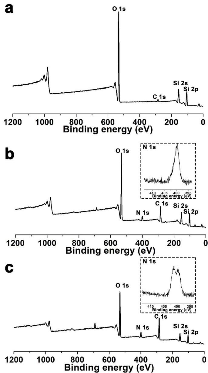
**Fig. S2** Typical XPS wide-scan spectra of SiO<sub>2</sub> (a), SiO<sub>2</sub>-NH<sub>2</sub> (b) and SiO<sub>2</sub>-Ad (c), and N 1s core-level spectra of SiO<sub>2</sub>-NH<sub>2</sub> (inset of b) and SiO<sub>2</sub>-Ad (inset of c).
