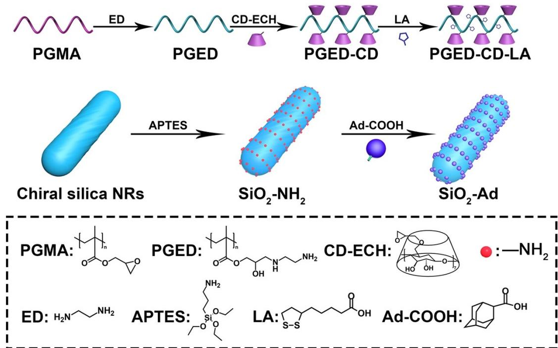
**Fig. S1** Schematic illustration of preparation processes of polycations and surface functionalized of chiral silica NRs.
