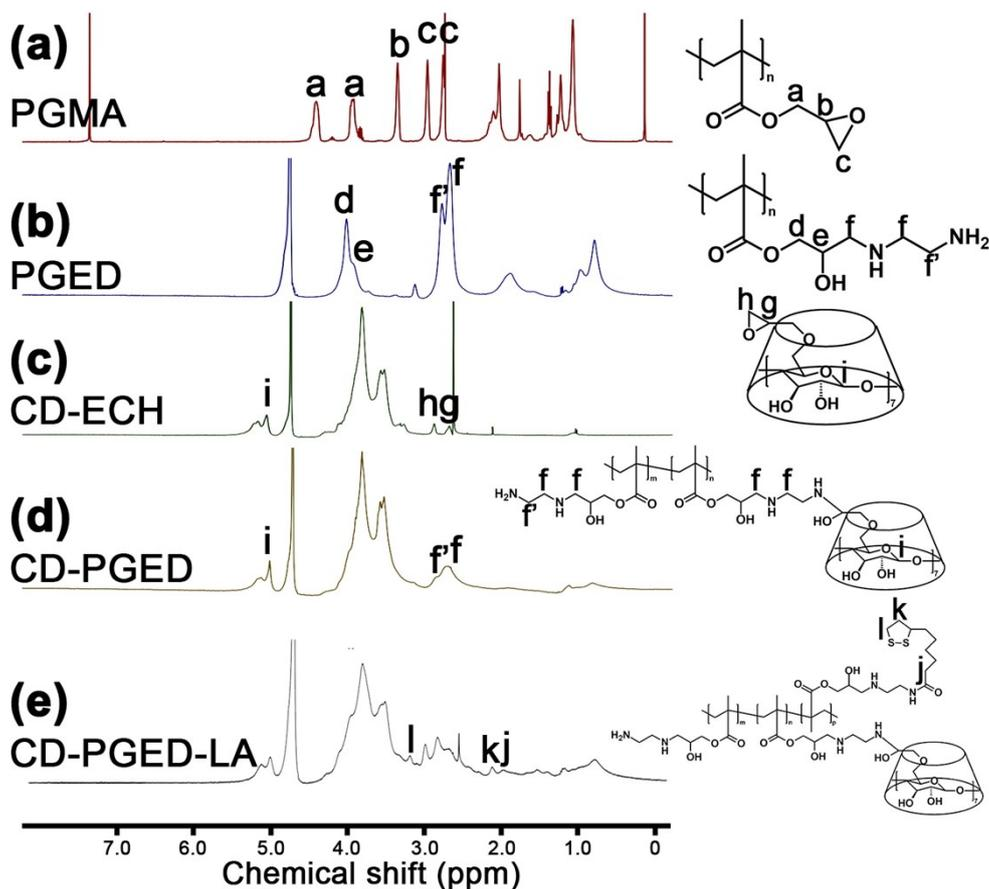
**Fig. S3** 400 MHz  $^1\text{H}$  NMR spectra of PGMA (a), PGED (b), ECH-CD (c), PGED-CD (d) and PGED-CD-LA (e). The chemical structures of PGMA, PGED, ECH-CD, PGED-CD and PGED-CD-LA were characterized by  $^1\text{H}$  NMR spectra (Figure S3).
