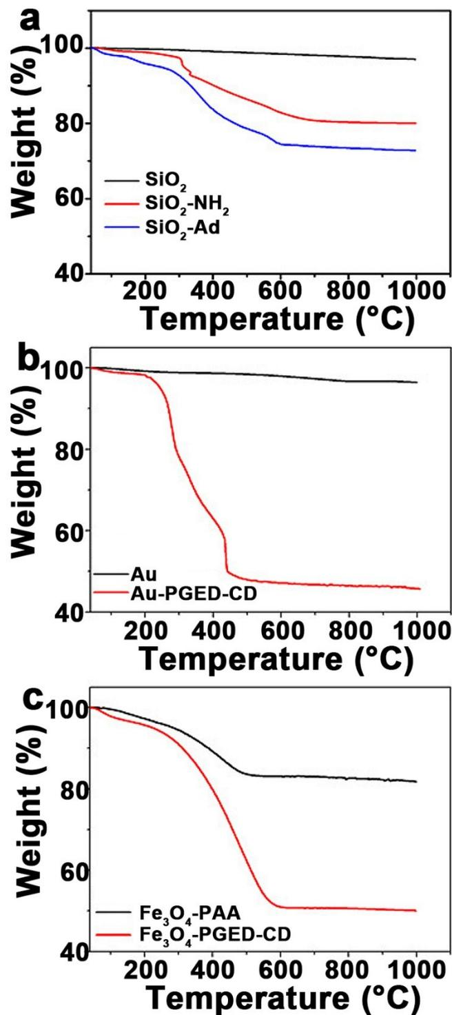
Fig. S4 TG analysis of SiO<sub>2</sub>-Ad (a), Au-PGED-CD (b) and Fe<sub>3</sub>O<sub>4</sub>-PGED-CD (c).
