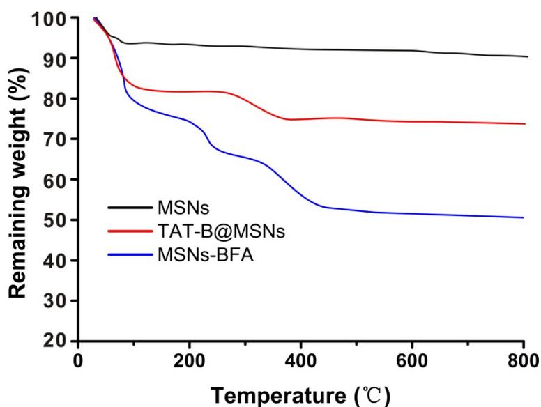
**Fig. S3** Thermogravimetric analysis of MSNs (black), TAT-B@MSNs (red), and MSNs-BFA (blue).
