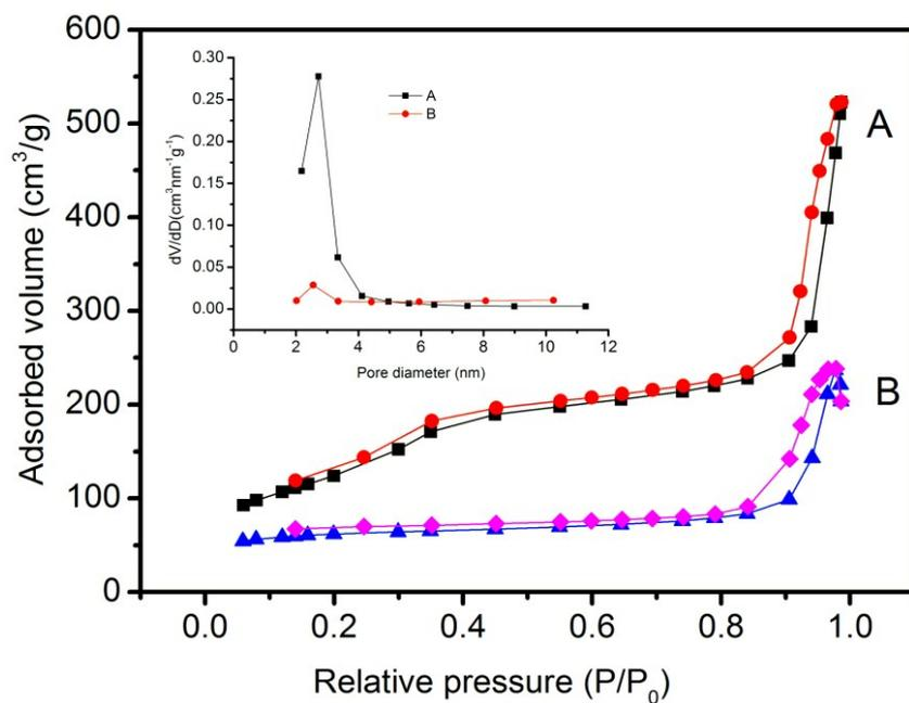
**Fig. S4** BET N<sub>2</sub> adsorption-desorption curves of TAT-B@MSNs (A) and MSNs-BFA (B), Insert, corresponding pore size distributions of TAT-B@MSNs and MSNs-BFA based on BJH method.
