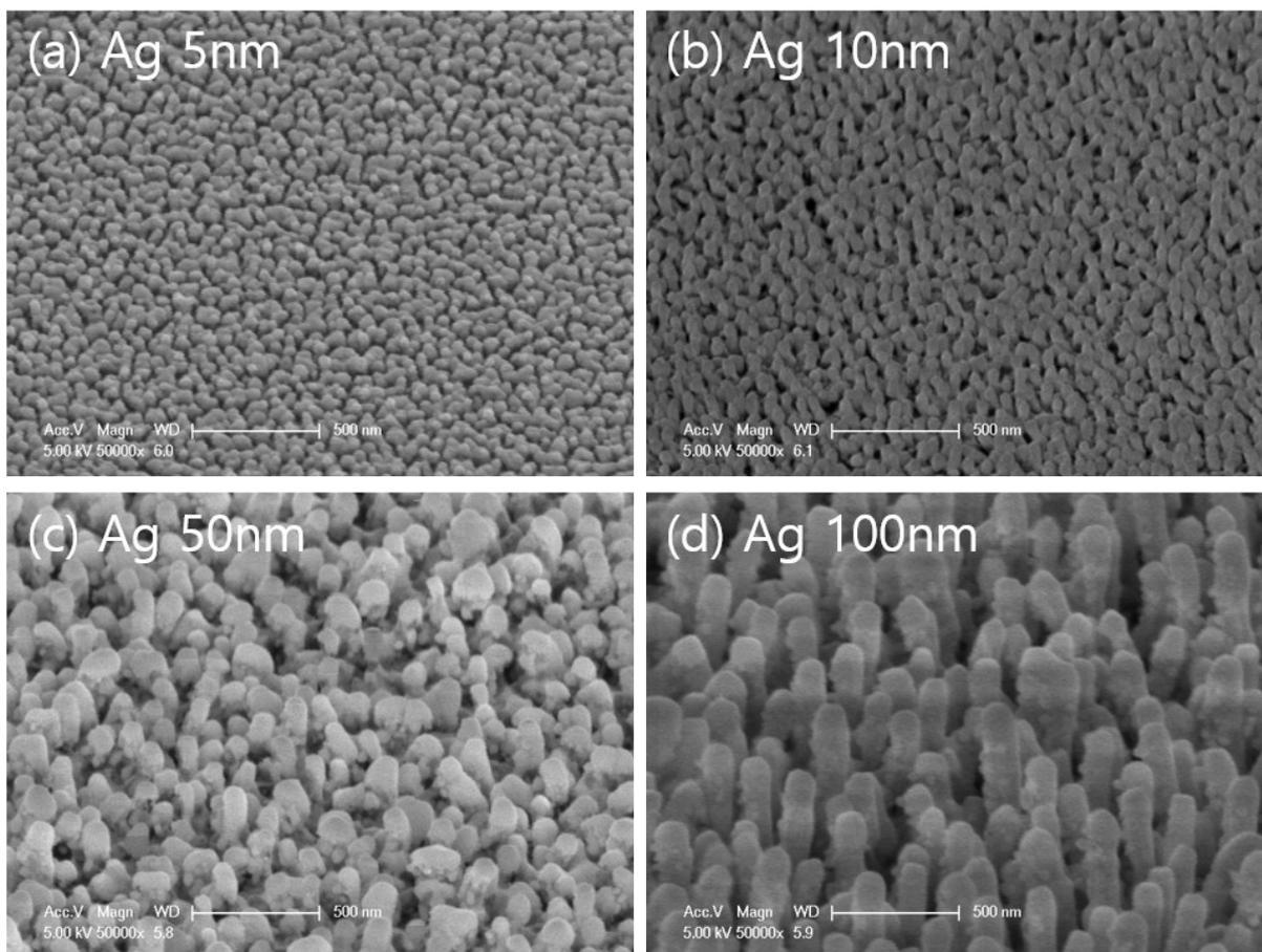
**Fig. S8** (a) Scanning electron microscopy (SEM, 45° tilt view) images of the AgCl nanostructure with different Ag thickness (a) 5 nm, (b) 10 nm, (c) 50 nm, and (d) 100 nm. Cl<sub>2</sub> plasma treatment time was 45 s.
