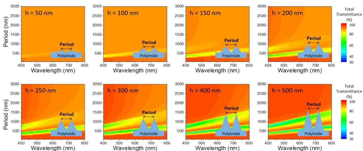
**Fig. S1** (a) Calculated total transmittance ( $T_{\text{total}}$ ) of the nanostructured plastic film as functions of period and height of nanostructure. Gap was set to be 0 nm.
