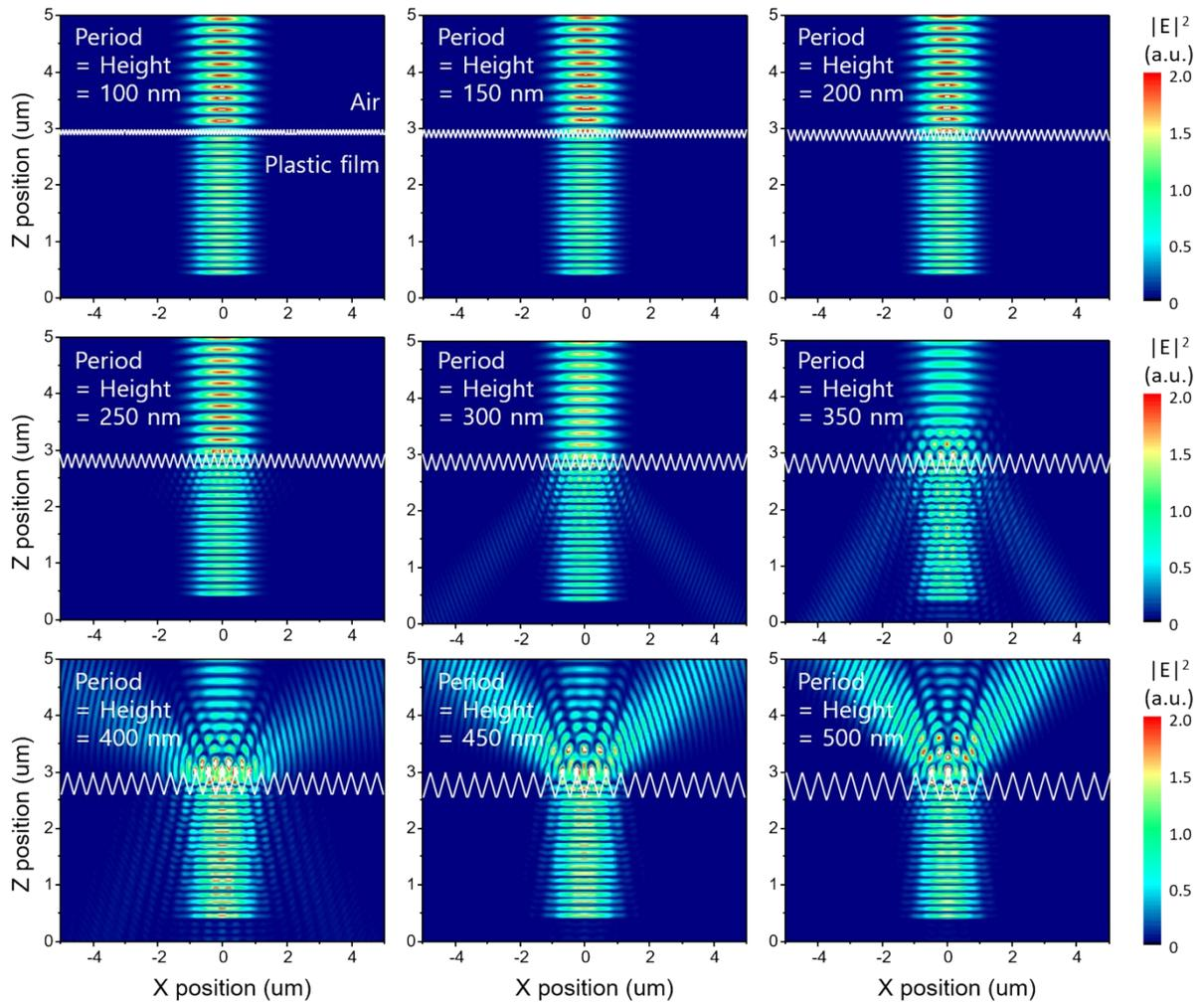
**Fig. S5** Cross-sectional electric field distribution as a function of period of the nanostructure. Height was assumed to same as period.
