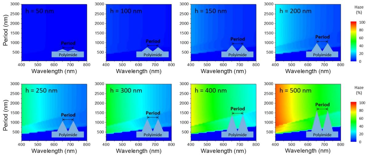
**Fig. S2 (a)** Calculated haze ( $H$ ) of the nanostructured plastic film as functions of period and height of nanostructure. Gap was set to be 0 nm.
