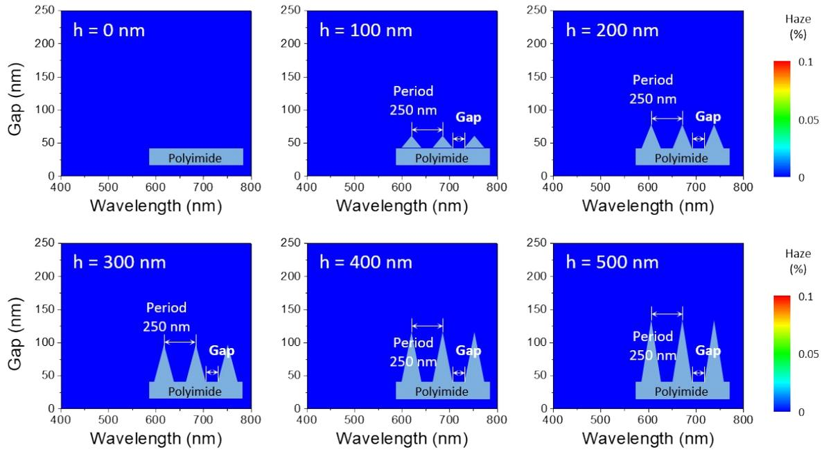
**Fig. S4 (a)** Calculated haze ( $H$ ) of the nanostructured plastic film as functions of gap and height of nanostructure. Period was set to be 250 nm.
