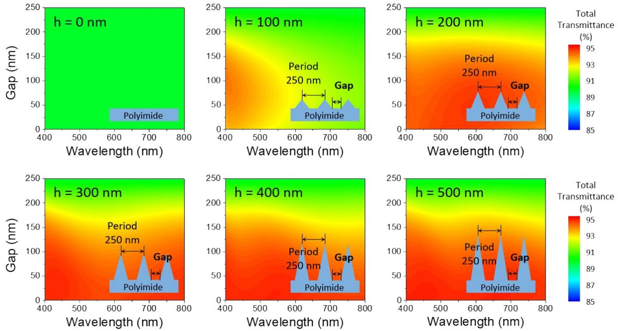
**Fig. S3 (a)** Calculated total transmittance ( $T_{\text{total}}$ ) of the nanostructured plastic film as functions of gap and height of nanostructure. Period was set to be 250 nm.
