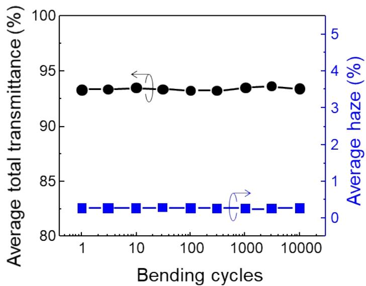
**Fig. S7** Average total transmittance and haze of AgCl nanostructure on PI film as a function of bending cycles with bending radius of 2 nm.
