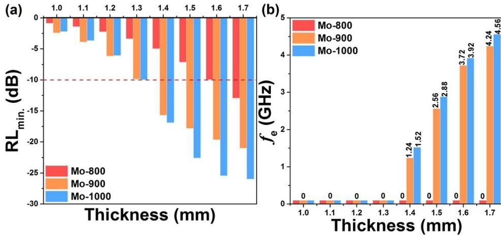
Figure S3. The reflection loss (RL) values of sample-paraffin (20 wt%) nanocomposites with the thickness from 1.0 to 1.7 mm; the effective bandwidth ( $f_e$ ) (<-10 dB) of the samples.
