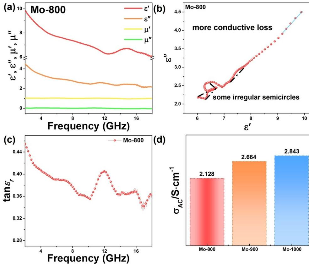
**Figure S6.** Measured frequency dependence of the permittivity and permeability of sample-paraffin (20 wt%) nanocomposites (a); Cole-Cole plots of Mo-800 (b); (c) Frequency dependence of dielectric loss of Mo-800 and Mo-1000 with 20 wt% paraffin nanocomposites; (d) the calculated conductivities of the samples.
