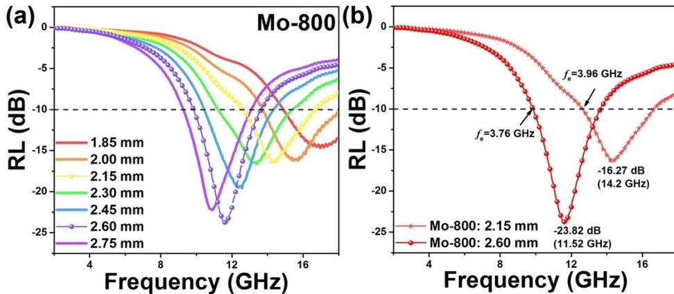
Figure S4. The reflection loss (RL) values of Mo-800 of sample-paraffin (20 wt%) nanocomposites (a); (b) the RL values of Mo-800 with the thickness of 2.15 and 2.60 mm.
