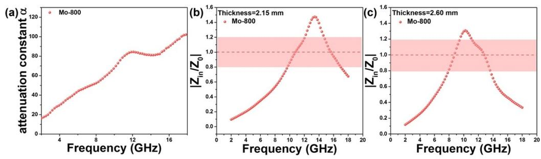
**Figure S7.** Attenuation constant  $\alpha$  of the samples (a); The  $|Z_{in}/Z_0|$  values of Mo-800/paraffin (20 wt%) nanocomposites with thickness of (b) 2.15 mm and (c) 2.60 mm.
