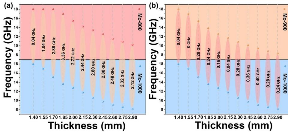
**Figure S5.** The shift of  $RL_{min}$  value with 20 wt% paraffin nanocomposites between Mo-800 and Mo-1000 (a) as well as between Mo-900 and Mo-1000 (b).
