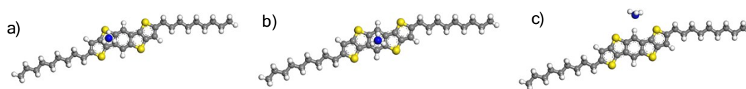
Figure S6. The three absorption configuration of the \text{NH}_3 molecule on the DTBDT- \text{C}_9 molecules.
