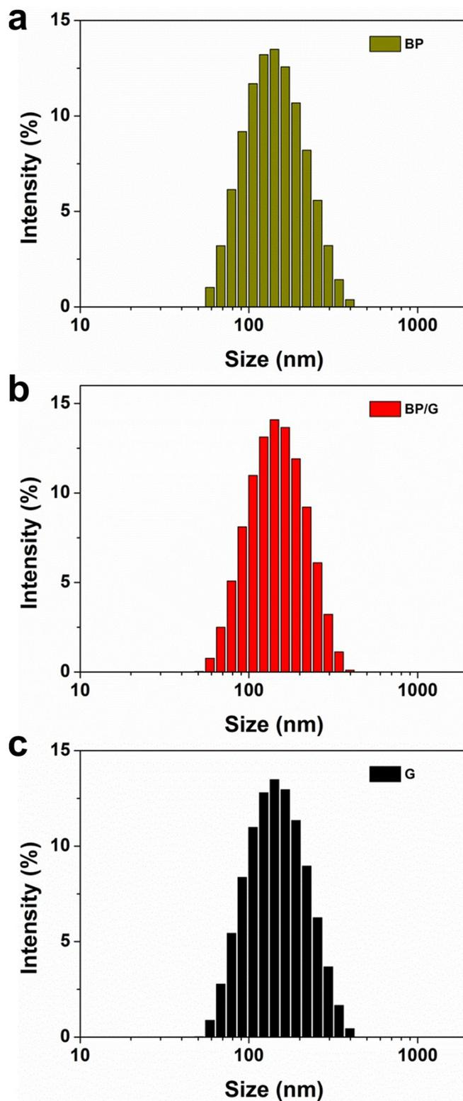
**Figure S1.** Hydrostatic radius distribution measured on zetasizer for (a) exfoliated BP in NMP, (b) co-exfoliated BP/G in NMP, and (c) exfoliated G in NMP.
