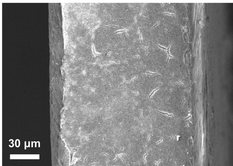
**Figure S4.** SEM cross-sectional view of the as-deposited materials on stainless steel electrode.
