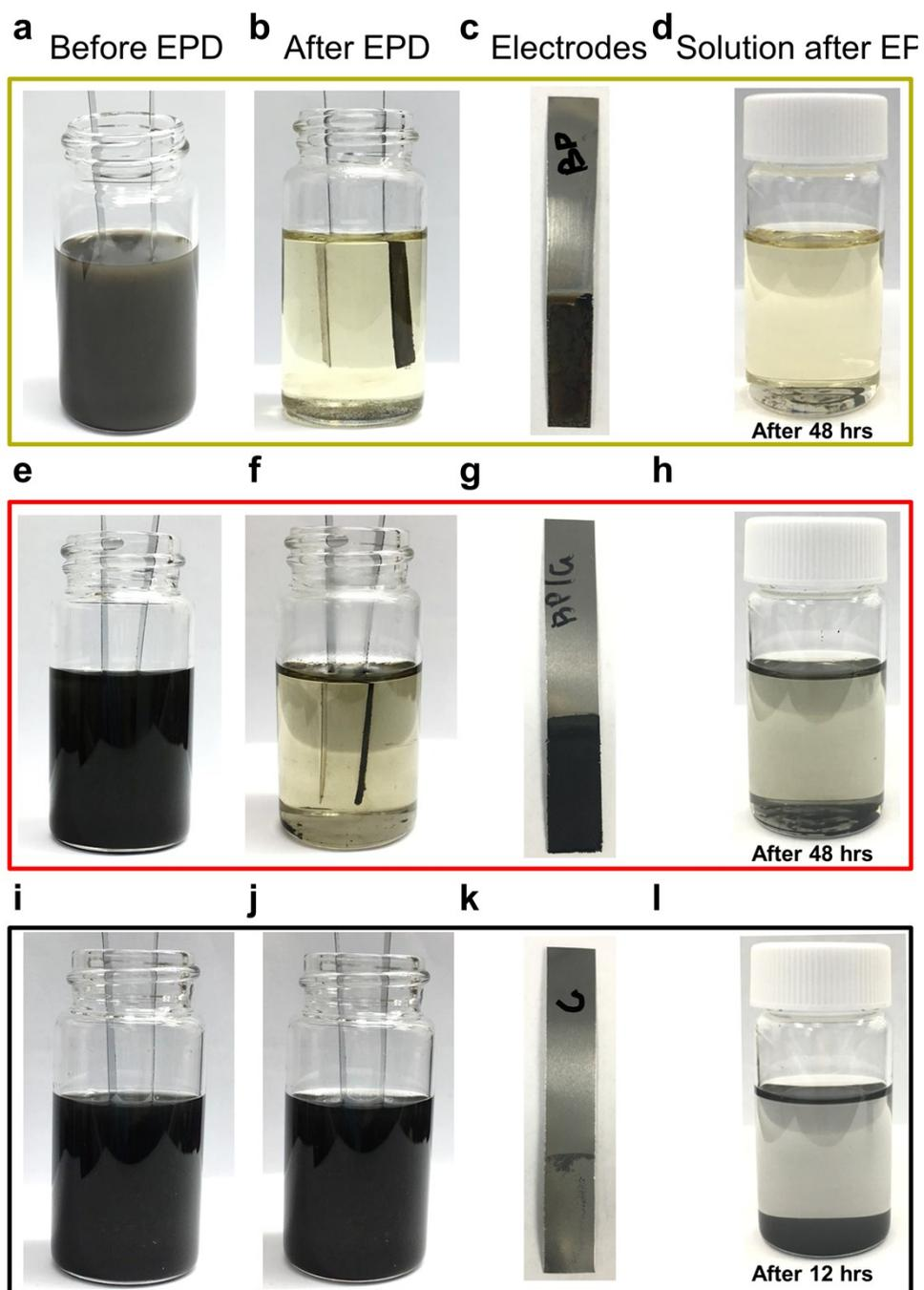
**Figure S2.** Exfoliated solution before and after EPD, the electrode looking and sedimentation tests for (a)-(d) BP in NMP; (e)-(h) BP/G in NMP; and (i)-(l) G in NMP.
