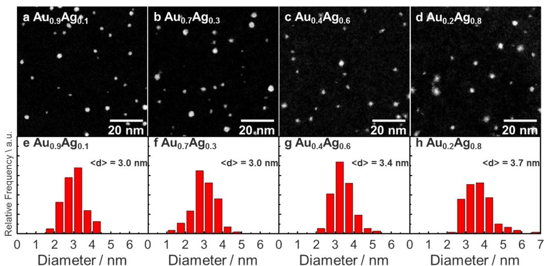
Figure S3. STEM images and histograms of diameter distributions of  $\text{Au}_x\text{Ag}_{1-x}$  BNPs: (a, e)  $\text{Au}_{0.9}\text{Ag}_{0.1}$ ; (b, f)  $\text{Au}_{0.7}\text{Ag}_{0.3}$ ; (c, g)  $\text{Au}_{0.3}\text{Ag}_{0.7}$ ; (d, h)  $\text{Au}_{0.2}\text{Ag}_{0.8}$ .
