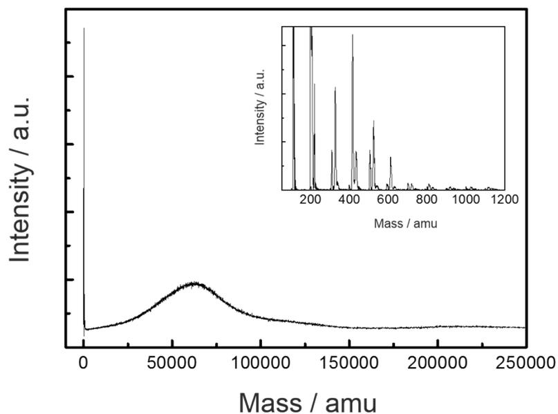
Figure S1. Full RToF mass spectrum of  $\text{Au}_x\text{Ag}_{1-x}$  clusters taken from Au-Ag alloy target 35 at% Au and 65 at% Ag from few atoms region to the main production region.
