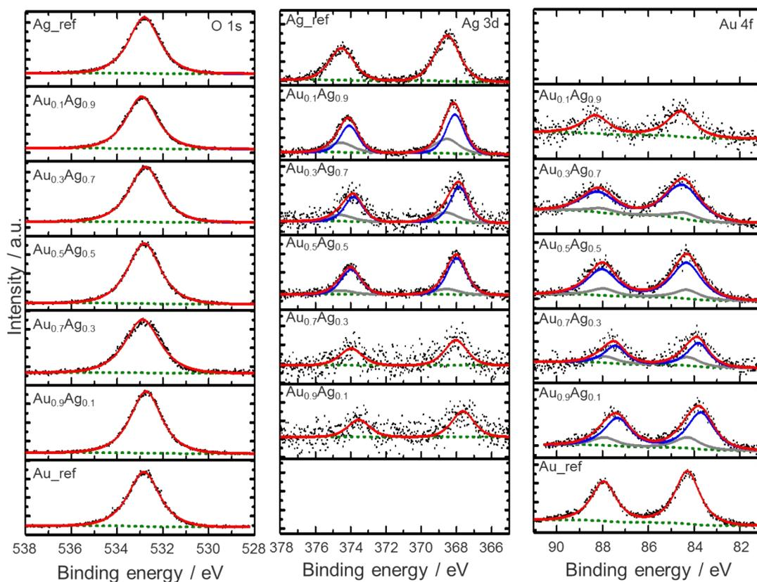
Figure S4. O 1s, Ag 3d and Au 4f XPS spectra of the  $\text{Au}_x\text{Ag}_{1-x}$  BNPs on  $\text{SiO}_2$  wafers from  $x = 0.9$  to  $0.1$ . The green dash lines are the Shirley backgrounds, the blue lines are pure phase of Au and Ag and the grey lines are the Au-Ag alloy phases.
