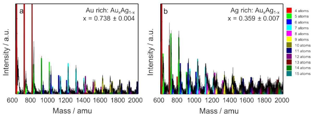
Figure S8. RTof-MS of deposited  $Au_xAg_{1-x}$  clusters, (a) and (b) mass spectra of  $73.8 \pm 0.4$  at% Au and  $26.2 \pm 0.4$  at% Ag as well as  $35.9 \pm 0.7$  at% Au and  $64.1 \pm 0.7$  at% Ag combined with simulation spectra.
