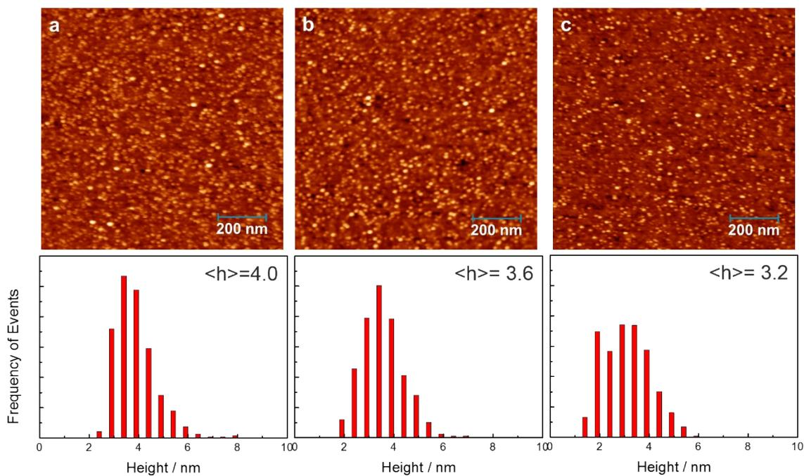
Figure S6. Height histograms of the 0.1 ML Au-Ag BNPs with different composition,  $\text{Au}_{0.9}\text{Ag}_{0.1}$ (a),  $\text{Au}_{0.6}\text{Ag}_{0.4}$ (b),  $\text{Au}_{0.2}\text{Ag}_{0.8}$ (c) deposited on  $\text{SiO}_2$  wafers.
