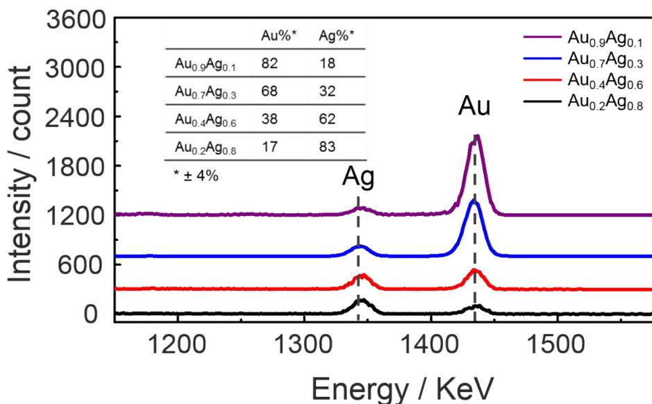
Figure S9. RBS spectra of deposited  $Au_xAg_{1-x}$  BNPs from gold rich to silver rich on  $SiO_2$  wafers. The inset table shows the overall composition of deposited clusters as determined by RBS.
