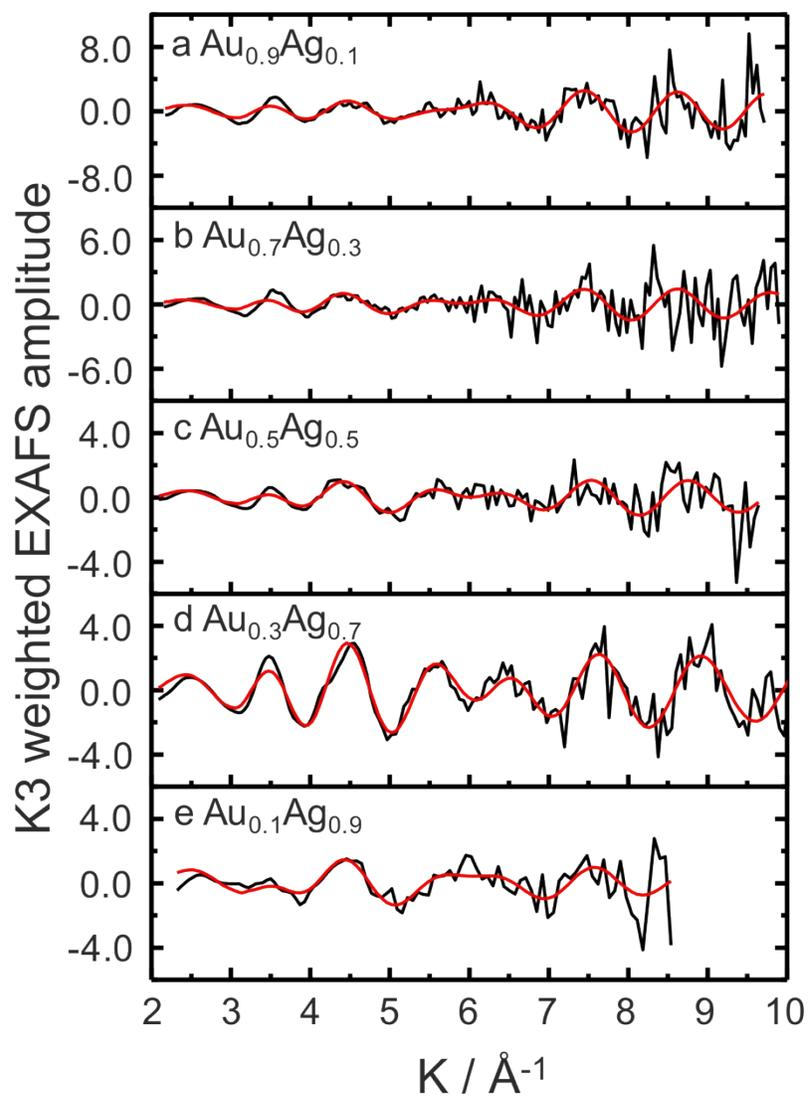
Figure S5.  $k^3$  weighted XAFS spectra of the  $\text{Au}_x\text{Ag}_{1-x}$  BNPs on  $\text{SiO}_2$  wafers from  $x = 0.9$  to  $0.1$ . The corresponding phase-corrected Fourier transformed EXAFS spectra is shown in main text Figure 2a.
