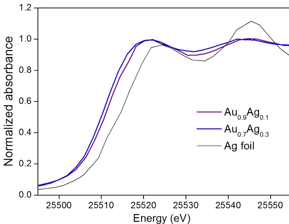
Figure S7. XANES spectra of gold-rich  $\text{Au}_{0.9}\text{Ag}_{0.1}$  and  $\text{Au}_{0.7}\text{Ag}_{0.3}$  BNPs along with Ag foil reference.
