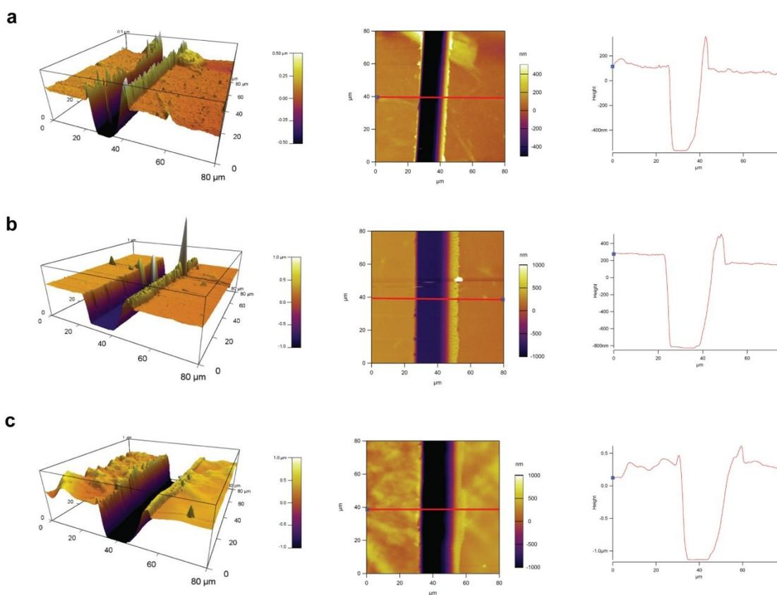
**Figure S11.** 3D images (left), height retraces (middle) and height profiles (right) of **BTBT-peptide** film (a), **C<sub>8</sub>-BTBT-peptide** film (b) and **BTBT-peptide** film with Al contacts (c).
