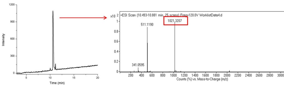
**Figure S3.** Chemical structure of **BTBT-peptide** molecule (top). Liquid chromatogram (left) and mass spectrum (right) of BTBT-Peptide molecule.
