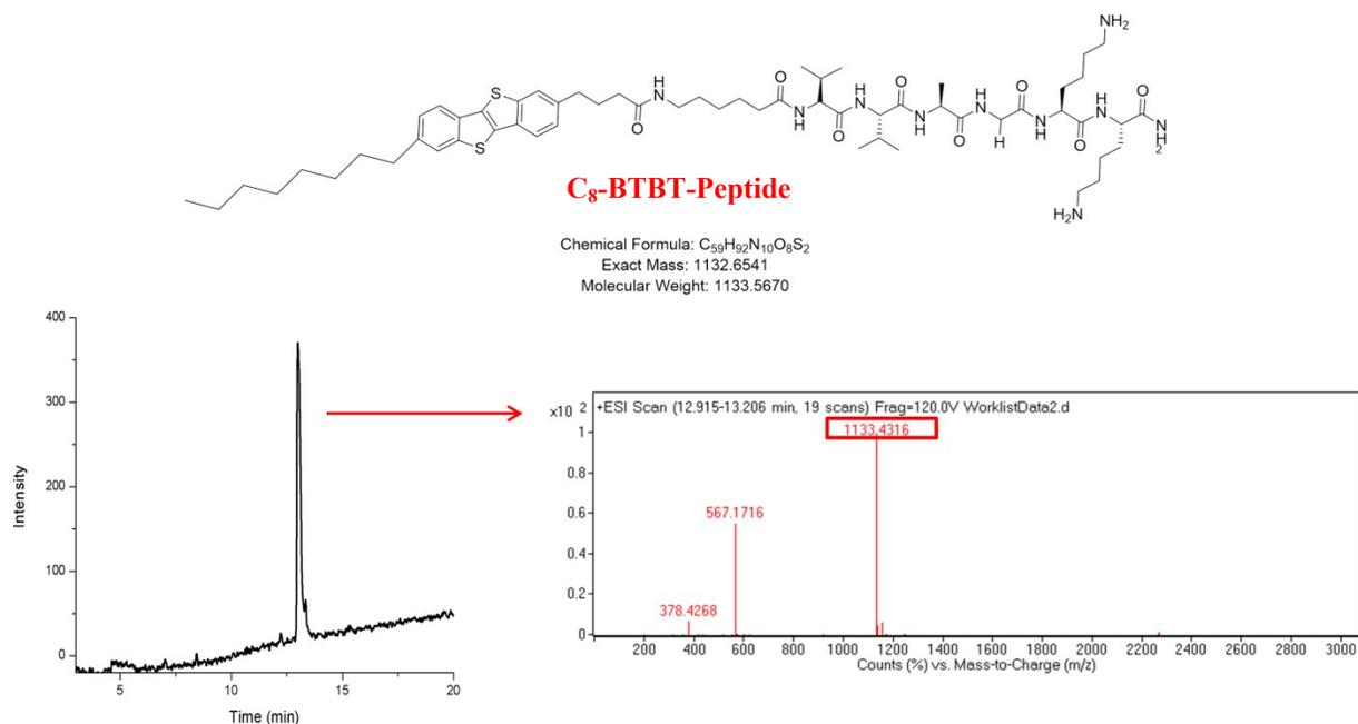
**Figure S4.** Chemical structure of **C<sub>8</sub>-BTBT-peptide** molecule (top). Liquid chromatogram (left) and mass spectrum (right) of **C<sub>8</sub>-BTBT-Peptide** molecule.
