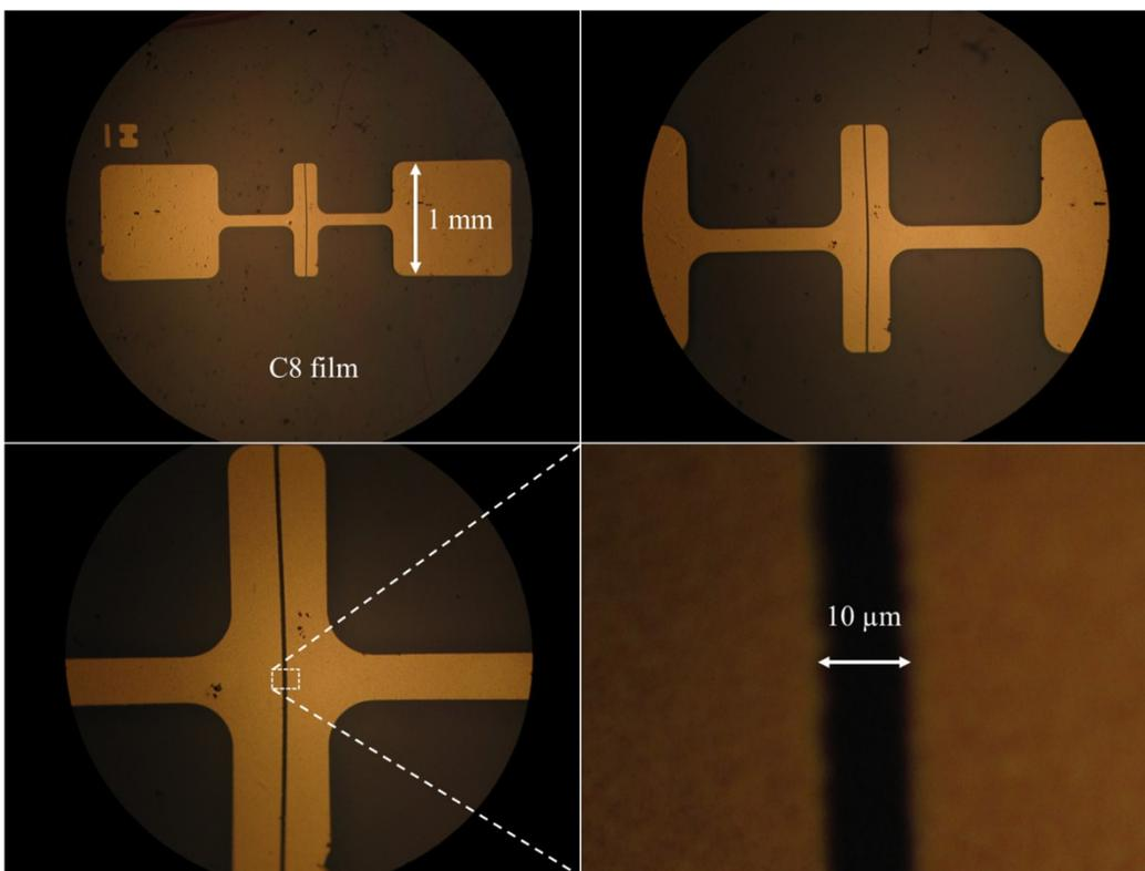
**Figure S8.** Optical microscope images of Au contacts on **C<sub>8</sub>-BTBT-peptide** film with  $L = 10 \mu\text{m}$  and  $W = 1 \text{ mm}$ .
