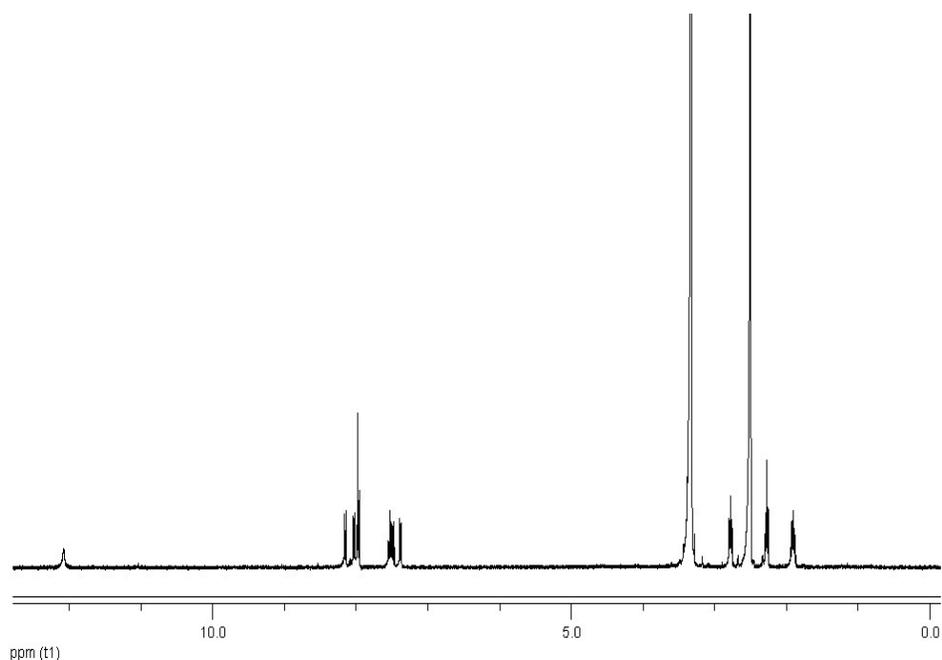
**Figure S1.**  $^1\text{H}$  NMR spectra of **BTBT-C<sub>3</sub>-COOH** in dimethyl sulfoxide-d<sub>6</sub>.
