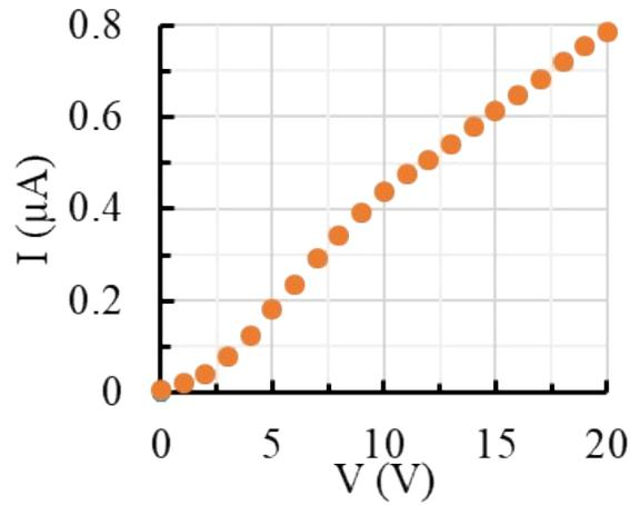
**Figure S12.** I-V characteristics of **BTBT-peptide** film between two Al electrodes.
