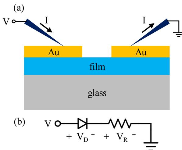
**Figure S9.** (a) Electric bias/current configurations on cross section illustration of a channel separating Au electrodes. (b) Electrical circuit model of the channel.
