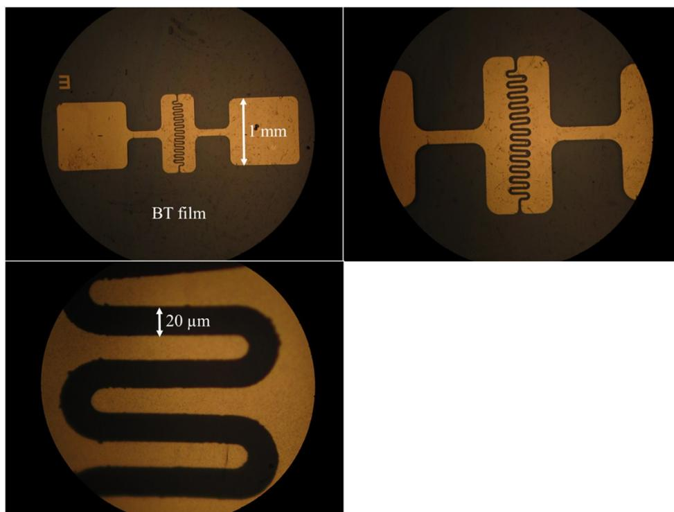
**Figure S7.** Optical microscope images of Au contacts on **BTBT-peptide** film with  $L = 20 \mu\text{m}$  and  $W = 4 \text{ mm}$ .
