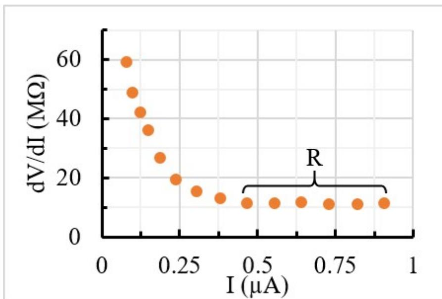
**Figure S10.** Derivative resistance of **BTBT-peptide** film between two Au electrodes.
