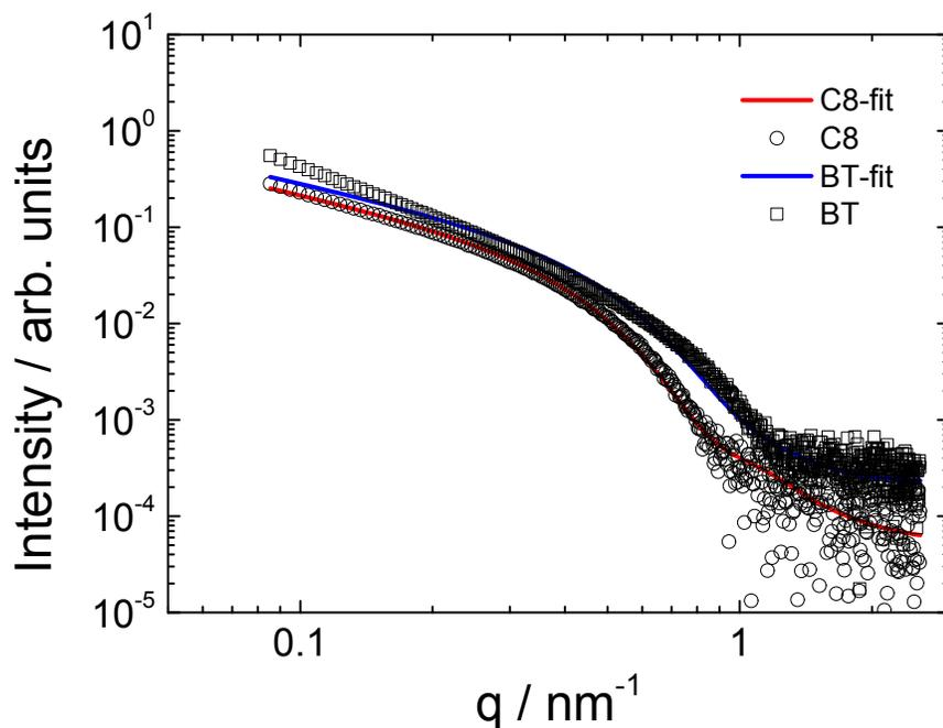
**Figure S5.** SAXS data measured for solutions of **BTBT-peptide** and **C<sub>8</sub>-BTBT-peptide** (open symbols) along with form factor fits (lines) using a core-shell cylinder model (described in the text).
