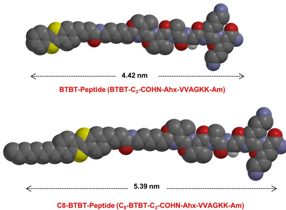
**Figure S6.** Computed (DFT, B3LYP/6-31G\*\*) molecular lengths of **BTBT-peptide** and **C<sub>8</sub>-BTBT-peptide** in their fully extended molecular conformations.
