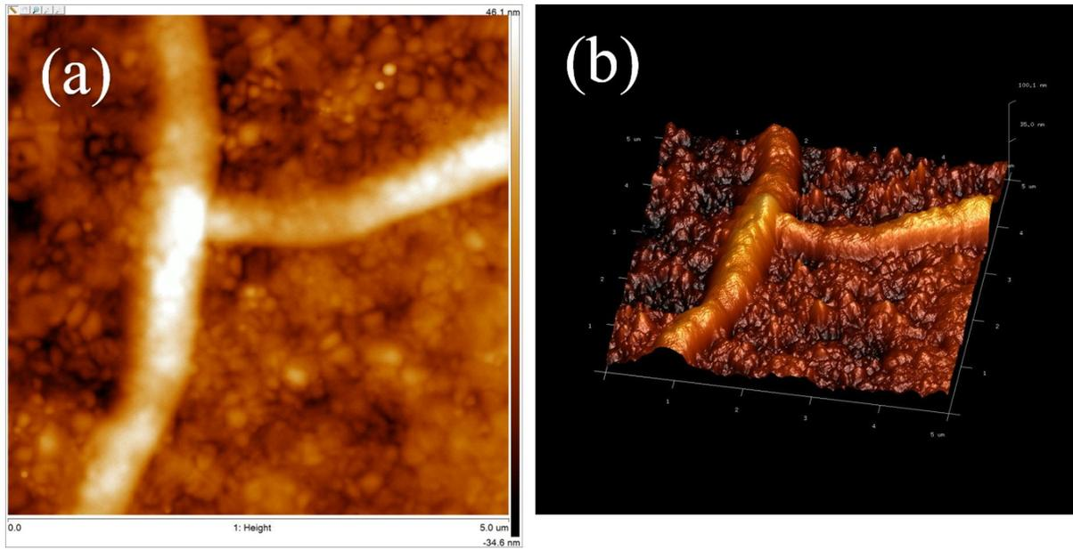
**Figure S7** (a) 2D-AFM height image and (b) 3D-AFM morphology image of the morphology of spray coated PCBM film on the top of perovskite, which clearly shows the PCBM coffee ring.
