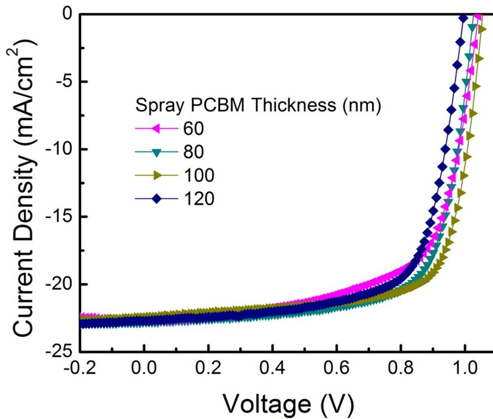
Figure S3  $J$ - $V$  curve of the device with different thickness of spray coated PCBM ETL
