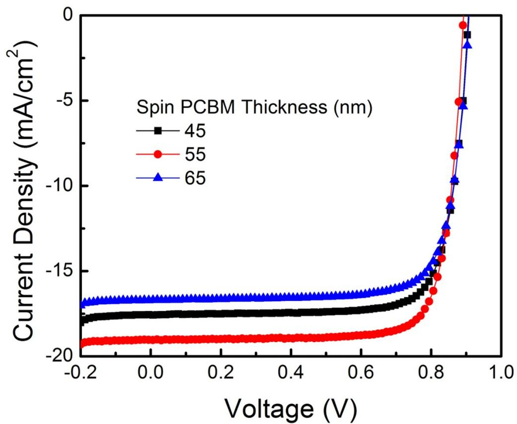
Figure S2 Characteristic  $J-V$  curve of the device with different thickness of spin coated PCBM ETL.
