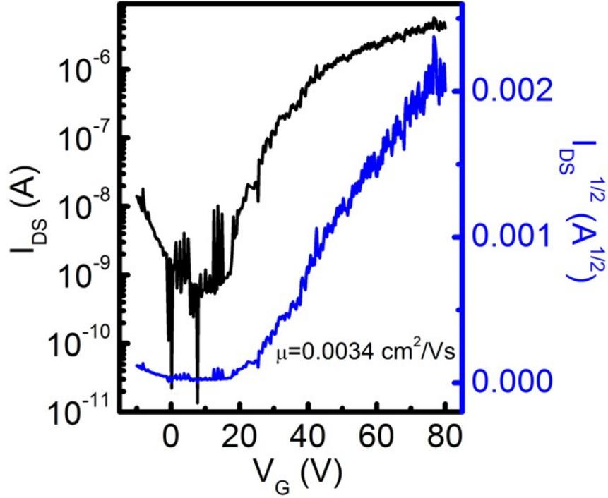
**Figure S8** Transfer characteristics of PCBM (spray coated) transistor operating in the n-channel regime at different gate voltages.
