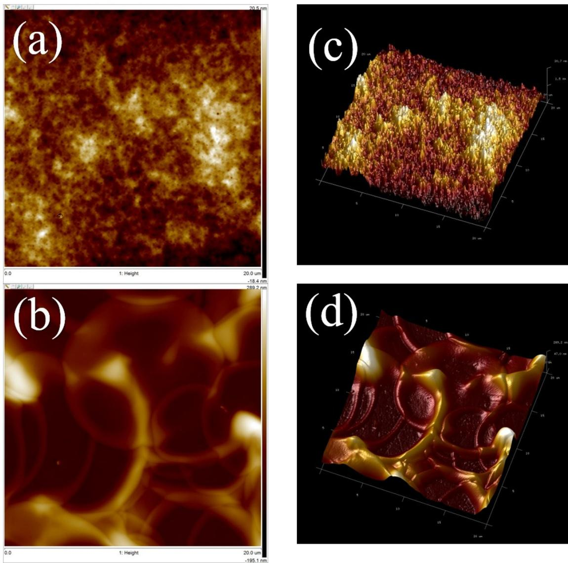
**Figure S5** 2D-AFM height image of (a) spin coated and (b) spray coated PCBM film on the top of glass. (c) and (d) are the 3D-AFM morphology image of (c) spin coated and (d) spray coated PCBM film, which is related to (a) and (b), respectively.
