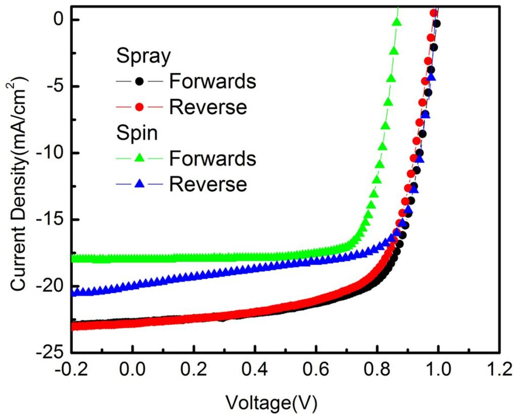
**Figure S4** Comparison of  $J$ - $V$  curves of best cell with spin and spray coated PCBM ETL measured by forward and reverse scans.
