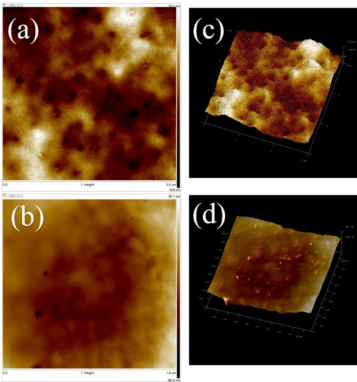
**Figure S6** 2D-AFM height image of (a) spin coated and (b) spray coated PCBM film on the top of perovskite film. (c) and (d) are the 3D-AFM image of (c) spin coated and (d) spray coated PCBM film, which is related to (a) and (b), respectively.
