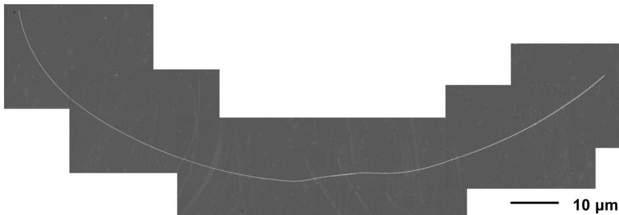
**Fig. S1.** SEM image of a single Ag NW longer than 100  $\mu\text{m}$ .
