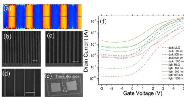
Fig.S3 (a) Top-view of simulated electric field distribution of GNR on SiO<sub>2</sub> substrate. SEM images of the origin GNR with different gaps :100 nm (b), 500 nm (c) and 900 nm (d). (e) SEM image of this phototransistor. (f) Transfer characteristic curves for vertical phototransistors under dark and 512 nm incident lights with different gaps.
