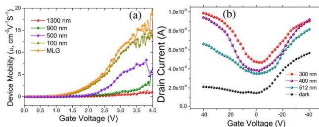
Fig. S6 (a) Device's field effect mobility of phototransistors with different GNR gaps. (b) linear transfer characteristic curves for P-type planar phototransistor ( $V_{DS}=0.6$  V) with different incident light wavelengths.
