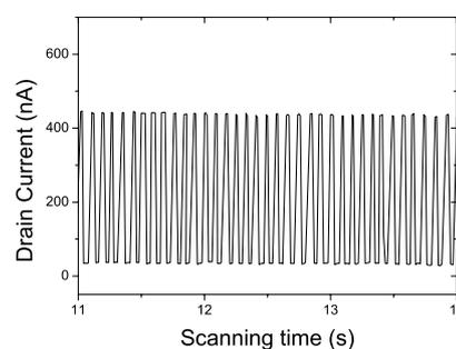
Fig. S7 Time-duration on/off measurement for vertical phototransistor with an ultrafast light signal (512 nm, 0.1 mW/cm<sup>2</sup> mean power density).
