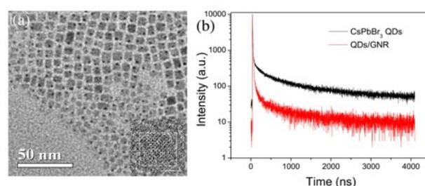
Fig.S2 (a) TEM image of overall CsPbBr<sub>3</sub> QDs in solution and detailed morphology of single QDs. (b) Time resolved Photoluminescence of QDs and QDs/GNR hybrids excited by 512 nm laser under room-temperature.
