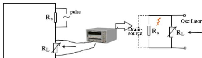
Fig. S8 The schematic for measuring the dynamic pulse signal and connecting method with the series variable resistance box (left). And the estimating method to obtain equivalent resistance by transformation of Thevenin law.
