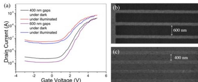
Fig.S4 (a) Transfer character curves of GNR/QDs/IGZO transistor with 400 nm and 600 nm gaps under dark and 512 nm light's illumination. (b)SEM image of GNR film with 600 nm gaps. (c) SEM image of GNR film with 400 nm gaps.
