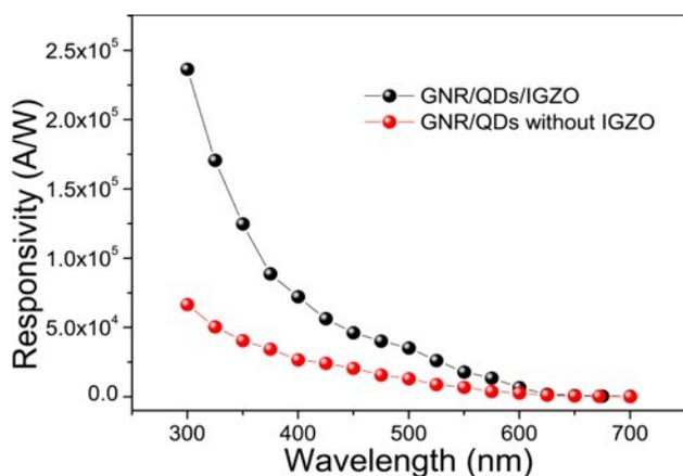
Fig.S5 Responsivity of GNR/QDs/IGZO and GNR/QDs phototransistors versus different wavelengths.
