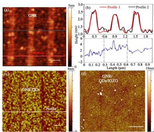
Fig.S1 (a) AFM image of GNR surface morphology (scale bar: 300 nm). (b) The height information of profile 1 and 2 in GNR surface and profile of GNR/QDs hybrids. (c) AFM image of GNR/QDs hybrids' surface morphology. (d) AFM image on top of GNR/QDs/IGZO surface to illustrate roughness of this film.
