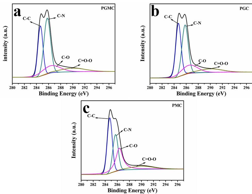
**Fig. S5.** The C 1s XPS spectra of PGMC, PGC and PMC.
