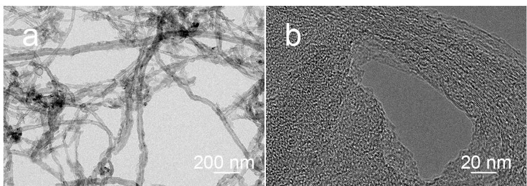
**Fig. S2.** The TEM images of acid treated MWNTs.
