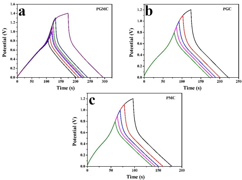
**Fig. S6.** Charge/discharge curves of the PGMC, PGC and PMC composite electrodes
