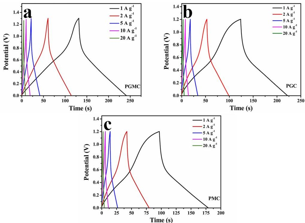
**Fig. S7.** Charge/discharge curves of composite at different current density: (a) PGMC, (b) PGC and (c) PMC in two-electrode system.
