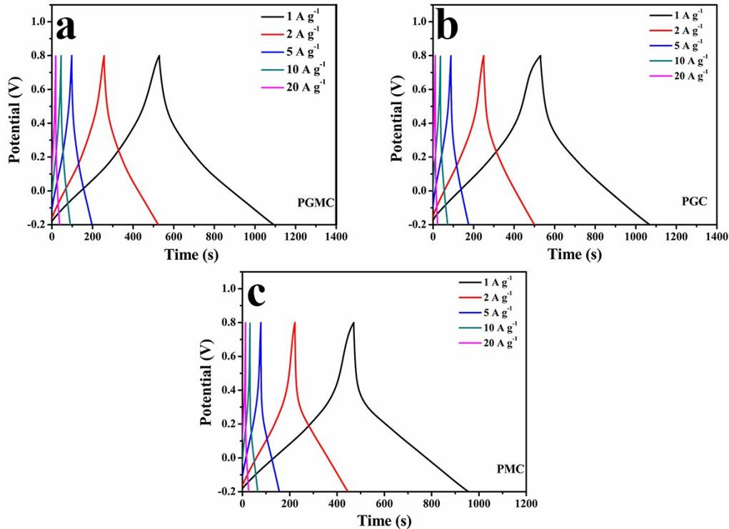
**Fig. S8.** Charge/discharge curves of composite at different current density: (a) PGMC, (b) PGC and (c) PMC in three-electrode system.
