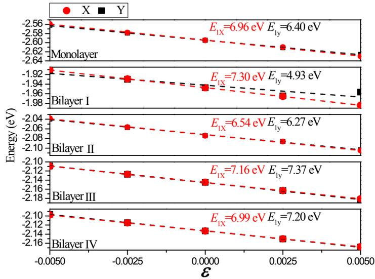
**Figure s4.** Energy shift of CBM for monolayer or bilayer GeAsSe with respect to the lattice dilation and compression along the X and Y directions, respectively.
