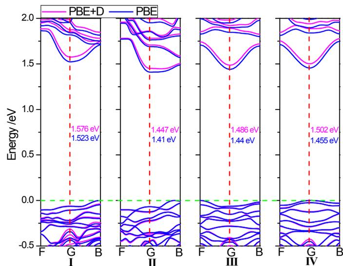
**Figure s6.** The band structure of bilayer GeAsSe calculated with PBE (blue lines) and PBE+D (magenta lines) method.
