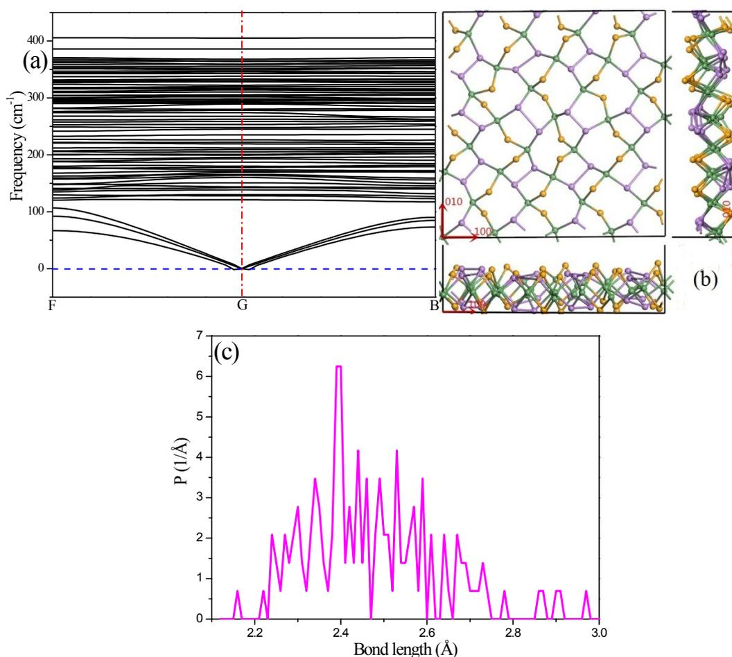
**Figure s1.** (a) The phonon dispersion curves of monolayer GeAsSe. (b) Top and side views of an
