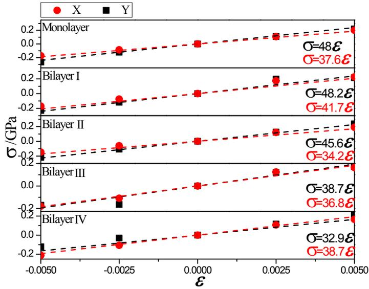
**Figure s3.** Axial stresses of monolayer or bilayer GeAsSe with respect to the uniaxial stretching and compression along the x (100) or y (010) directions. Dash lines represent the linear fitted results.
