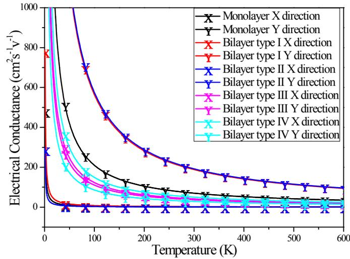
**Figure s5.** The electrical mobility of monolayer and bilayer GeAsSe considering temperature effects.
