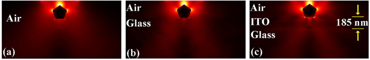
**Fig. S10** 3D simulation of electric-field distribution of AgNWs in air (a), located on glass substrate without (b) or with a layer of ITO seen from the cross-sectional view.
