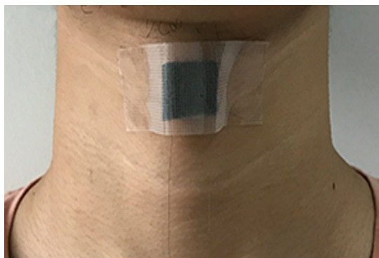
Figure S13. Photo showing how the pressure sensor can be used for sound sensing.
