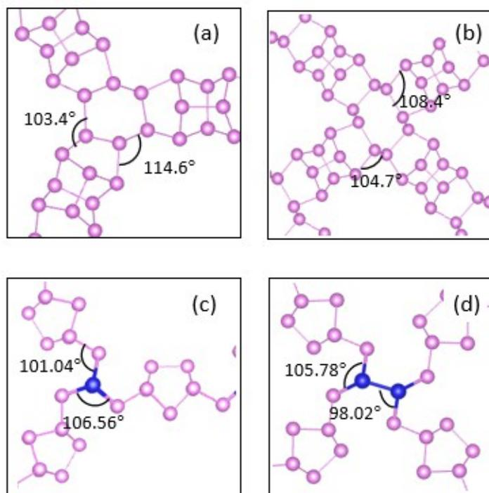
**Figure S2.** Bonding angles between  $P_{12}$  building blocks for (a) P-Hex, (b) P-Monoclinic, (c) V-Hex, and (d) V-Tetr, The bridge P atoms and P dimers are highlighted in blue.
