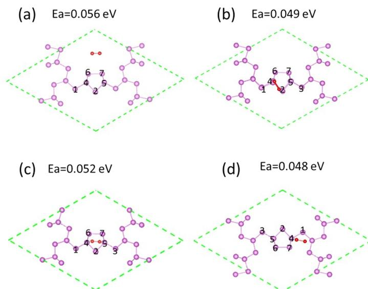
Figure. S3. Top view of the examined possible adsorption configurations of  $O_2$  molecule adsorbed on allotrope of V-Hex.  $E_a$  denotes the adsorption energy per  $O_2$  molecule. P and O atoms are colored in pink and red, respectively.
