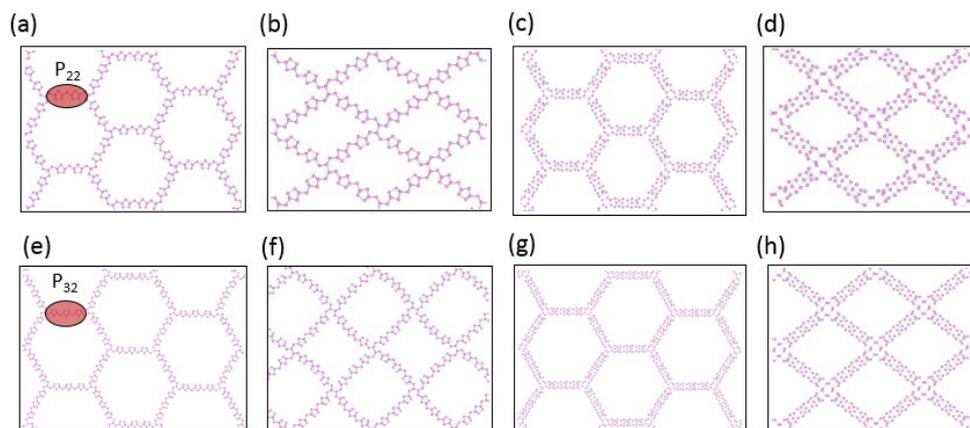
**Figure S5.** Geometric structures of V-Hex, V-Tetr, P-Hex, and P-Monoclinic formed with the  $P_{22}$  and  $P_{32}$  building blocks, respectively.
