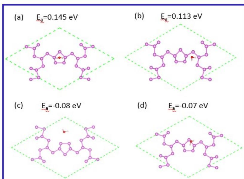
**Figure S6.** Top view of the examined possible adsorption configurations of  $H_2O$  molecule adsorbed on allotrope of V-Hex.  $E_a$  denotes the adsorption energy per  $H_2O$  molecule.
