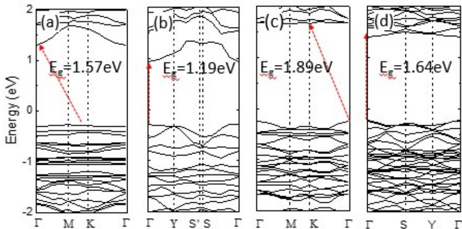
**Figure S4.** Band structures of the 2D clathrate phosphorenes obtained within the PBE scheme for (a) P-Hex, (b) P-Monoclinic, (c) V-Hex, and (d) V-Tetr, all based on the  $P_{12}$  building blocks.
