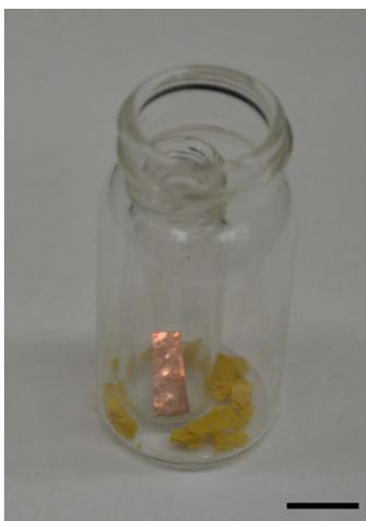
**Fig. S1** Photo of the reaction setup before sealing and injection of dilute  $\text{H}_2\text{SO}_4$  solution. The double vials ensure that the graphene sample is only exposed to  $\text{H}_2\text{S}$  gas which is generated in situ, not any liquids or solids. Scale bar: 1 cm.
