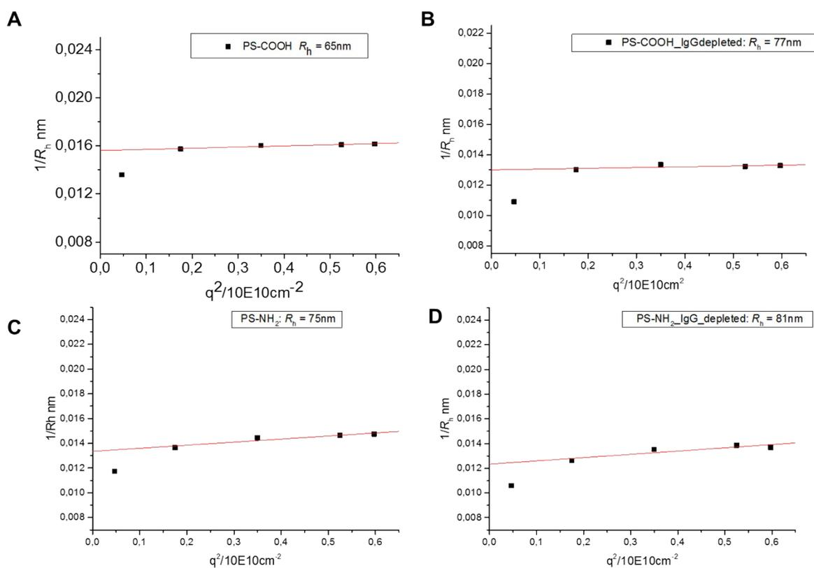
**Figure S 2.** Multi-angle dynamic light scattering (DLS) analysis. Angular dependency of the hydrodynamic radius  $R_h$  for uncoated (A, C) and pre-coated (B, D) nanoparticles. PS-COOH are shown in (A, B) and PS-NH<sub>2</sub> in (C, D).
