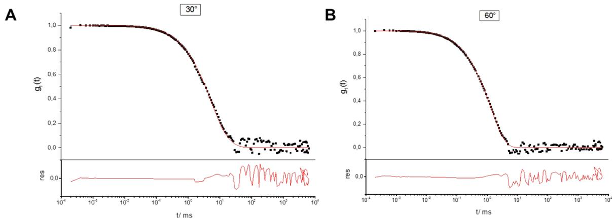
**Figure S 7.** Multi-angle dynamic light scattering analysis: *Upper graph:* Autocorrelation function  $g_1(t)$  (black dots) of pre-coated PS-COOH nanoparticles incubated with human plasma at a scattering angle  $\theta = 30^\circ$  (A) or  $\theta = 60^\circ$  (B). The red line (–) represents the forced fit. There is no additional aggregation term needed indicating that the pre-coated nanoparticles remain stable in human plasma.
