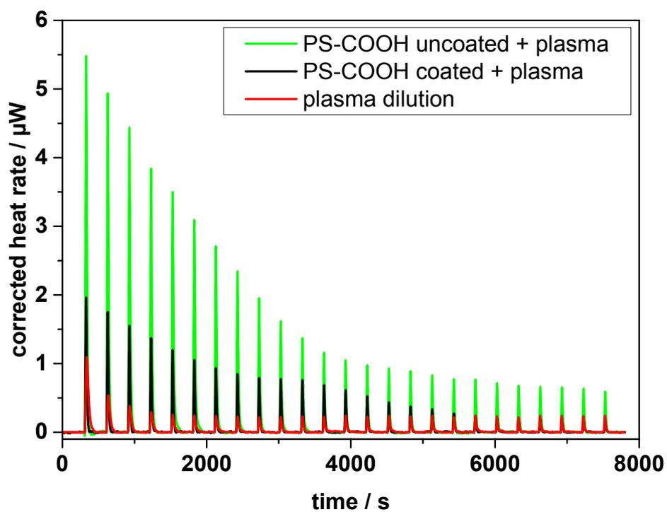
**Figure S 5.** Corrected heat rates of isothermal titration calorimetry experiments (ITC) experiments. The plasma dilution describes the titration of plasma into water and was subtracted from the adsorption measurements after integration.
