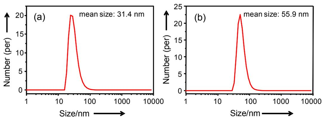
**Fig. S3** DLS measurements of the CoOOH nanoflakes (a) and the RCDs-CoOOH hybrid (b) in DI water.
