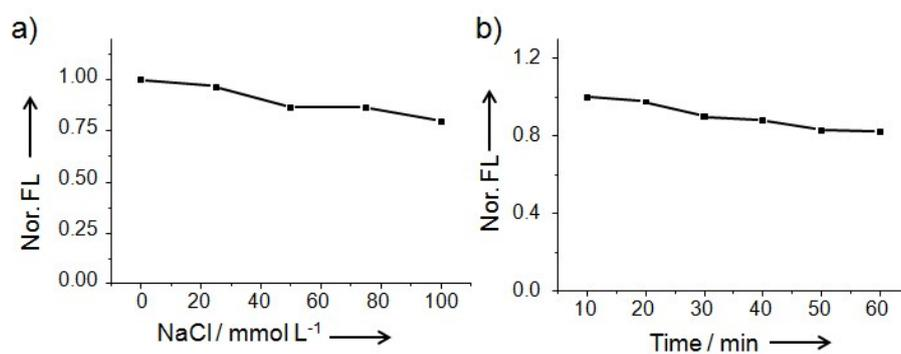
**Fig. S2** a) The relative fluorescence emission intensity of the RCDs at 640 nm (excitation at 550 nm) under the various ionic strengths (NaCl). b) Photostability of the RCDs (emission at 640 nm) under continuous irradiation with a xenon lamp (150 W).
