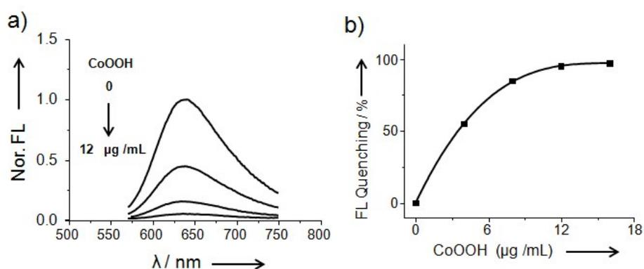
Fig. S6 a) Fluorescence quenching of RCDs (5 µg/mL) in the presence of different amounts of CoOOH. b) Fitting curve between fluorescence quenching efficiency and the concentration of CoOOH.
