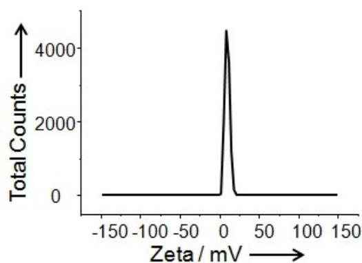
**Fig. S4** Surface Zeta potential of CoOOH nanoflakes in water.
