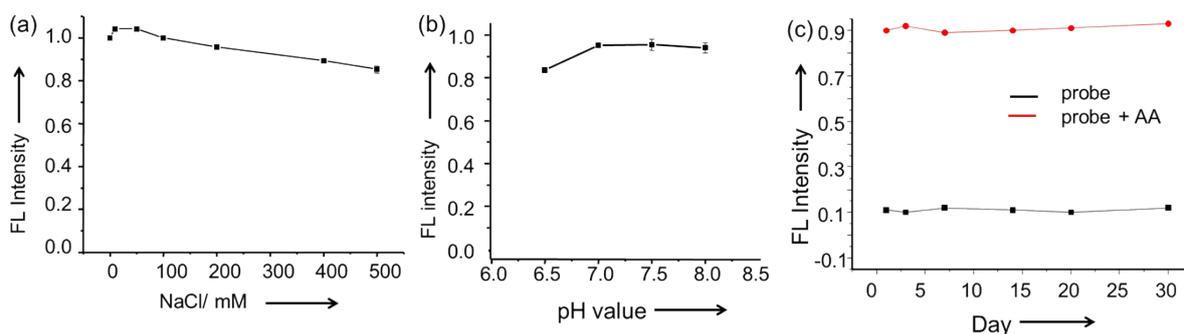
Fig. S7 a) Relative fluorescence emission intensity of the RCDs-CoOOH at 640 nm (excitation at 550 nm) under the various ionic strengths (NaCl) and physiological pH value from 6.5 to 8.0 (b). c) long term storage ability of the probe (17 µg/mL) in the absence (black line) and presence of 60 µM AA (red line).
