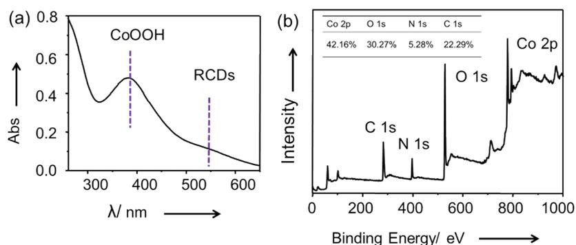
Fig. S5 a) UV-Vis absorption spectrum of the probe (i.e., RCDs-CoOOH); b) XPS characterization of the RCDs-CoOOH hybrid (inset: mass percentage of the elements Co, O, N and C).
