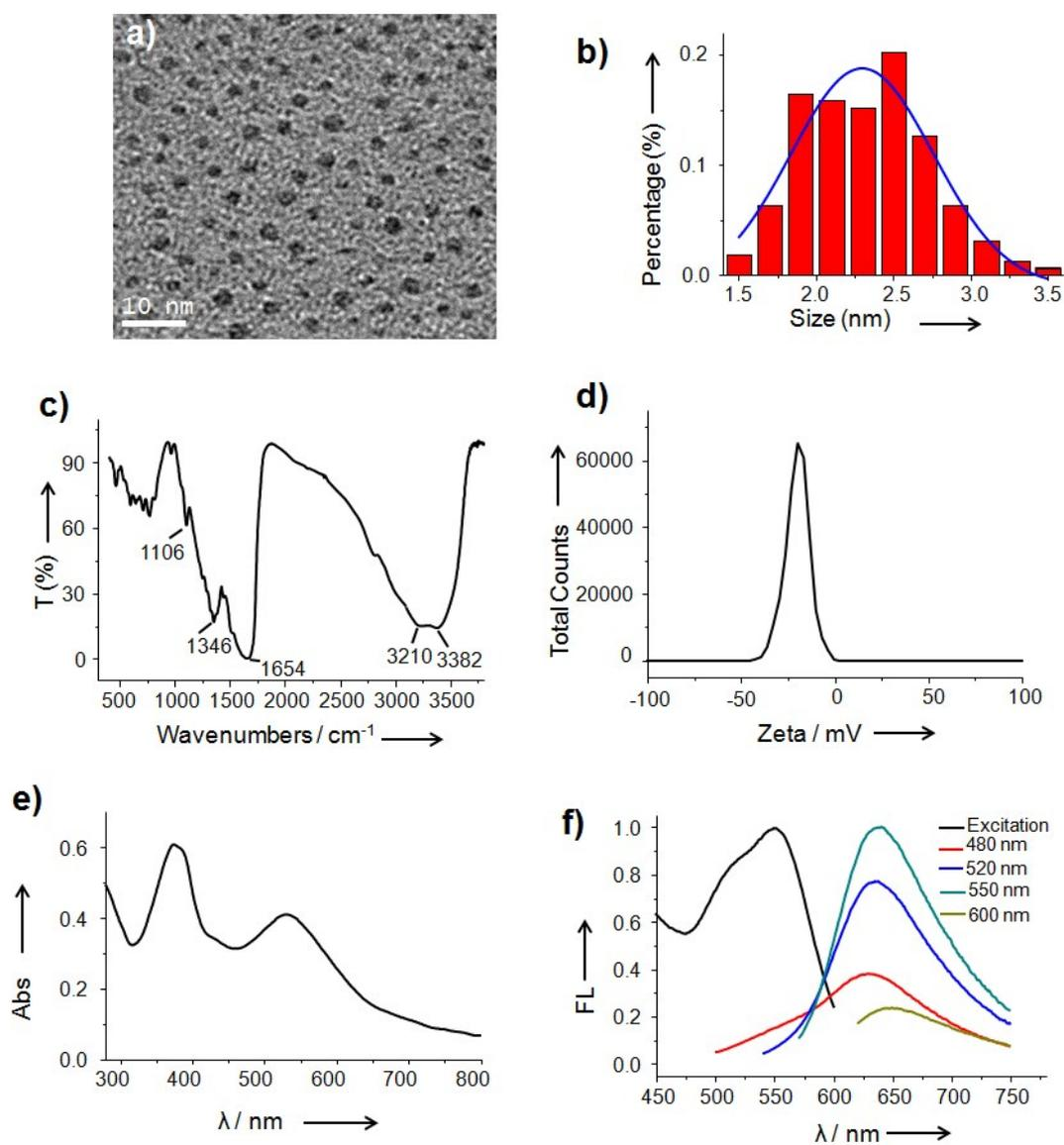
**Fig. S1** a, b) TEM image of the RCDs (a) and corresponding size distribution of TEM (b). c) FT-IR spectrum of the RCDs. d) Zeta potential of the RCDs in water. e) UV-Vis absorption spectrum of the RCDs. f) Fluorescence excitation spectrum and fluorescence emission spectra under different excitation wavelengths of RCDs, respectively.
