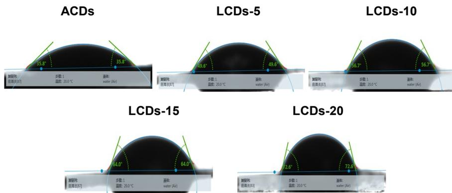
**Figure S2.** The contact angles of ACDs, LCDs-5, LCDs-10, LCDs-15, LCDs-20.
