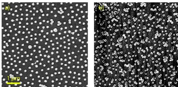
**Figure S1.** SEM images of a quasi-random array of the layered Au-Pd nanodisks on (a) the parent substrate before annealing and transfer and (b) after the transfer process to a fiber.
