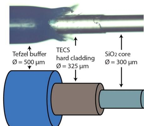
**Figure S2.** Optical micrograph of the optical fiber used (top) and a corresponding schematic illustration (bottom) showing the core, the cladding and the buffer coating with their respective diameters. The removal of the fiber coating and cladding is described in the Methods section in the main text. The schematic is not drawn to scale.
