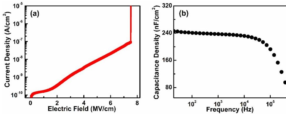
**Fig. S7** (a) leakage current density and (b) areal capacitance of  $\text{ZrO}_x$  dielectric.
