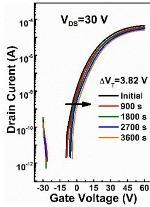
**Fig. S5** Transfer curves of  $\text{Zn}_{0.3}\text{Sn}_{0.7}\text{O}$  NFNs/ $\text{SiO}_2$  FETs under PBS tests for 3600 s.
