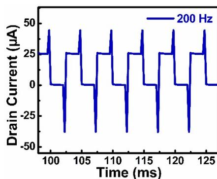
**Fig. S8** Drain current responses to a square wave signal applied to the gate voltage with 200 Hz frequency.
