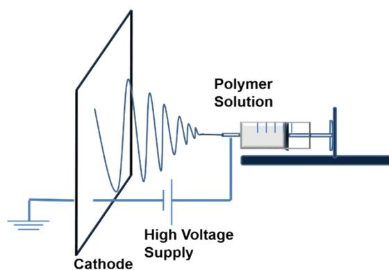
**Fig. S1** Schematic of electrospinning process.
