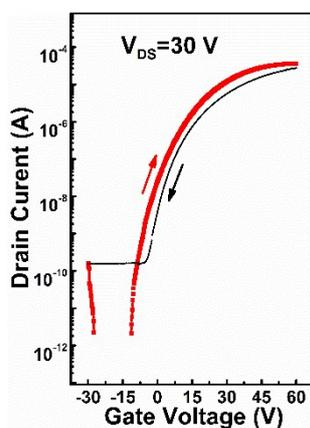
**Fig. S4** Transfer curves of the electrospun  $\text{Zn}_{0.3}\text{Sn}_{0.7}\text{O}$  NFNs/ $\text{SiO}_2$  FETs measured with forward and reverse sweep.
