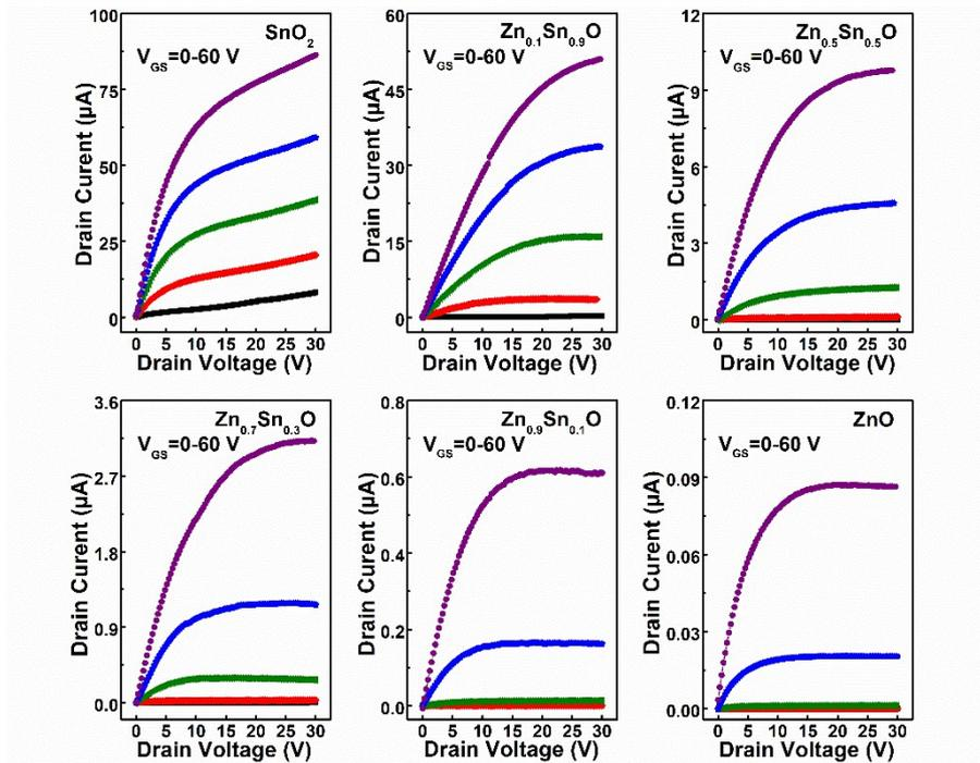
**Fig. S6** Output characteristics of the FETs based on  $\text{Zn}_x\text{Sn}_{1-x}\text{O}$  NFNs with various Zn to Sn molar ratios on  $\text{SiO}_2$  dielectric.
