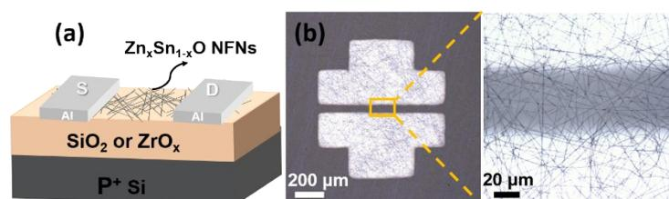
**Fig. S2** (a) Schematic diagram of FETs used in this study. (b) Typical optical microscopy image of the FETs based on  $\text{Zn}_{0.3}\text{Sn}_{0.7}\text{O}$  NFNs and inset of the relative channel amplification diagram of the selected area marked with an orange rectangle in (b).
