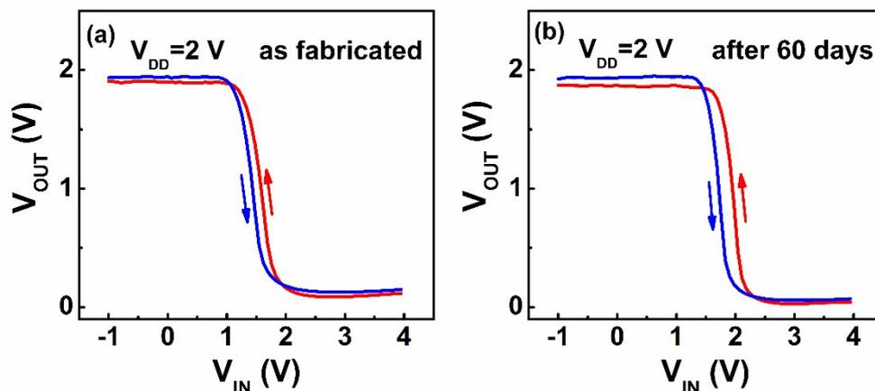
**Fig. S9** VTC curves of inverter based on  $Zn_{0.3}Sn_{0.7}O$  NFNs/ $ZrO_x$  FETs, with forward and reverse sweep, measured immediately after fabrication (a) and measured 60 days later (b).
