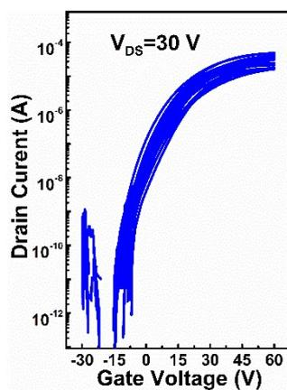
**Fig. S3** Transfer curves of the electrospun  $\text{Zn}_{0.3}\text{Sn}_{0.7}\text{O}$  NFNs/ $\text{SiO}_2$  FETs ( $3 \times 5$  array) at  $V_{DS} = 30$  V.
