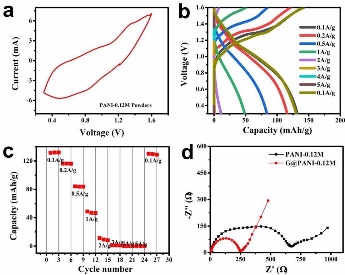
**Figure S4.** For Zinc-ion battery with conventional PANI cathode: (a) CV curves of PANI at the scan rate of 1 mV/s. (b) Voltage profiles curves at the different current densities. (c) Discharge capacity of different current. (d) EIS plots of pure PANI cathode and 3D graphene hydrogel film cathode based Zn-ions hybrid cells.
