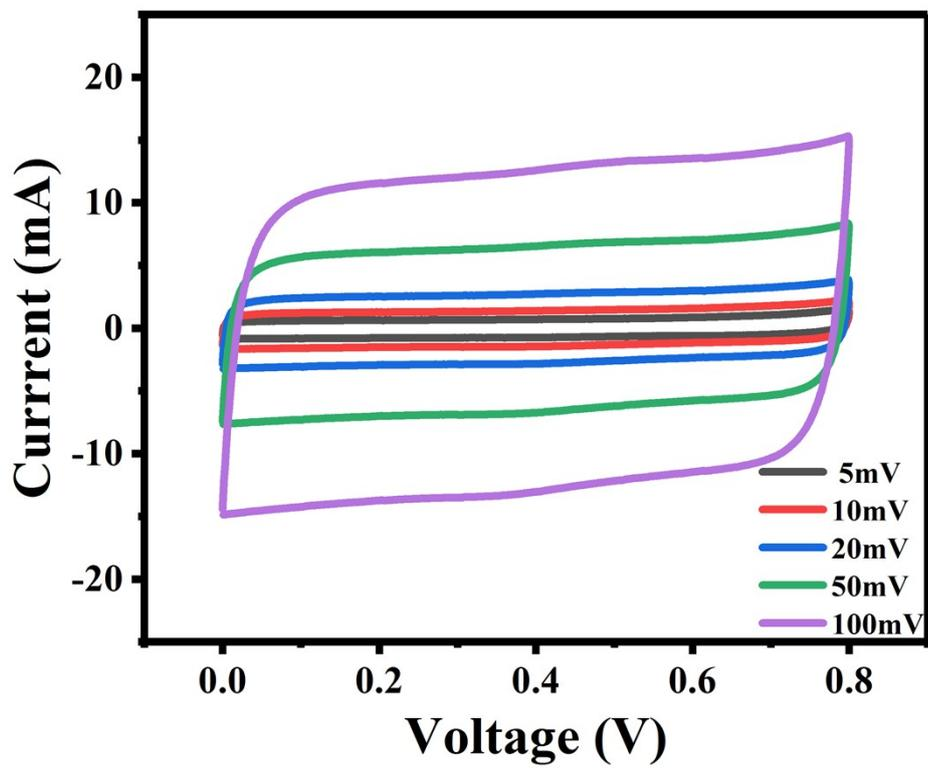
**Figure S3.** The CV curves of 3D graphene hydrogel film electrodes based supercapacitor
