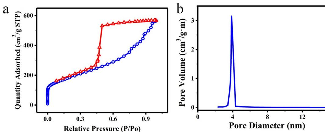
**Figure S2.** N<sub>2</sub> adsorption/desorption measurements: (a) N<sub>2</sub> adsorption-desorption isotherm of the freeze-dried composite hydrogel exhibits a type IV curve with a H4 hysteresis loop. (b) Pores size distribution indicates the composite hydrogel includes large amount of mesopores.
