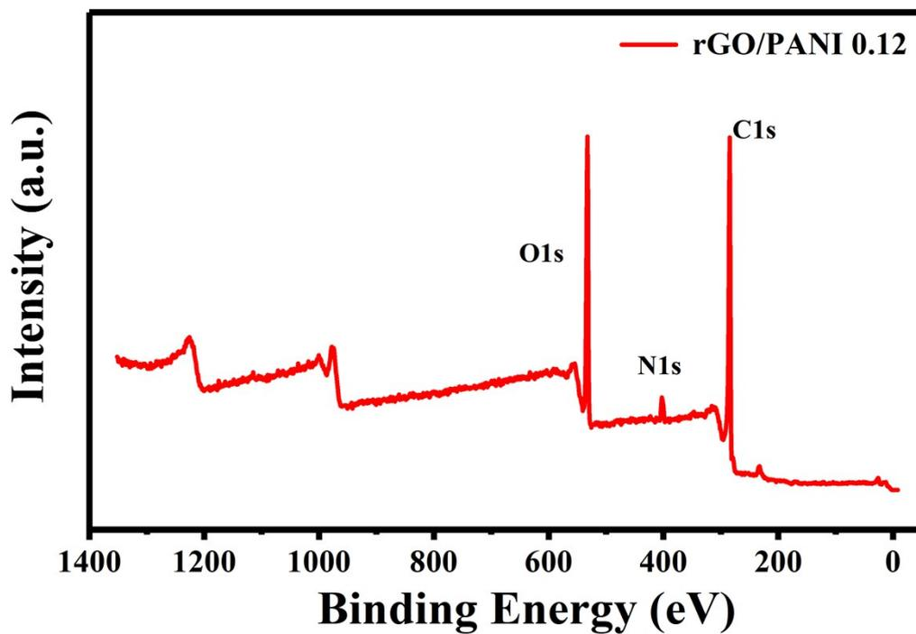
**Figure S1.** The XPS survey spectrum of Freeze-dried 3D graphene@PANI-0.12M hydrogel.
