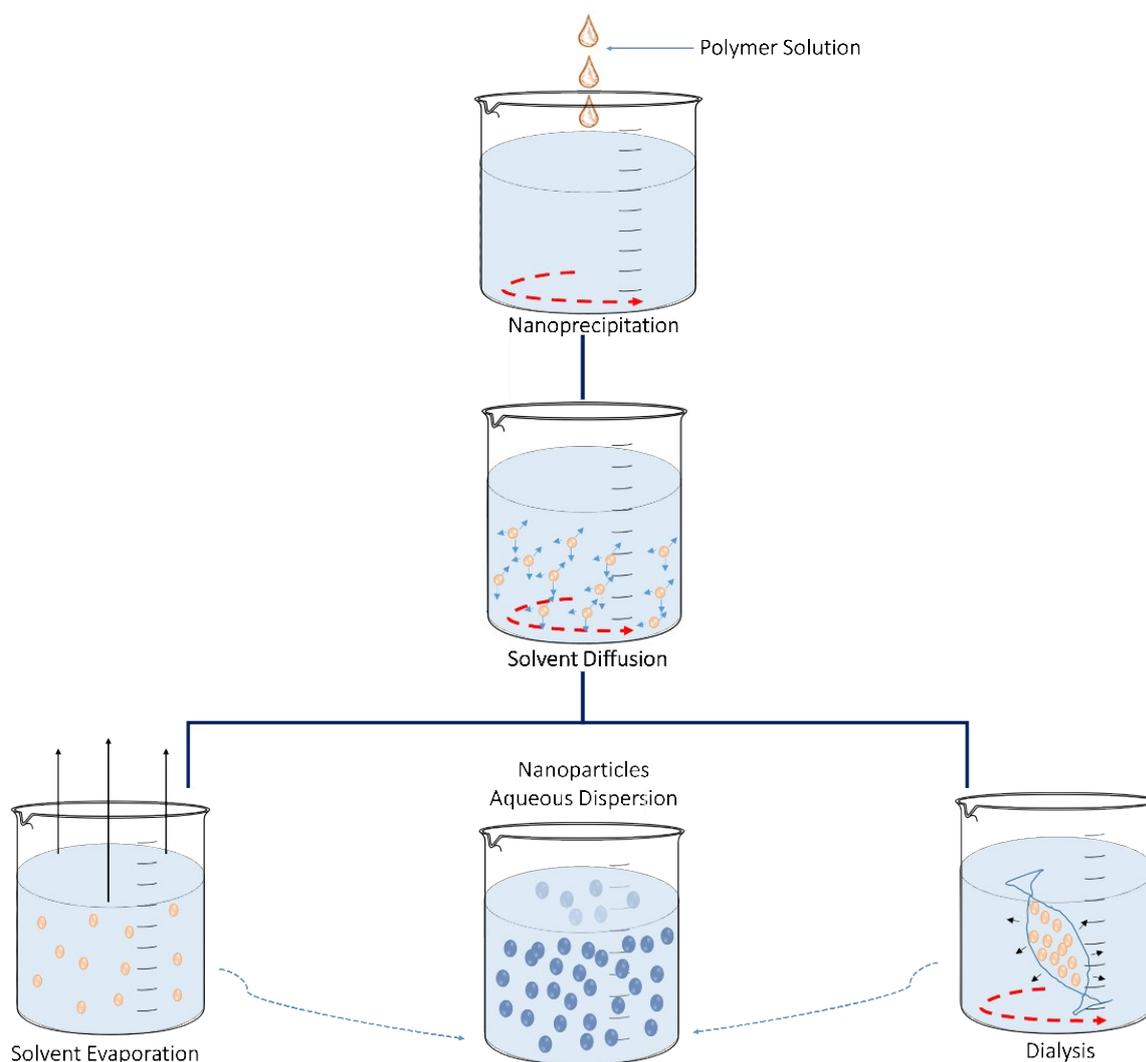
Figure S1. Illustration of the route to the generation of (nano)particles from poly(amino acid)-based macromolecules in solution, using the 'dropping-in' method.
