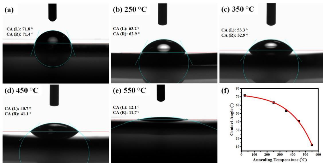
**Fig. S8** CA of DI water droplets on SiO<sub>2</sub>/Si substrate (a) before and after annealing in air for 10 min at (b) 250 °C, (c) 350 °C, (d) 450 °C, (e) 550 °C, respectively.
