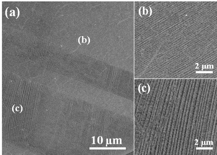
**Fig. S1** (a) SEM image of as-grown h-BN film on Cu. (b,c) Magnified SEM images in (a) showing the different orientation of the step bunches on different Cu grains.
