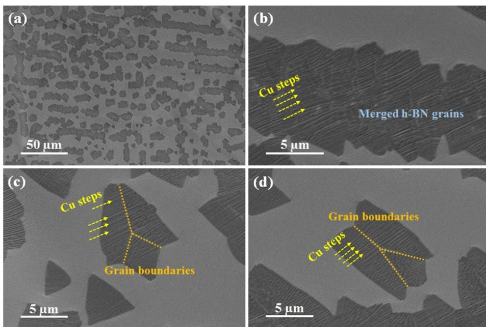
**Fig. S2** (a) SEM image of a partially continuous monolayer h-BN film. (b–d) Magnified SEM images revealing the Cu corrugation across multiple h-BN grain boundaries.
