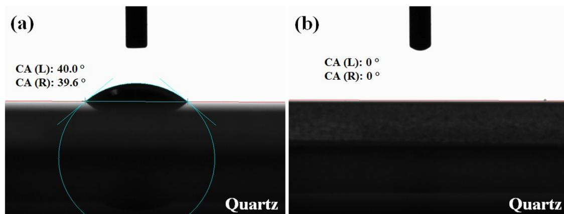
**Fig. S9** CA of DI water droplets on quartz substrates (a) before and (b) after annealing in air at 550 °C for 10min.
