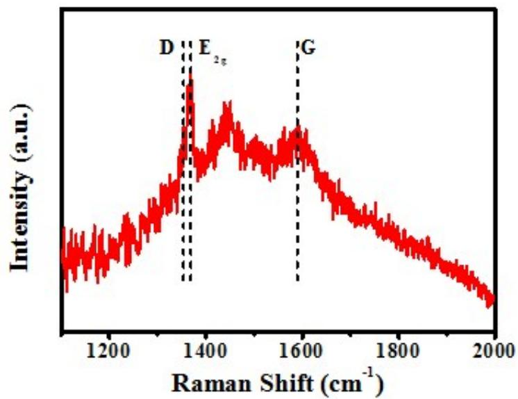
**Fig. S5** Representative Raman spectrum in some regions of the annealed h-BN film with multilayers indicating the presence of carbonaceous contamination by the presence of D and G bands.
