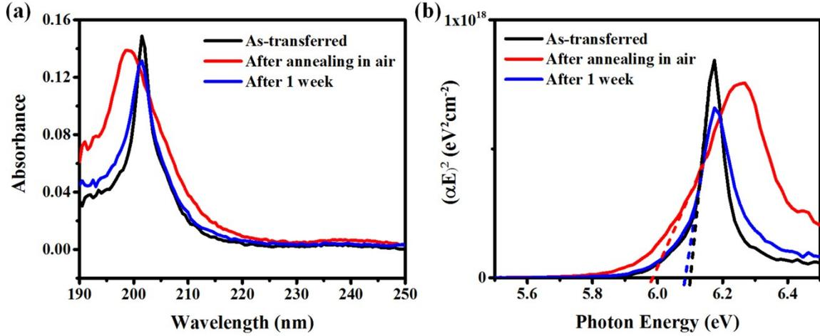
**Fig. S7** (a) UV-vis absorbance spectra and its corresponding (b) Tauc's plot of an as-transferred monolayer h-BN film (black trace), after annealing in air at 550 °C for 10 min (red trace) and after another week of inactivity (blue trace), on quartz substrate.
