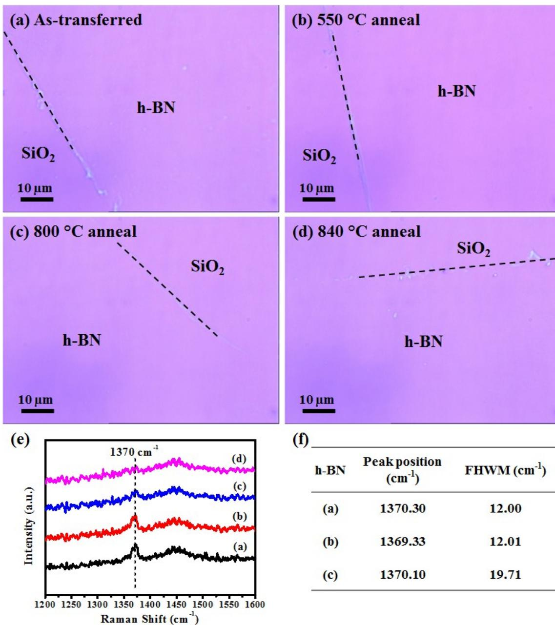
**Fig. S4** Optical images of (a) as-transferred h-BN film on SiO<sub>2</sub>/Si substrate and after annealing in air at (b) 550 °C, (c) 800 °C and (d) 840 °C. (e,f) Raman spectra and their corresponding fitted peaks of the respective h-BN films in (a – d).
