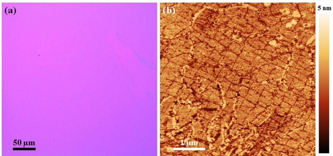
**Fig. S3** (a) Optical and (b) AFM images of transferred h-BN film after annealing at 840 °C for 2 h. The onset of oxidation can be observed by the presences of nanoscale pits and the elongated etch lines along the wrinkled structures.<sup>1</sup>
