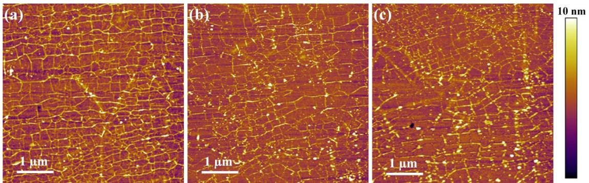
**Fig. S6** AFM images of (a) as-transferred h-BN film and after annealing at 550 °C under 200:20 sccm of Ar/H<sub>2</sub> for (b) 10 min and (c) 1 h. The h-BN wrinkles are still prevalent even after 1 h of annealing in Ar and H<sub>2</sub>.
