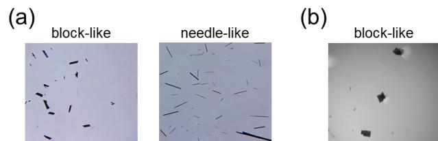
**Figure S3.** Photographs of single crystals of (a)  $[\text{Au}_{24}\text{Pd}(\text{PPh}_3)_{10}(\text{SC}_2\text{H}_4\text{Ph})_5\text{Cl}_2]\text{Cl}$  (block- and needle-like) and (b)  $[\text{Au}_{25}(\text{PPh}_3)_{10}(\text{SC}_2\text{H}_4\text{Ph})_5\text{Cl}_2][(\text{SbF}_6)_2]$  (block-like).
