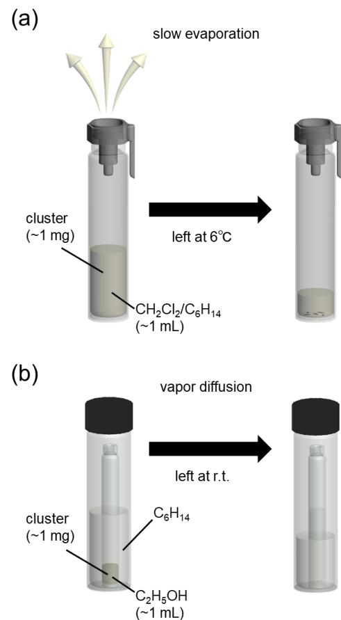
**Figure S2.** Schematic depiction of crystallization of (a)  $[\text{Au}_{24}\text{Pd}(\text{PPh}_3)_{10}(\text{SC}_2\text{H}_4\text{Ph})_5\text{Cl}_2]\text{Cl}$  (slow evaporation) and (b)  $[\text{Au}_{25}(\text{PPh}_3)_{10}(\text{SC}_2\text{H}_4\text{Ph})_5\text{Cl}_2][(\text{SbF}_6)_2]$  (vapor diffusion).
