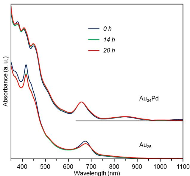
**Figure S11.** Time dependence of optical absorption spectra of chloroform solution of (a)  $[\text{Au}_{24}\text{Pd}(\text{PPh}_3)_{10}(\text{SC}_2\text{H}_4\text{Ph})_5\text{Cl}_2]\text{Cl}$  and (b)  $[\text{Au}_{25}(\text{PPh}_3)_{10}(\text{SC}_2\text{H}_4\text{Ph})_5\text{Cl}_2](\text{SbF}_6)_2$ .
