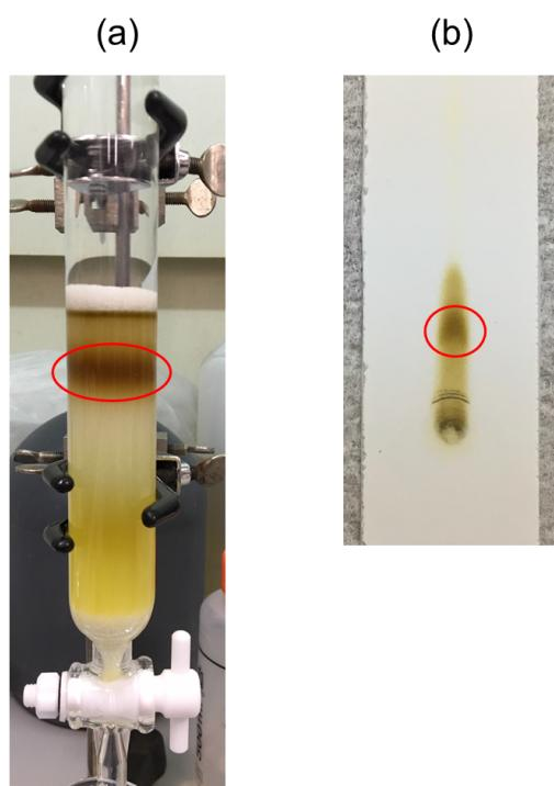
**Figure S1.** Purification of  $[\text{Au}_{24}\text{Pd}(\text{PPh}_3)_{10}(\text{SC}_2\text{H}_4\text{Ph})_5\text{Cl}_2]\text{Cl}$  by (a) silica-gel column chromatography and (b) thin-layer chromatography to obtain high-purity samples. Red circles indicate  $[\text{Au}_{24}\text{Pd}(\text{PPh}_3)_{10}(\text{SC}_2\text{H}_4\text{Ph})_5\text{Cl}_2]\text{Cl}$ .
