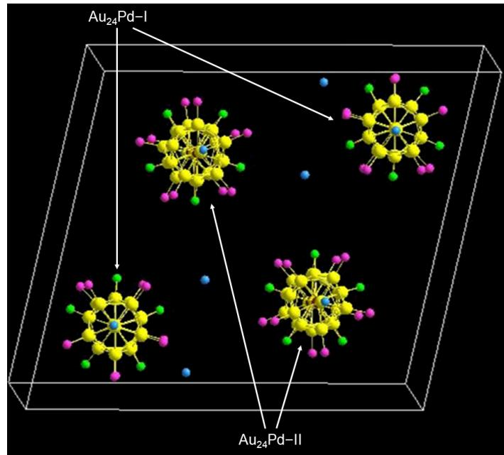
**Figure S6.** Unit cell of the crystal of  $[\text{Au}_{24}\text{Pd}(\text{PPh}_3)_{10}(\text{SC}_2\text{H}_4\text{Ph})_5\text{Cl}_2]\text{Cl}$ .
