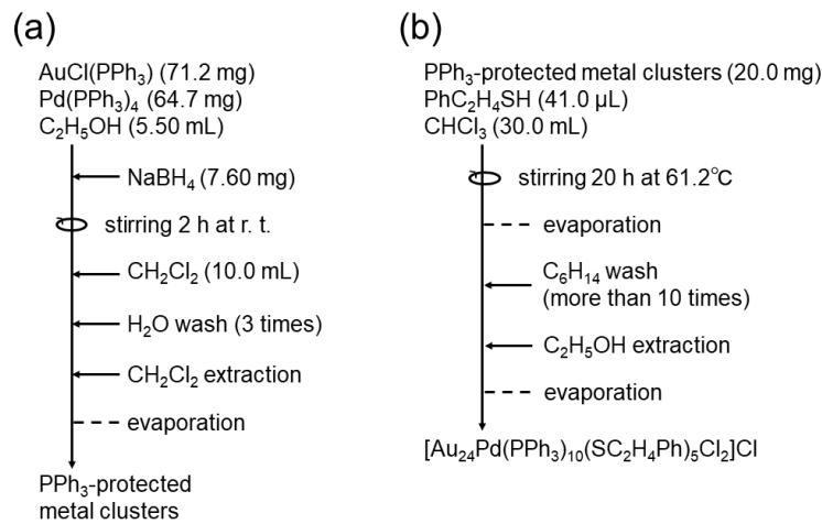
**Scheme S1.** Protocol for isolating high-purity  $[\text{Au}_{24}\text{Pd}(\text{PPh}_3)_{10}(\text{SC}_2\text{H}_4\text{Ph})_5\text{Cl}_2]\text{Cl}$ .
