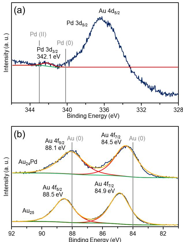
**Figure S13.** (a) Pd 3d<sub>3/2</sub> spectrum and (b) Au 4f spectrum of  $[\text{Au}_{24}\text{Pd}(\text{PPh}_3)_{10}(\text{SC}_2\text{H}_4\text{Ph})_5\text{Cl}_2]\text{Cl}$ . In (b), Au 4f spectra of  $[\text{Au}_{25}(\text{PPh}_3)_{10}(\text{SC}_2\text{H}_4\text{Ph})_5\text{Cl}_2][(\text{SbF}_6)_2]$  is also shown for comparison.
