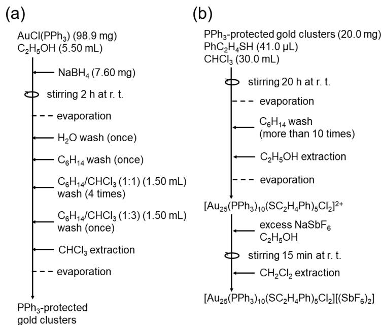
**Scheme S2.** Protocol for isolating high-purity  $[\text{Au}_{25}(\text{PPh}_3)_{10}(\text{SC}_2\text{H}_4\text{Ph})_5\text{Cl}_2][(\text{SbF}_6)_2]$ .<sup>1</sup>
