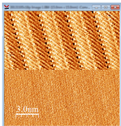
Figure S4.2. Half-half image. STM current image of C18p at the TCB/HOPG interface. The bias voltage was changed during scanning, revealing atomic resolution of the HOPG. 15 \text{ nm} \times 15 \text{ nm} ; I_t = 18 \text{ pA} . V_b = -350 \text{ mV} (SAM). I_t = 18 \text{ pA} , V_b = 40 \text{ mV} (HOPG).
