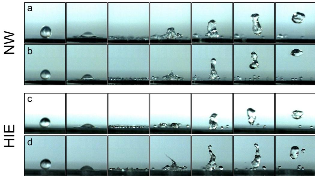
**Fig. S3** Snapshots of the impact dynamics on NWs surface with (a) 0 %, pure water droplet and (b) 1 % ethanol in water mixture liquid droplet. Impact dynamics on HIE surface also captured with (c) 0 %, pure water droplet and (d) 1 % ethanol in water mixture liquid droplet. The dropping height is fixed at 30 cm, and the frame rate is 5000 fps.
