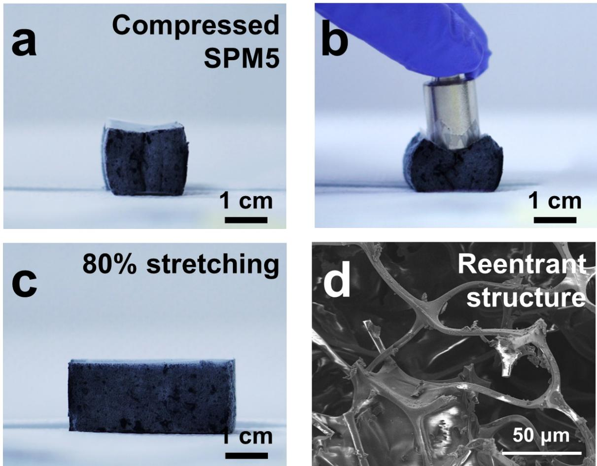
**Figure S4.** Digital image of SPM5 with lateral compression. (a) Laterally compressed SPM5. (b) Deformed SPM5 under vertical pressure. (c) Stretched SPM5 (d) SEM image of compressed SPM5.
