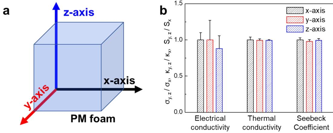
**Figure S3.** (a) Schematic image of PM foam with measurement direction, (b) relative electrical conductivity, thermal conductivity and Seebeck coefficient against to horizontal direction (x-axis).
