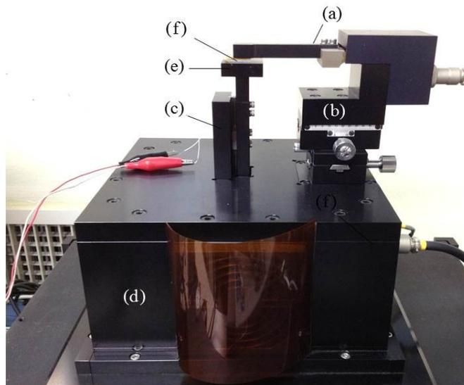
**Figure S9.** Fatigue test setup with moving coil linear stage to evaluate the durability of the sensor: (a) cantilever type load-cell, (b) positioning stage, (c) linear-guide, (d) actuator part composed of field magnet and moving bobbin with coil, (e) jig and flat plate, and (f) distributed force sensor.
