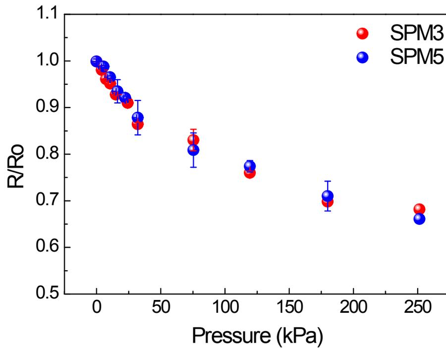
**Figure S6.** Change in the electrical resistance of 95%-compressed SPM foams with different thickness of PEDOT:PSS layer (SPM3 and SPM5) as a function of applied pressure.
