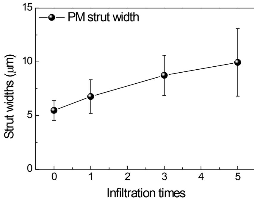
**Figure S1.** The strut widths as a function of PEDOT:PSS infiltration times. The strut widths increase linearly with infiltration numbers.
