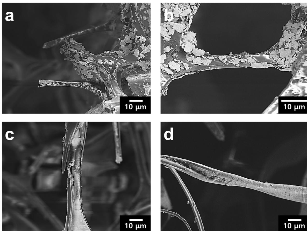
**Figure S2.** SEM image of PM (a, b) and SPM (c, d) after repeated pressure loading and unloading test. In PM, delaminated powdery PEDOT:PSS from the MF skeleton is observed (a, b). On the other hand, in SPM, PEDOT:PSS powder is not observed hence the particle is stuck to SEBS sheath. Moreover, SEBS mechanically enhances of the SPM by holding the structure after pressure (c).
