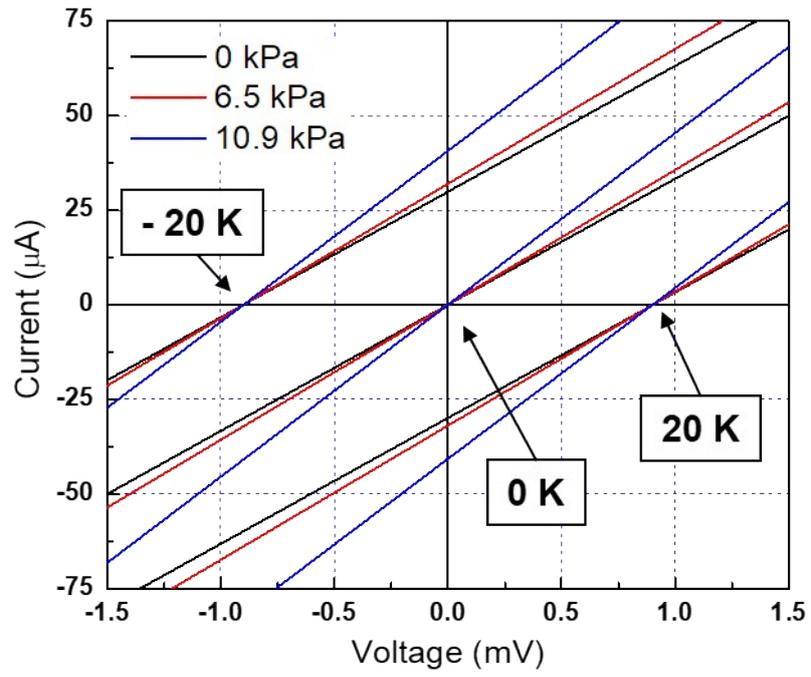
**Figure S8.** I-V curves of the SPM-based TEG as a function of temperature difference and pressure. The  $T_0$  is 0 K.
