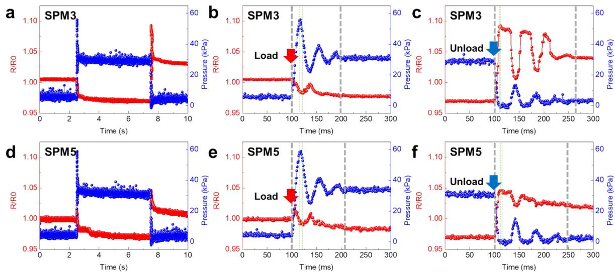
**Figure S7.** Pressure-sensing performance of 95%-compressed SPM3 and SPM5 foams. The resistnace difference versus time for (a-c) SPM3 and (d-f) SPM5 with 35 kPa for the observation of response and recovery behaviors.
